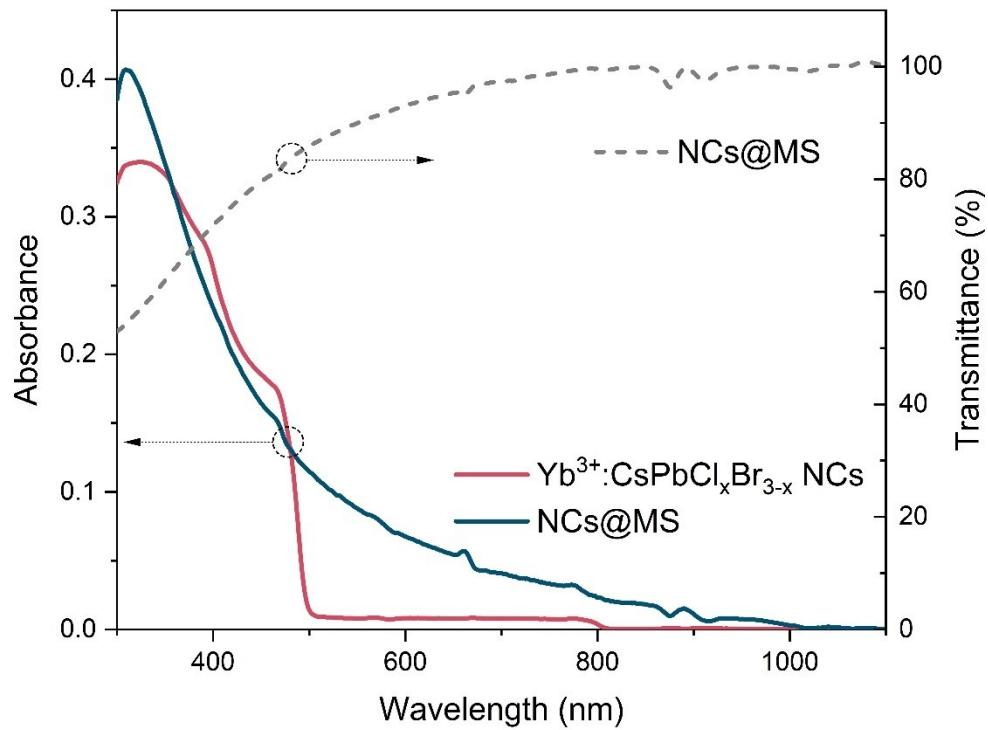
Fig. S13. Absorption spectra (solid lines) of Yb<sup>3+</sup>:CsPbCl<sub>3</sub> NCs and those NCs embedded into MS (NCs@MS), and transmittance spectrum (dashed line) of the latter.
