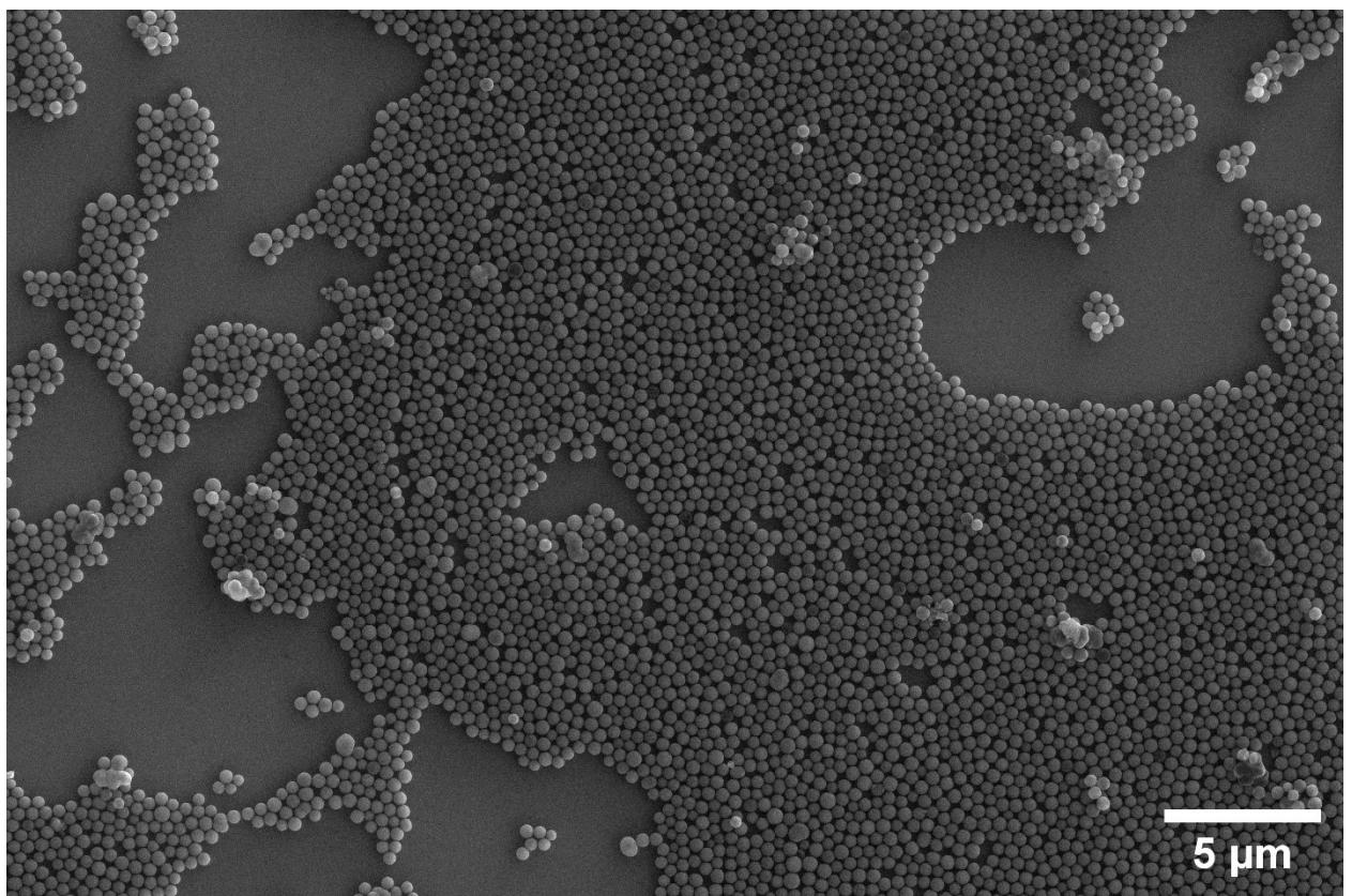
Fig. S12. Large-area SEM image of MS with embedded  $\text{Yb}^{3+}:\text{CsPbCl}_3$  NCs, spread over Si substrate.
