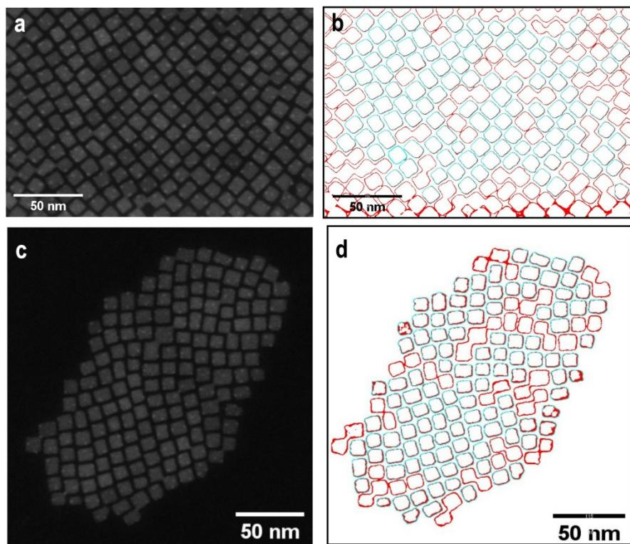
Fig. S2. HAADF-STEM images (a, c) of  $\text{Yb}^{3+}:\text{CsPbCl}_3$  NCs and (b, d) estimation of their area using ImageJ software. The blue counter indicates counted NCs, while the red counter indicates non-counted (merged or border-sharing) NCs. An average edge length was calculated as a root square of the average counted area.
