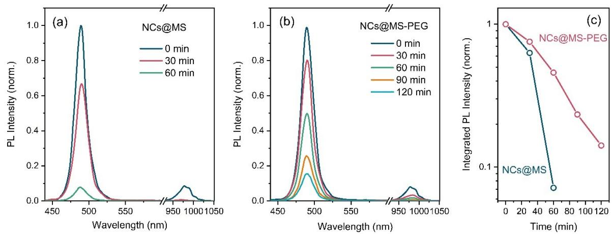
Fig. S17. Stability of PL response in water for NCs@MS without and with PEG functionalization. PL spectra taken for NCs@ MS without (a) and with (b) PEG functionalization after the specified periods of time. (c) The dependencies of integrated PL intensities over time in water for NCs@MS without (blue) and with (red) PEG functionalization.
