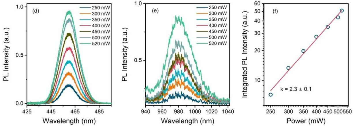
Fig. S19. PL spectra in the visible (a, d) and NIR (b, e) spectral regions taken from NCs@MS covered with PEG and dispersed in toluene (upper panel) and water (bottom panel) under TPA-excitation. (c, f) Corresponding dependencies of the integrated PL intensity upon the excitation power; the slopes confirm occurrence of the TPA excitation.
