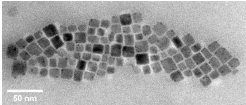
Fig. S1. TEM image of  $\text{Yb}^{3+}:\text{CsPbCl}_3$  NCs.
