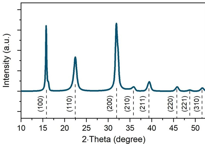
Fig. S3. XRD pattern of the synthesized Yb<sup>3+</sup>:CsPbCl<sub>3</sub> NCs compared to the reference (vertical dashed lines) CsPbCl<sub>3</sub> cubic perovskite phase (PDF Card No. 01-075-0411).
