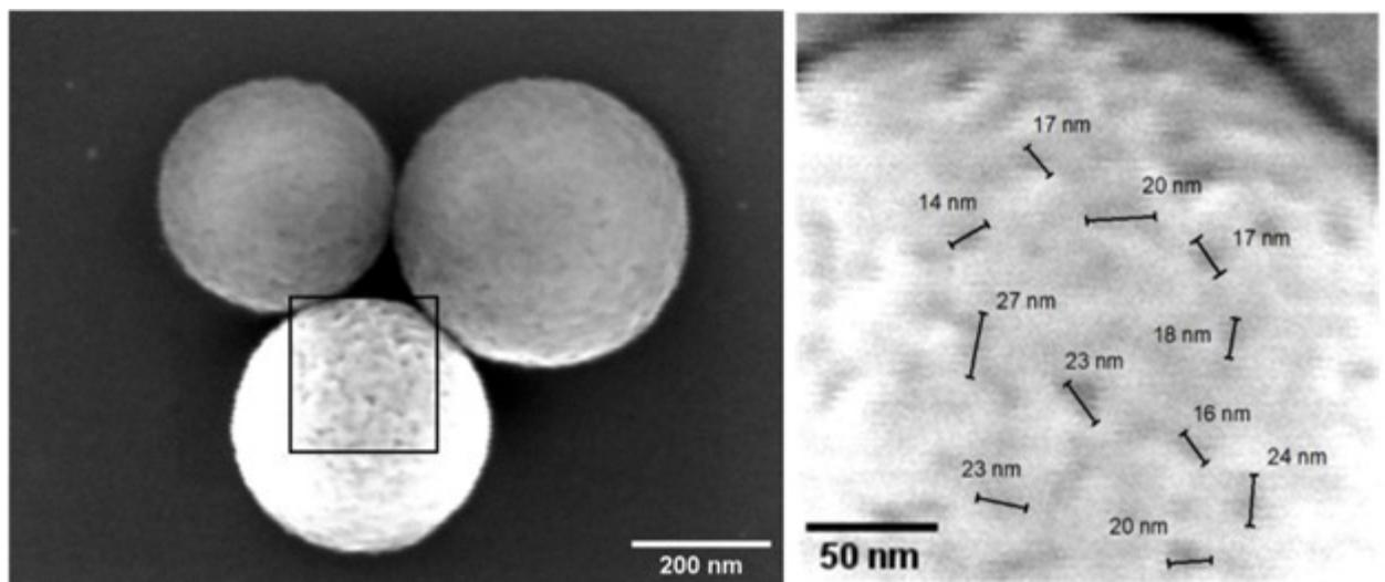
Fig. S11. Estimation of MS pores size from their SEM images.
