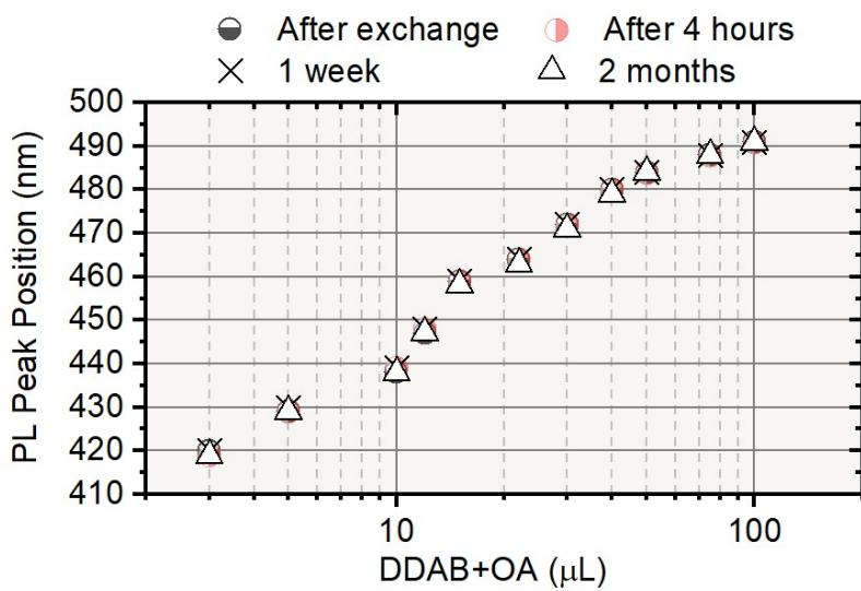
Fig. S6. Stability of the band-edge PL peak positions for the Yb<sup>3+</sup>:CsPbCl<sub>x</sub>Br<sub>3-x</sub> NCs after an anion exchange.
