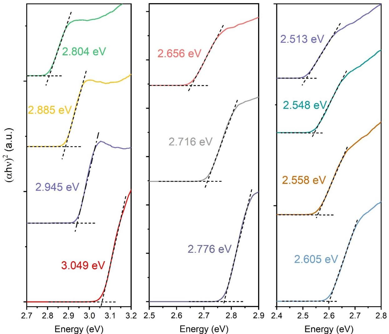
Fig. S8. Tauc plots for the  $\text{Yb}^{3+}:\text{CsPbCl}_x\text{Br}_{3-x}$  NCs shown in Fig. S6. The bandgaps were calculated as an intercept of the slope's linear fit with a zero line.
