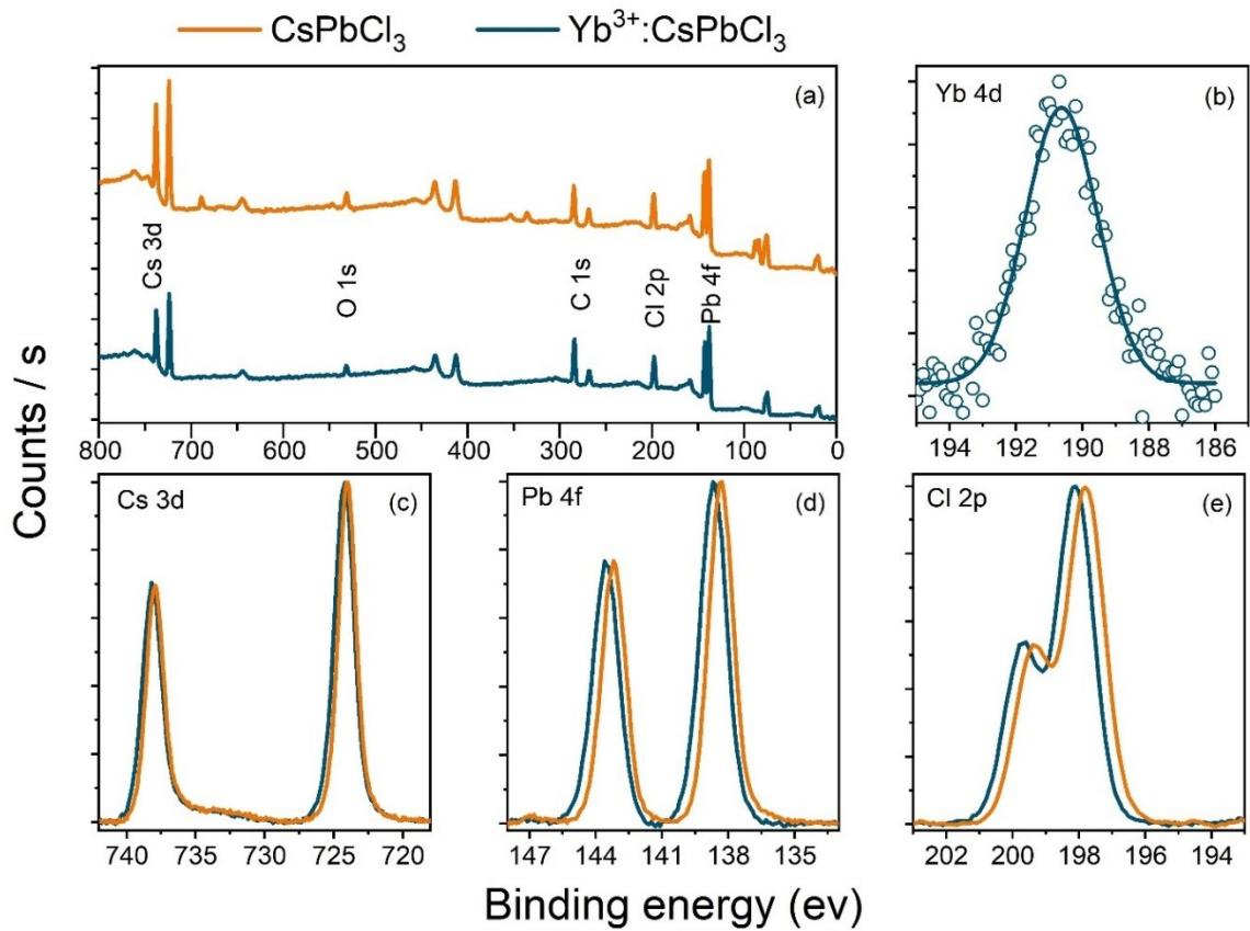
Fig. S5. (a) Survey XPS spectra for the undoped CsPbCl<sub>3</sub> (orange line) and doped Yb<sup>3+</sup>:CsPbCl<sub>3</sub> (blue line) NCs. (b) High-resolution XPS spectra of the Yb 4d peak for the doped Yb<sup>3+</sup>:CsPbCl<sub>3</sub> NCs. High-resolution XPS spectra for Cs 3d (c), Pb 4f (d), and Cl 2p (e) peaks for the undoped CsPbCl<sub>3</sub> (orange lines) and doped Yb<sup>3+</sup>:CsPbCl<sub>3</sub> (blue lines) NCs.
