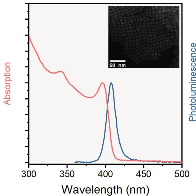
Fig. S4. Absorption and PL spectra of the undoped CsPbCl<sub>3</sub> NCs. The inset shows their HAADF-STEM image.
