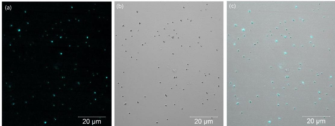
Fig. S18. Large-area luminescence (a), transmitted light (b), and superimposed (c) images of the NCs@MS covered with PEG obtained by CLSM.
