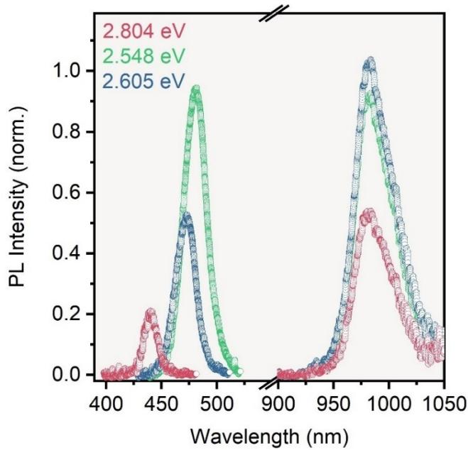
Fig. S9. PL spectra of the  $\text{Yb}^{3+}:\text{CsPbCl}_x\text{Br}_{3-x}$  NCs with different bandgaps (marked with numbers on the frame) taken under two-photon (800 nm) excitation and corrected to the spectral sensitivity of the detection system.
