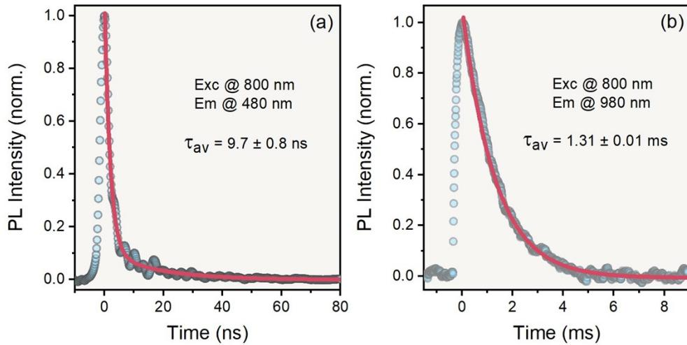
Fig. S10. PL decay kinetics recorded under 800 nm excitation for the band-edge related (a) and  $\text{Yb}^{3+}$ -related (b) emissions for  $\text{Yb}^{3+}:\text{CsPbCl}_3$  NCs. Solid lines are two- (a) and one-exponential (b) fits, respectively.
