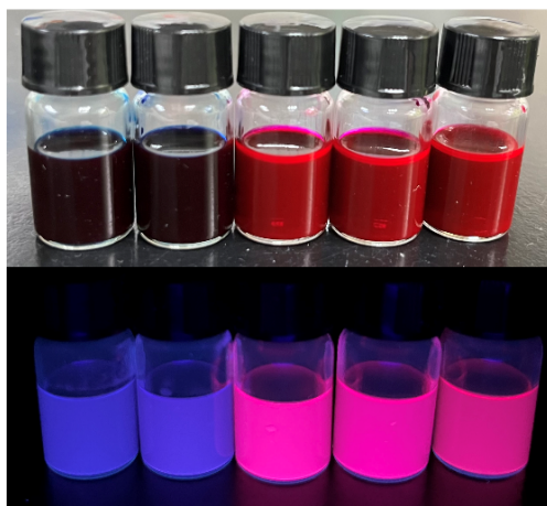
Figure S2. The images are photographs of reaction mixtures prepared at different reaction temperatures with ATA and NBA as co-reactants under daylight (top) and 365 nm UV light (bottom). From left to right, these samples were prepared at 120, 140, 160, 180 and 200 °C, respectively.
