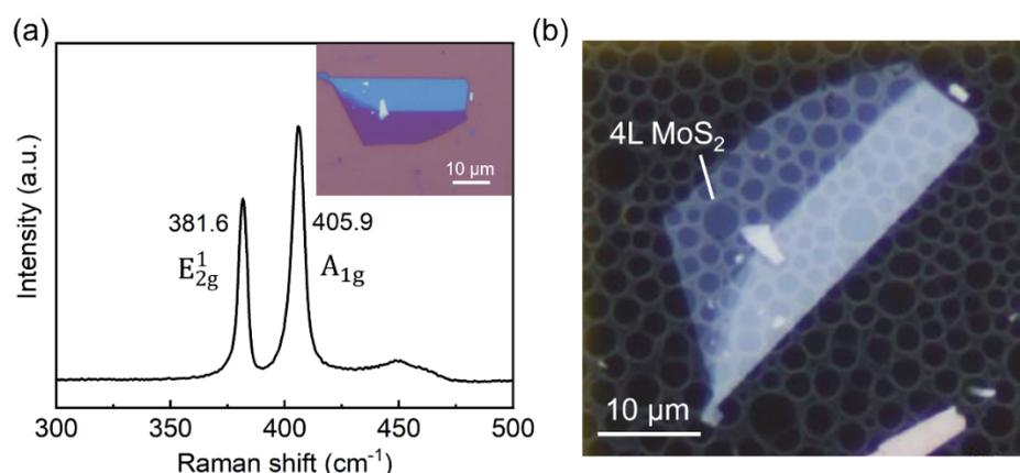
**Figure S1.** (a) Raman spectrum of the thinner layer of MoS<sub>2</sub>. Inset: Optical image of a MoS<sub>2</sub> flake on SiO<sub>2</sub>/Si substrate. Raman spectrum was captured from the thinner layer (purple color). (b) Optical image of the MoS<sub>2</sub> flake transferred on gold microgrid coated with a holey carbon film.
