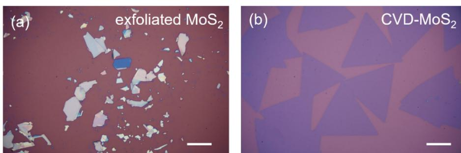
**Figure S5.** Optical images of mechanically exfoliated MoS<sub>2</sub> flakes (a) and monolayer MoS<sub>2</sub> domains grown by chemical vapor deposition (CVD) (b) on SiO<sub>2</sub>/Si substrate. The scale bars are all 20 μm.
