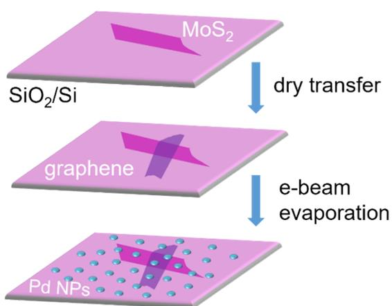
**Figure S7.** Schematic diagram of the preparation process of Pd NPs/graphene/MoS<sub>2</sub> heterostructure.
