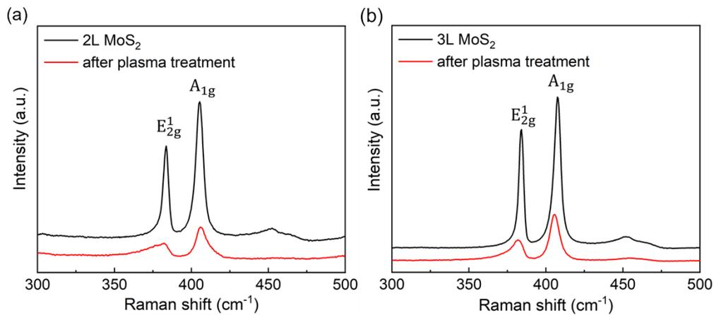
**Figure S4.** Raman spectra of 2L (a) and 3L (b) MoS<sub>2</sub> before and after air plasma treatment.
