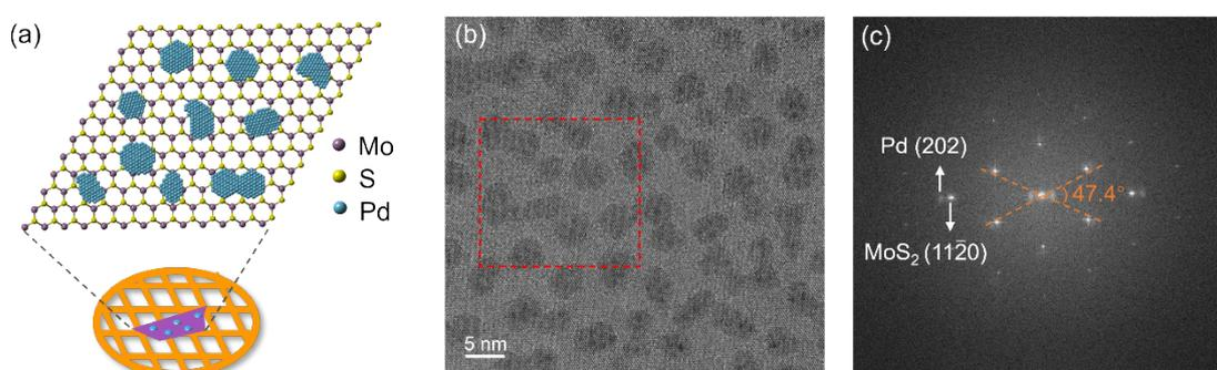
**Figure S2.** (a) The schematic of Pd NPs/MoS<sub>2</sub> heterostructure on a gold TEM microgrid. (b) HRTEM image of Pd NPs/MoS<sub>2</sub> heterostructure with moiré fringes. (c) Fast Fourier transform (FFT) pattern obtained from the region marked by the red dashed frame in (b). The expansion of the diffraction spots near the central spot reflects the distribution of the rotation angles. The included angle between the two orange dashed lines is measured to be  $47.4^\circ$ .
