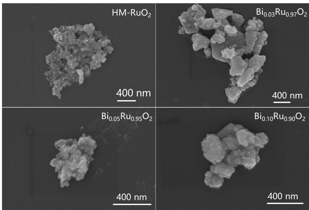
Figure S8 SEM images of HM-RuO<sub>2</sub>, Bi<sub>0.03</sub>Ru<sub>0.97</sub>O<sub>2</sub>, Bi<sub>0.05</sub>Ru<sub>0.95</sub>O<sub>2</sub>, Bi<sub>0.10</sub>Ru<sub>0.90</sub>O<sub>2</sub>.
