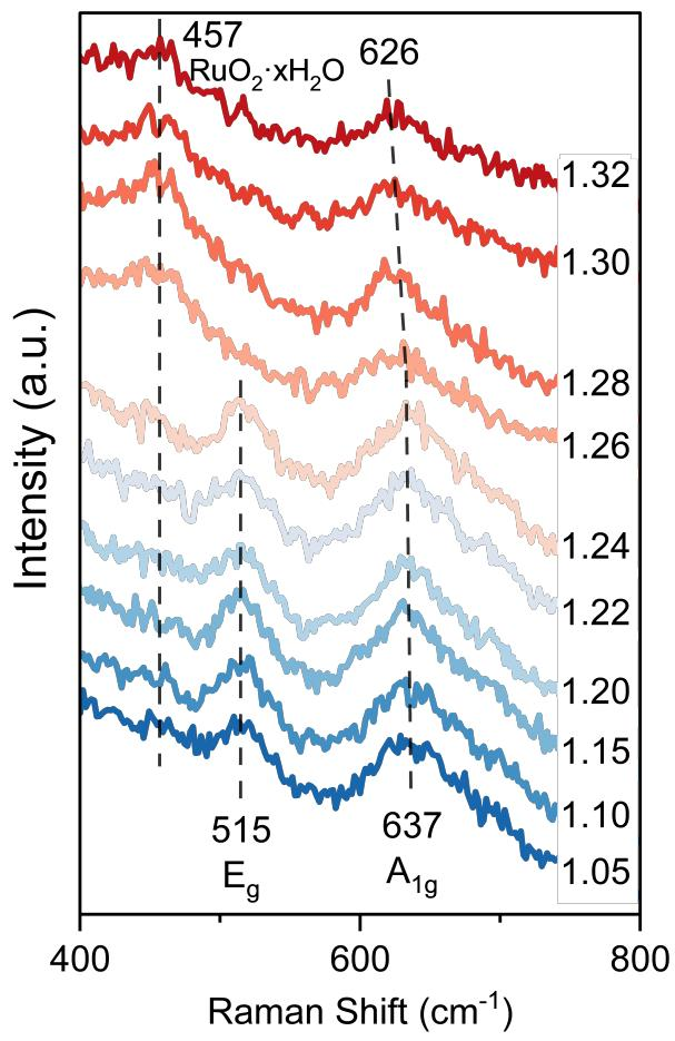
Figure S22. In-situ Raman spectra collected form  $\text{Bi}_{0.05}\text{Ru}_{0.95}\text{O}_2$  catalyst in  $0.1 \text{ M HClO}_4$ .
