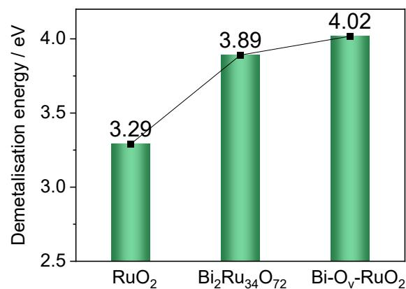
Figure S29 The demetalisation energies of  $\text{RuO}_2$ ,  $\text{Bi}_2\text{Ru}_{34}\text{O}_{72}$  and  $\text{Bi}-\text{O}_v-\text{RuO}_2$ .
