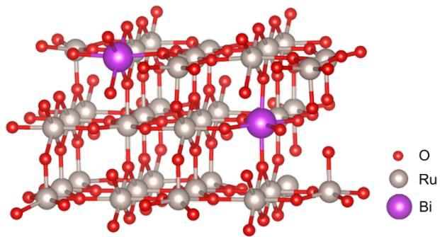
Figure S1 Slab model of  $\text{Bi}_2\text{Ru}_{34}\text{O}_{72}$  after structural optimization.
