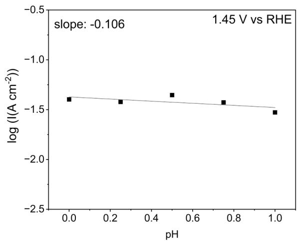
Figure S28 Log (I (A cm<sup>-2</sup>)) of  $\text{Bi}_{0.05}\text{Ru}_{0.95}\text{O}_2$  electrode at 1.45 V vs. RHE as a function of pH.
