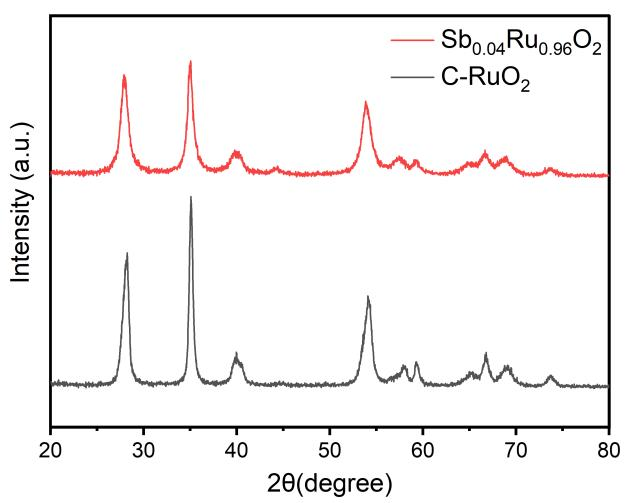
Figure S23 XRD patterns of  $\text{Sb}_{0.04}\text{Ru}_{0.96}\text{O}_2$  and C-RuO<sub>2</sub>.
