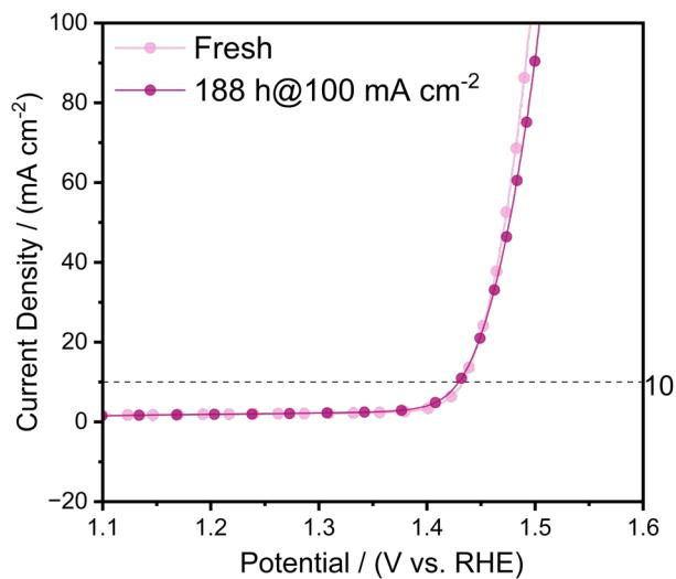
Figure S20 Polarization curves at the scan rate of  $5\text{ mV s}^{-1}$  for  $\text{Bi}_{0.05}\text{Ru}_{0.95}\text{O}_2$  electrode in 0.5 M  $\text{H}_2\text{SO}_4$  electrolyte before and after 188-h stability test at  $100\text{mA cm}^{-2}$ .
