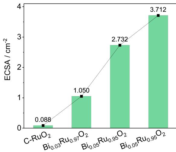
Figure S12 Comparison of electrochemical active surface areas of  $\text{Bi}_x\text{Ru}_{1-x}\text{O}_2$  and C-RuO<sub>2</sub>.
