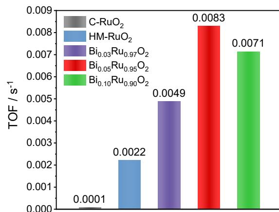
Figure S17 Turnover frequency comparison of  $\text{Bi}_x\text{Ru}_{1-x}\text{O}_2$ , HM-RuO<sub>2</sub> and C-RuO<sub>2</sub>.
