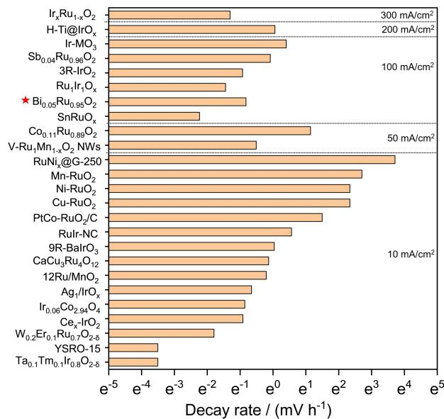
Figure S21 Comparison of decay rate (mV h<sup>-1</sup>) between Bi<sub>0.05</sub>Ru<sub>0.95</sub>O<sub>2</sub>, Sb<sub>0.04</sub>Ru<sub>0.96</sub>O<sub>2</sub> and recently-reported Ru- and Ir-based catalysts at their reported current density.
