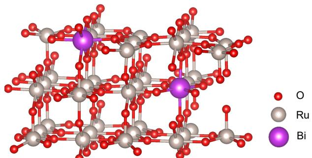
Figure S3 Slab model of  $\text{Bi}-\text{O}_v-\text{RuO}_2$  after structural optimization.
