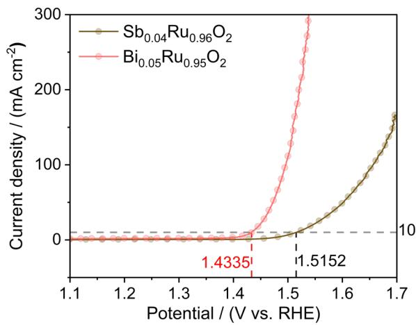
Figure S26 Polarization curves at the scan rate of 5 mV s<sup>-1</sup> for Sb<sub>0.04</sub>Ru<sub>0.96</sub>O<sub>2</sub> and Bi<sub>0.05</sub>Ru<sub>0.95</sub>O<sub>2</sub> electrodes in 0.5 M H<sub>2</sub>SO<sub>4</sub> electrolyte.
