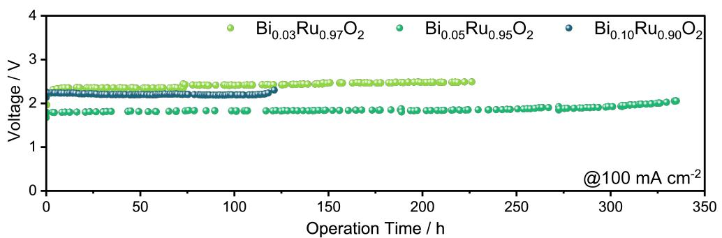
Figure S15 Chronopotentiometry tests of  $\text{Bi}_x\text{Ru}_{1-x}\text{O}_2$  at  $100 \text{ mA cm}^{-2}$  in  $0.5 \text{ M H}_2\text{SO}_4$  electrolyte.
