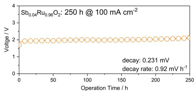
Figure S27 Stability test of Sb<sub>0.04</sub>Ru<sub>0.96</sub>O<sub>2</sub> electrode at the current density of 100 mA cm<sup>-2</sup> in 0.5 M H<sub>2</sub>SO<sub>4</sub>.
