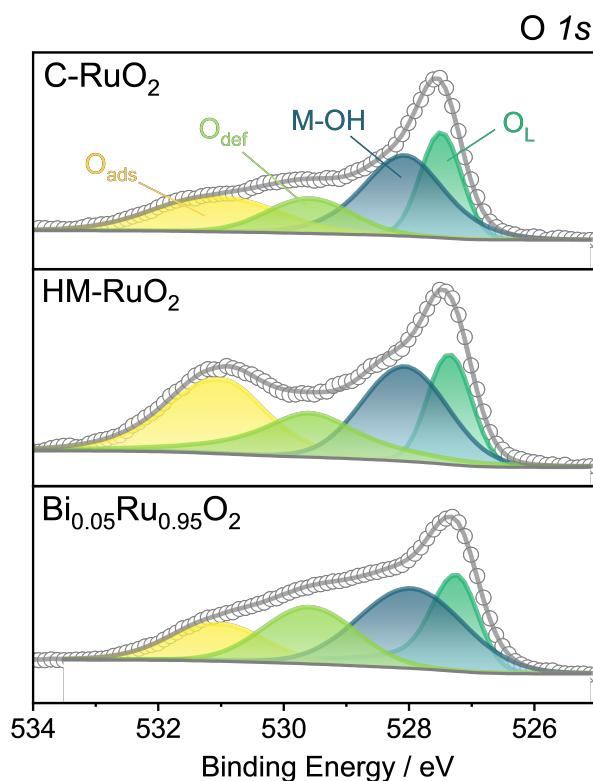
Figure S10 O 1s XPS spectra of  $\text{Bi}_{0.05}\text{Ru}_{0.95}\text{O}_2$ , HM-RuO<sub>2</sub> and C-RuO<sub>2</sub>. More details are shown in Table S2.
