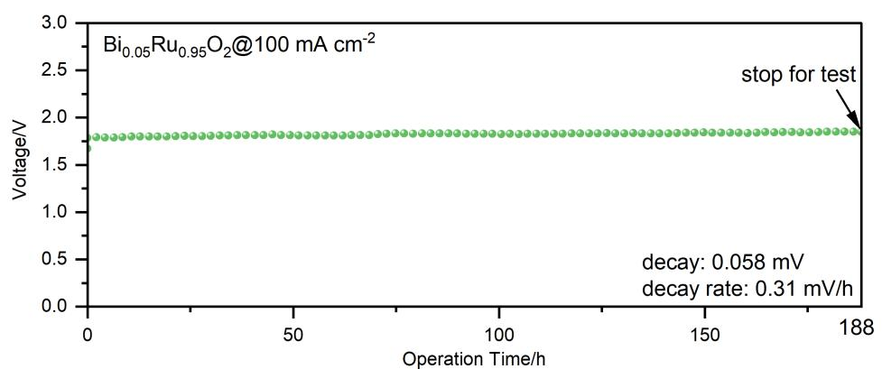
Figure S18 Chronopotentiometry test of  $\text{Bi}_{0.05}\text{Ru}_{0.95}\text{O}_2$  in 0.5 M  $\text{H}_2\text{SO}_4$  electrolyte at 100  $\text{mA cm}^{-2}$  for 188 h. The electrode after the stability test was used for subsequent tests.
