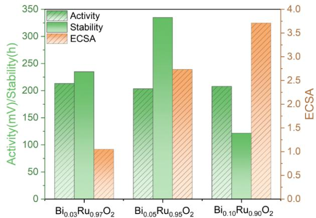
Figure S16 Comparison of activity (overpotential@10 mA cm<sup>-2</sup>) and stability (at 100 mA cm<sup>-2</sup>) among various  $\text{Bi}_x\text{Ru}_{1-x}\text{O}_2$ .
