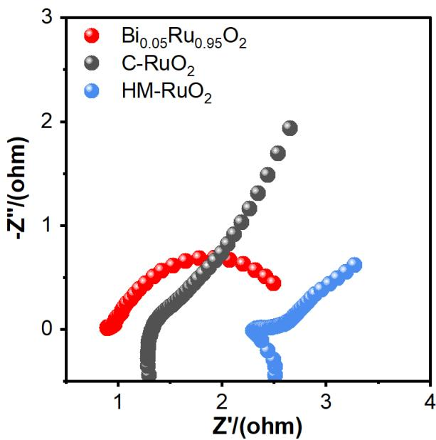
Figure S14 EIS plot of  $\text{Bi}_{0.05}\text{Ru}_{0.95}\text{O}_2$ , HM-RuO<sub>2</sub> and C-RuO<sub>2</sub> at a voltage (init E) of 1.24 V in 0.5 M H<sub>2</sub>SO<sub>4</sub> electrolyte. The frequency range for testing is from 100 kHz to 1 Hz.
