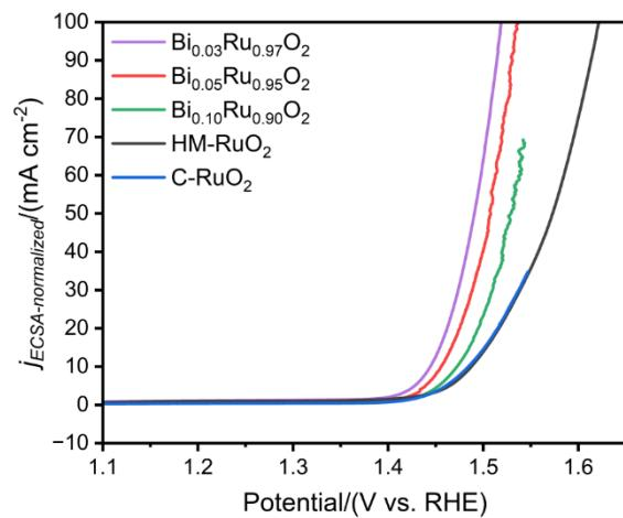
Figure S13 Specific activity curves of  $\text{Bi}_x\text{Ru}_{1-x}\text{O}_2$ , HM-RuO<sub>2</sub> and C-RuO<sub>2</sub> electrode collected at the scan rate of 5 mV s<sup>-1</sup> in 0.5 M H<sub>2</sub>SO<sub>4</sub> electrolyte.
