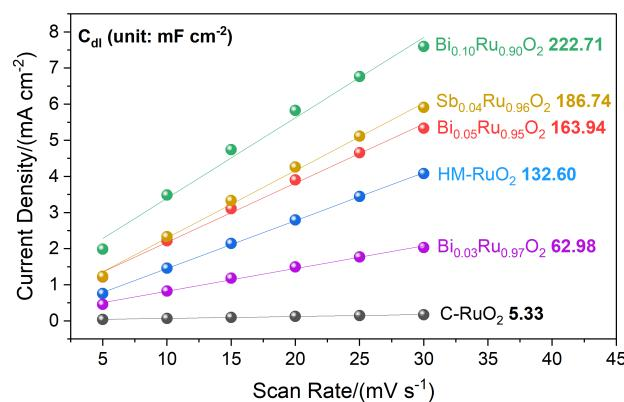
Figure S11  $C_{dl}$  linear fitting plot of  $\text{Bi}_x\text{Ru}_{1-x}\text{O}_2$ ,  $\text{Sb}_{0.04}\text{Ru}_{0.96}\text{O}_2$ , HM-RuO<sub>2</sub> and C-RuO<sub>2</sub> derived from CV curves.
