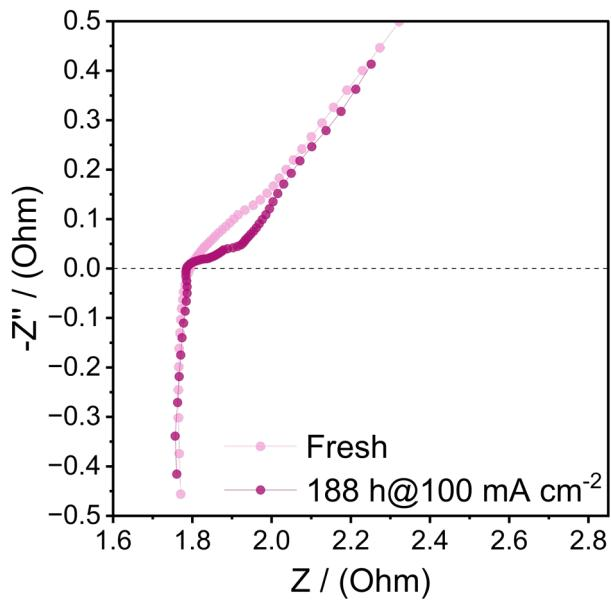
Figure S19 EIS plots of  $\text{Bi}_{0.05}\text{Ru}_{0.95}\text{O}_2$  at a voltage (init E) of 1.24 V in 0.5 M  $\text{H}_2\text{SO}_4$  electrolyte before and after 188-h stability test at  $100\text{mA cm}^{-2}$ . The frequency range for testing is from 100 kHz to 1 Hz.
