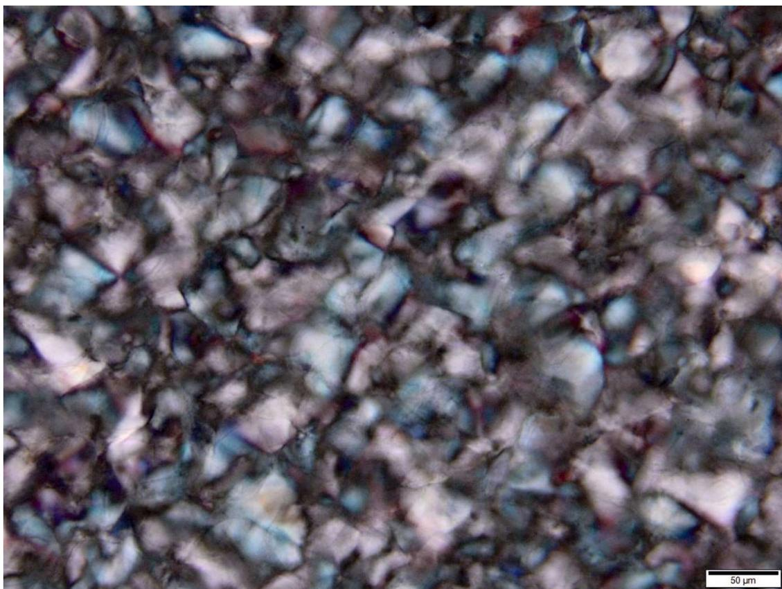
**Figure S17.** Polarized optical microscopy (POM) image of CNMO film prepared from organosilica precursor and CNC suspension (**Et-CNMO-1**). Image was captured between crossed polarizers using a 20x objective lens in transmittance mode. Scale bar is 50  $\mu\text{m}$ . Original image included in **Figure 4c** in the manuscript.
