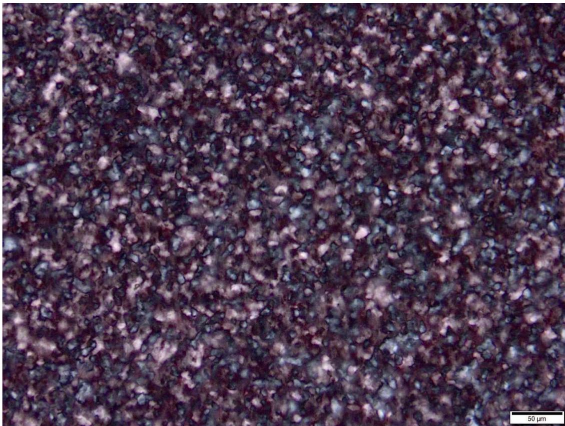
**Figure S18.** Polarized optical microscopy (POM) image of CNMO film prepared from organosilica precursor, CNC suspension and sucrose (**Et-CNMO-3e**). Image was captured between crossed polarizers using a 20x objective lens in transmittance mode. Scale bar is 50  $\mu\text{m}$ . Original image included in **Figure 4d** in the manuscript.
