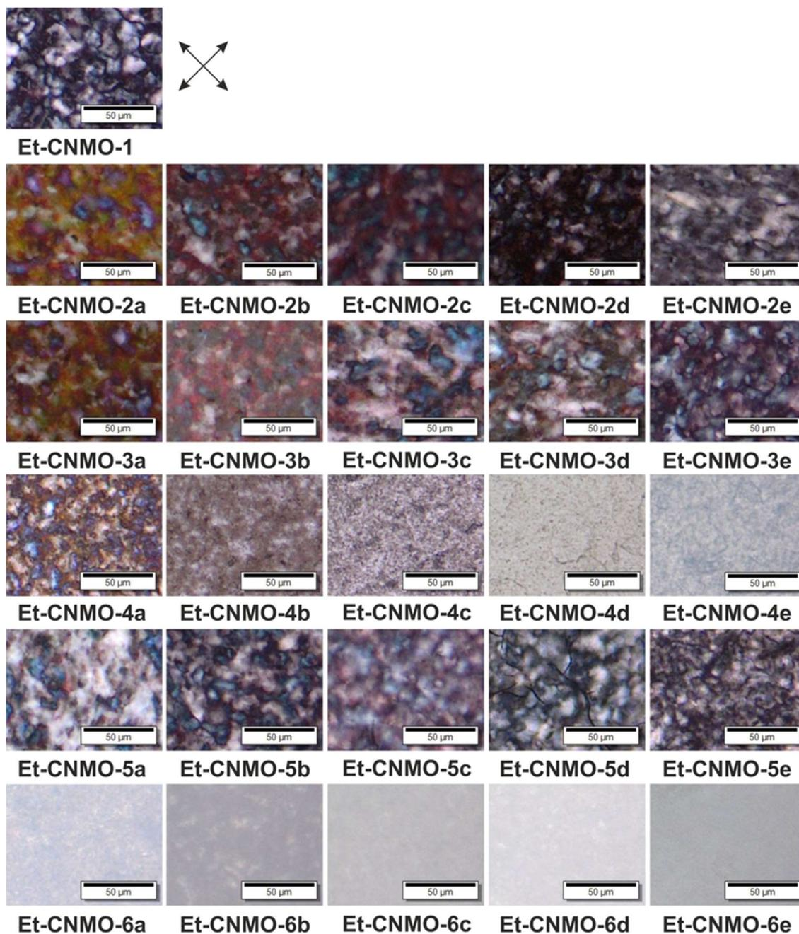
**Figure S14.** Polarized optical microscopy (POM) images of all CNMO films. Images were captured between crossed polarizers using a 20x objective lens in transmittance mode. Scale bars are 50  $\mu\text{m}$ .
