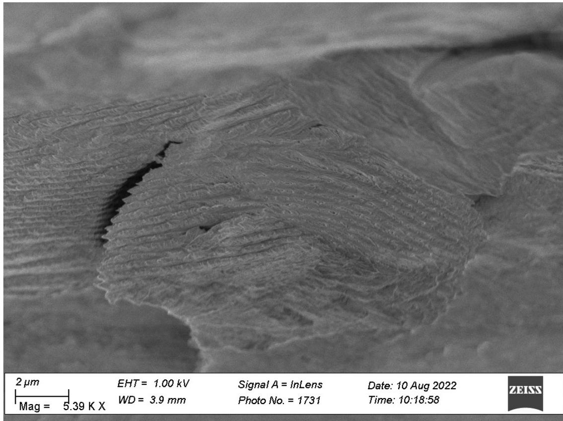
**Figure S19.** SEM image (cross section) of composites prepared from organosilica precursor and CNC suspension (C-1) – original image included in **Figure 5a** in the manuscript.
