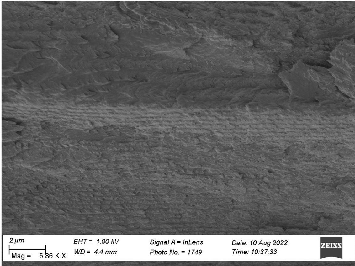
**Figure S21.** SEM image (cross section) of composites prepared from organosilica precursor and CNC suspension (**Et-CNMO-1**) – original image included in **Figure 5c** in the manuscript.
