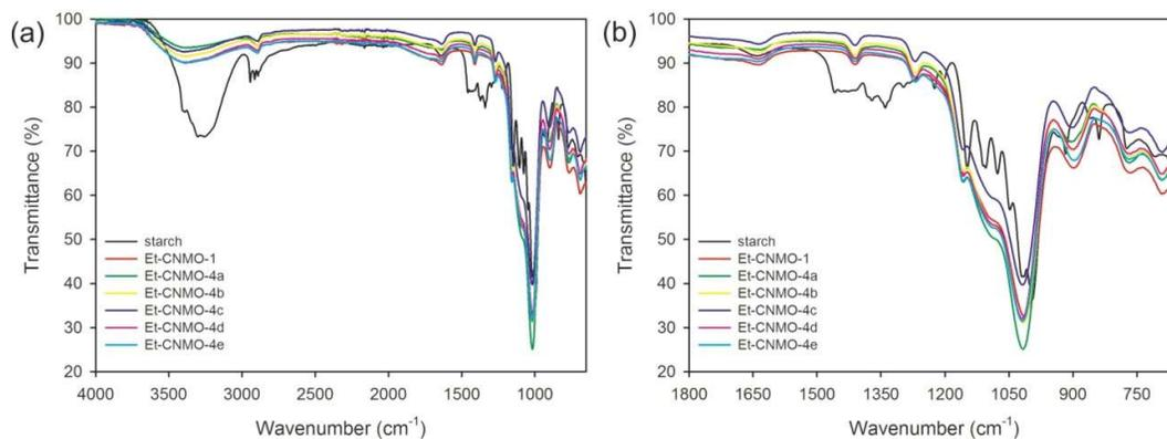
**Figure S5.** IR spectra measured for starch, **Et-CNMO-1** and **Et-CNMO-4**; (a) full spectral range, (b) zoomed range.
