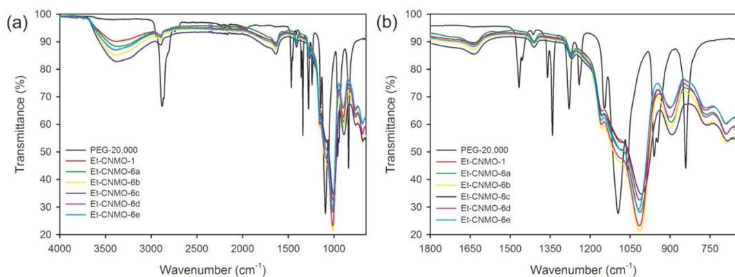
**Figure S7.** IR spectra measured for PEG-20,000, **Et-CNMO-1** and **Et-CNMO-6**; (a) full spectral range, (b) zoomed range.
