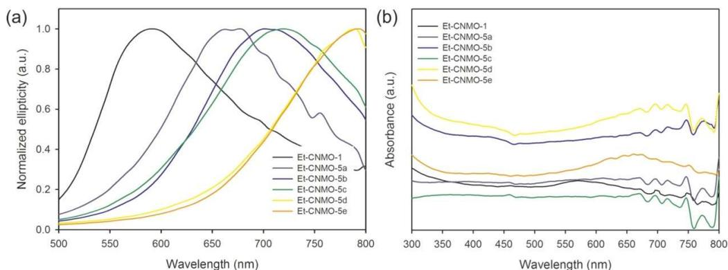
**Figure S11.** (a) CD spectra and (b) UV-vis spectra\* measured for **Et-CNMO-1** and **Et-CNMO-5** organosilica films.
