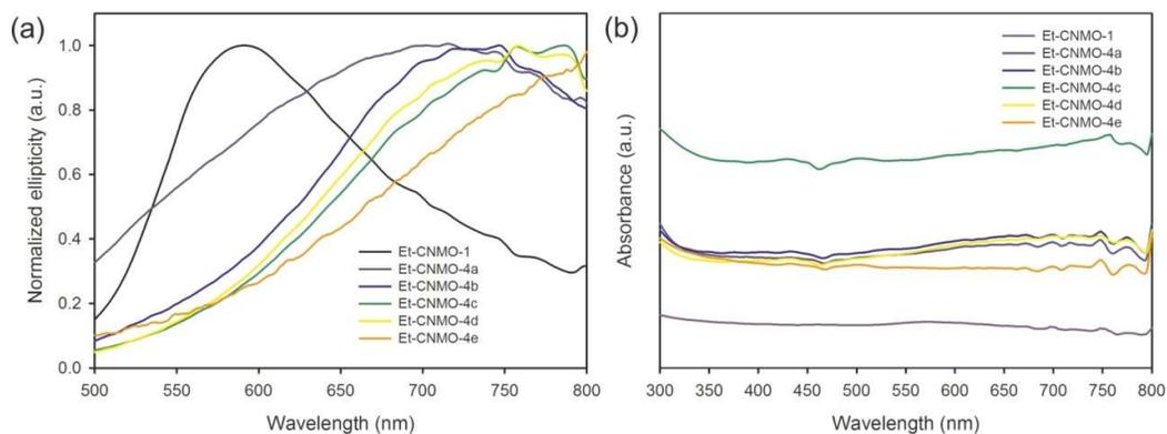
**Figure S10.** (a) CD spectra and (b) UV-vis spectra\* measured for **Et-CNMO-1** and **Et-CNMO-4** organosilica films.
