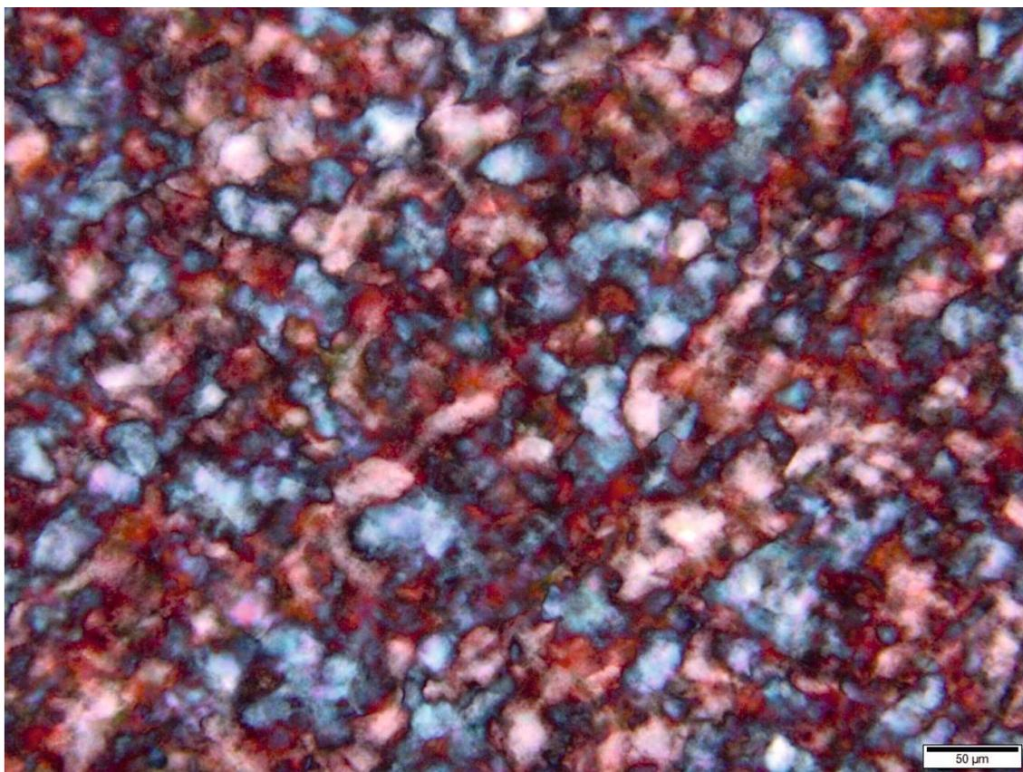
**Figure S15.** Polarized optical microscopy (POM) image of composite **C-1** prepared from organosilica precursor and CNC suspension. Image was captured between crossed polarizers using a 20x objective lens in transmittance mode. Scale bar is 50  $\mu\text{m}$ . Original image included in **Figure 4a** in the manuscript.
