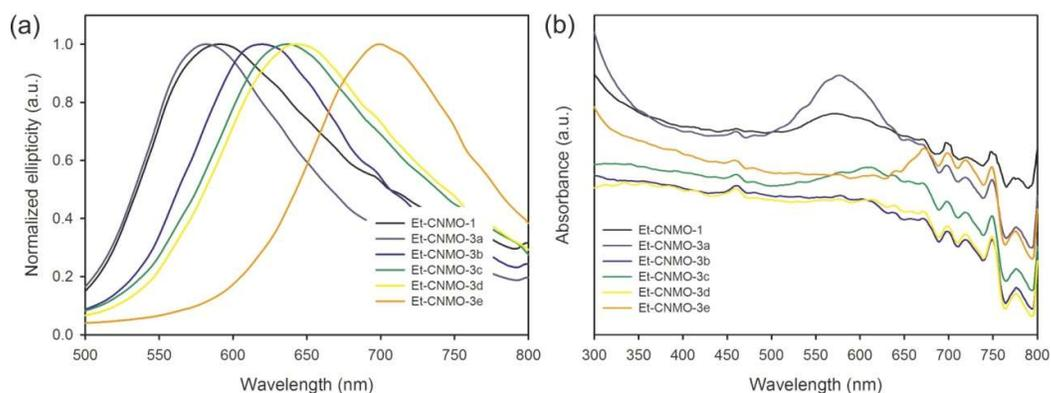
**Figure S9.** (a) CD spectra and (b) UV-vis spectra measured for **Et-CNMO-1** and **Et-CNMO-3** organosilica films.
