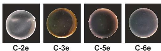
**Figure S2.** Photographs of select non-cracked composite films prepared from CNCs, organosilica precursor and additives (glucose, sucrose, PEG-400 or PEG-20,000). The diameter of each of sample is 2.5 cm.
