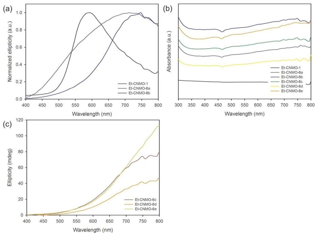
**Figure S12.** (a) CD spectra measured for **Et-CNMO-1** and **Et-CNMO-6a,b** organosilica films. (b) UV-vis spectra measured for **Et-CNMO-1** and **Et-CNMO-6** organosilica films. (c) CD spectra measured for **Et-CNMO-6c-e** organosilica films.
