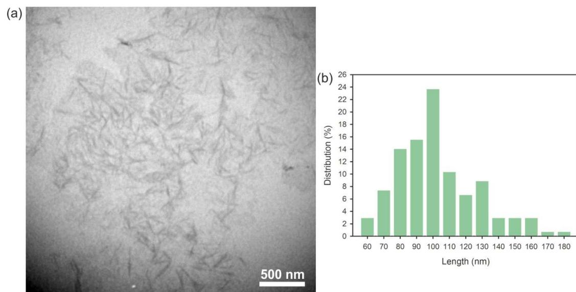
**Figure S1.** (a) TEM image of the CNC suspension. (b) Length distribution of CNCs (number of analyzed nanoparticles: 135). The mean size for CNCs is  $(108 \pm 24)$  nm.
