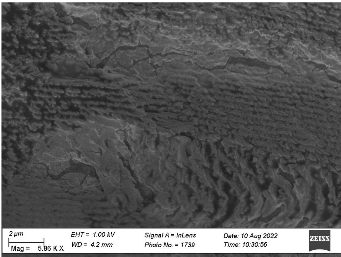
**Figure S20.** SEM image (cross section) of composites prepared from organosilica precursor, CNC suspension and glucose (**C-2e**) – original image included in **Figure 5b** in the manuscript.
