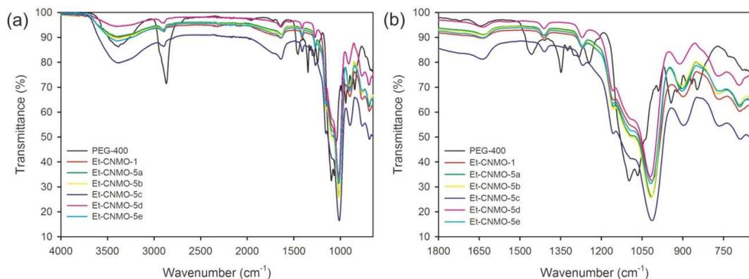
**Figure S6.** IR spectra measured for PEG-400, **Et-CNMO-1** and **Et-CNMO-5**; (a) full spectral range, (b) zoomed range.
