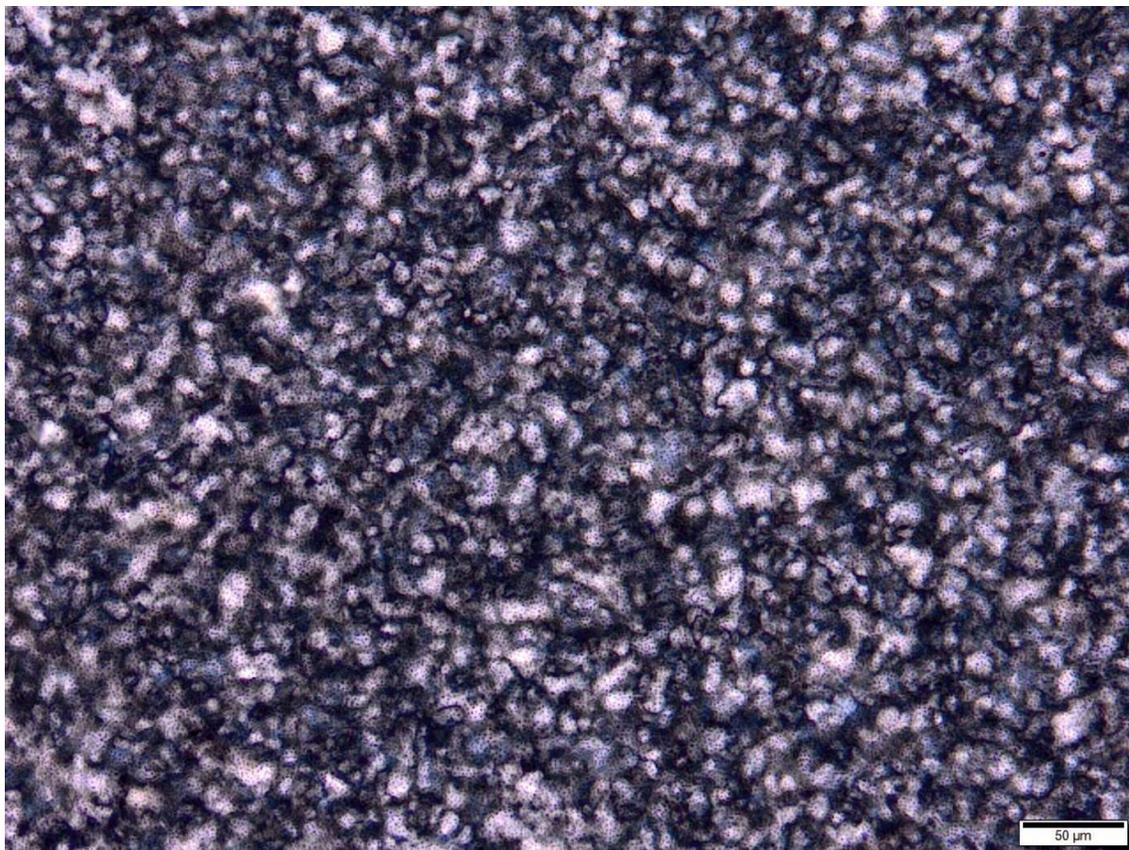
**Figure S16.** Polarized optical microscopy (POM) image of composite **C-3e** prepared from organosilica precursor, CNC suspension and sucrose. Image was captured between crossed polarizers using a 20x objective lens in transmittance mode. Scale bar is 50  $\mu\text{m}$ . Original image included in **Figure 4b** in the manuscript.
