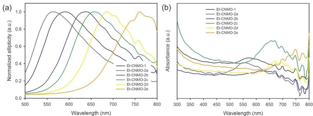
**Figure S8.** (a) CD spectra and (b) UV-vis spectra\* measured for **Et-CNMO-1** and **Et-CNMO-2** organosilica films.
