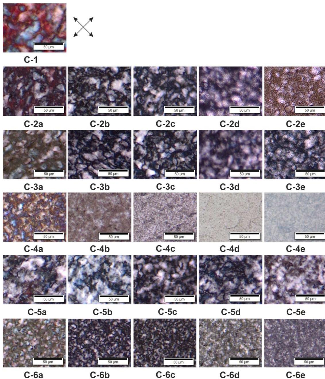
**Figure S13.** Polarized optical microscopy (POM) images of all composite films. Images were captured between crossed polarizers using a 20x objective lens in transmittance mode. Scale bars are 50 μm.
