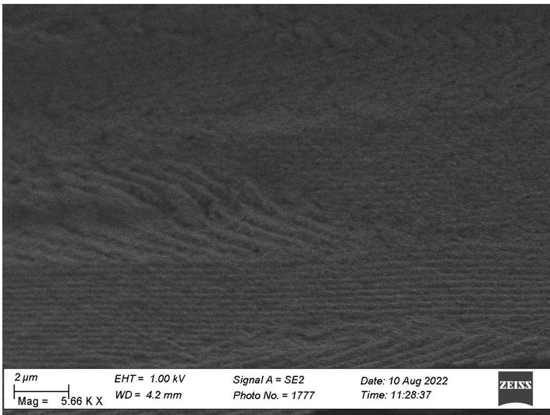
**Figure S22.** SEM image (cross section) of CNMO film prepared from organosilica precursor, CNC suspension and glucose (**Et-CNMO-2e**) – original image included in **Figure 5d** in the manuscript.
