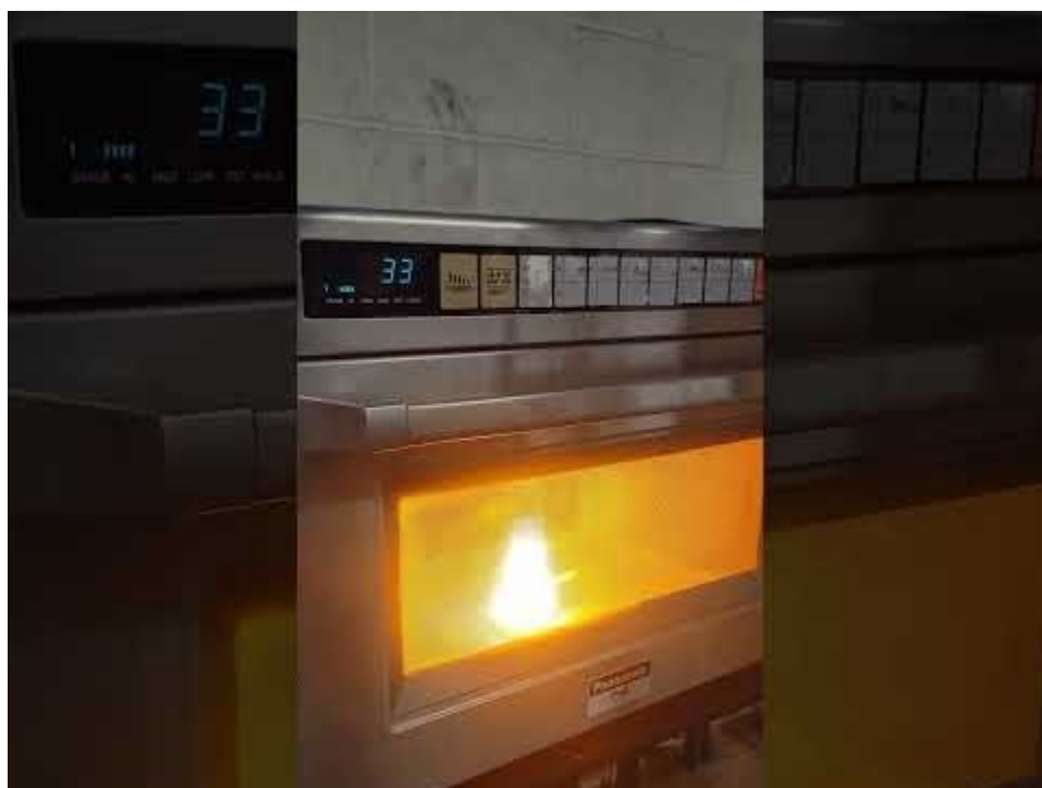
Movie I. C2CNT CNTs from CO 2 ; microwaved 1 minute at 3200 W in a borosilicate (Pyrex) flask. A sustained plasma is evident. Click the video to play, available at https://youtu.be/GRzeSMIZI_c .
