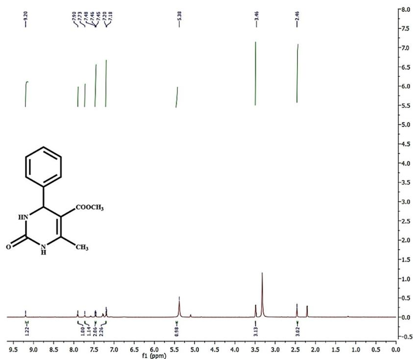
**Fig. S5.** <sup>1</sup>H NMR spectrum of the compound **4a**.
