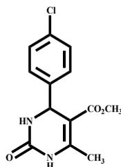
**4c** was prepared as per the general procedure using chlorobenzaldehyde (1.0 mmol, **1**), urea (1.5 mmol, **2**), methyl acetoacetate (1.0 mmol, **3**), and Ethanol (3mL). A brownish yellow colour product obtained. The NMR data are in full agreement with those previously published in the literature. **Yield: 90%**, M.p:178-181; Yield: 90%; M.p:
