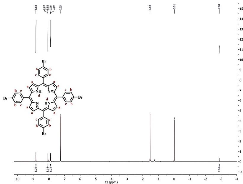
Fig. S13.  $^1\text{H}$ -NMR spectrum of the monomer tetrabromophenyl-porphyrin (**P**).
