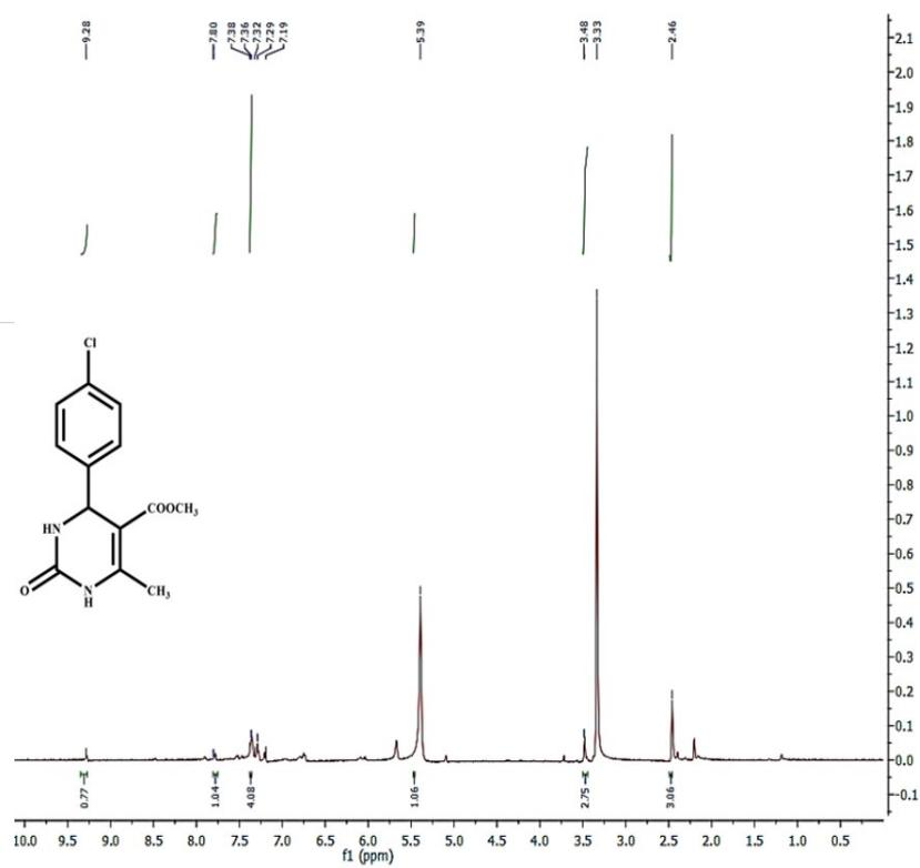
Fig. S9. <sup>1</sup>H-NMR spectrum of the compound 4c.
