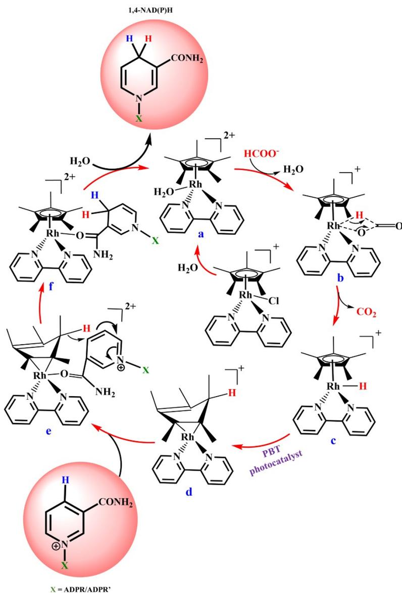
**Scheme S1.** Schematic representation of mechanistic pathway for photoregeneration of 1,4-NAD(P)H cofactor under solar light analogue with reduction of rhodium complex.
