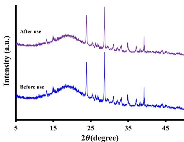
**Fig. S15.** Chemical stability of the PBT photocatalyst through XRD spectra.
