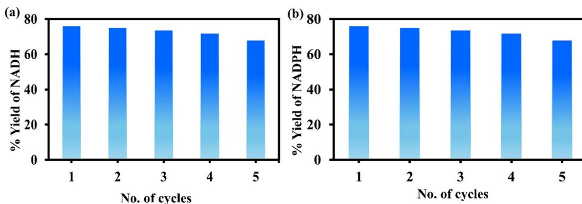
**Fig. S14.** Photocatalytic 1,4-NADH regeneration and (b) Photocatalytic 1,4-NADPH regeneration over multiple cycle (5 cycles) by use of PBT photocatalyst [ $\beta$ - NAD<sup>+</sup>/NADP<sup>+</sup> (1.24 mmol), AsA (1.24 mmol), EM (0.62 mmol) and PBT photocatalyst (0.5 mg)].
