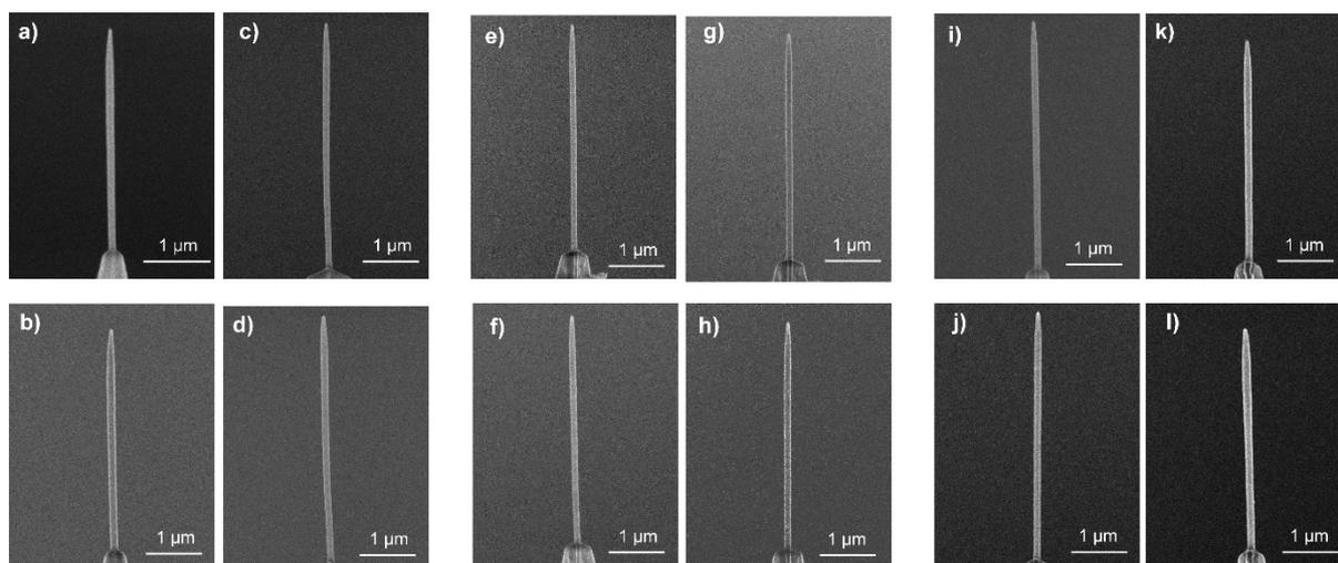
**Figure S4.** SEM images of 120 nm diameter EBD carbon nanoprobes before (a, c, e, g, i, k) and after (b, d, f, h, j, l) the cell penetration experiment: 5 μm/s static (a, b); 5 μm/s dynamic (c, d); 10 μm/s static (e, f); 10 μm/s dynamic (g, h); 30 μm/s static (i, j); 30 μm/s dynamic (k, l).
