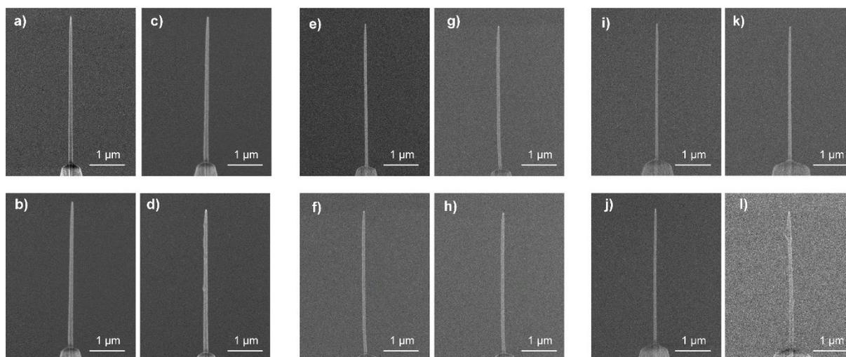
**Figure S5.** SEM images of 80 nm diameter EBD carbon nanoprobes before (a, c, e, g, i, k) and after (b, d, f, h, j, l) the cell penetration experiment: 5 μm/s static (a, b); 5 μm/s dynamic (c, d); 10 μm/s static (e, f); 10 μm/s dynamic (g, h); 30 μm/s static (i, j); 30 μm/s dynamic (k, l).
