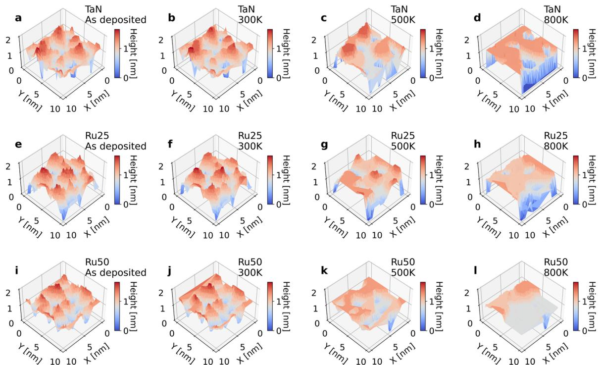
**Figure S15:** Surface of deposited Cu employing a partial pressure of  $P=0.5$  Pa. Rows are different substrates: TaN (a, b, c, d), Ru25 (e, f, g, h) and Ru50 (i, j, k, l). First column represent the film deposited at 500 K for the different substrates, while the other columns are the layer surfaces annealed at varying temperature: 300 K (b, f, j), 500 K (c, g, k) and 800 K (d, h, l).
