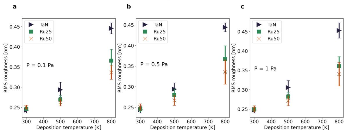
**Figure S11:** RMS roughness for growth simulations conducted on TaN, Ru25 and Ru50 at different temperatures (300 K, 500 K and 800 K) for a range of partial pressures: 0.1 (a), 0.5 (b) and 1 Pa (c). Ten growth simulations were averaged per data point, with error bars as the standard deviation.
