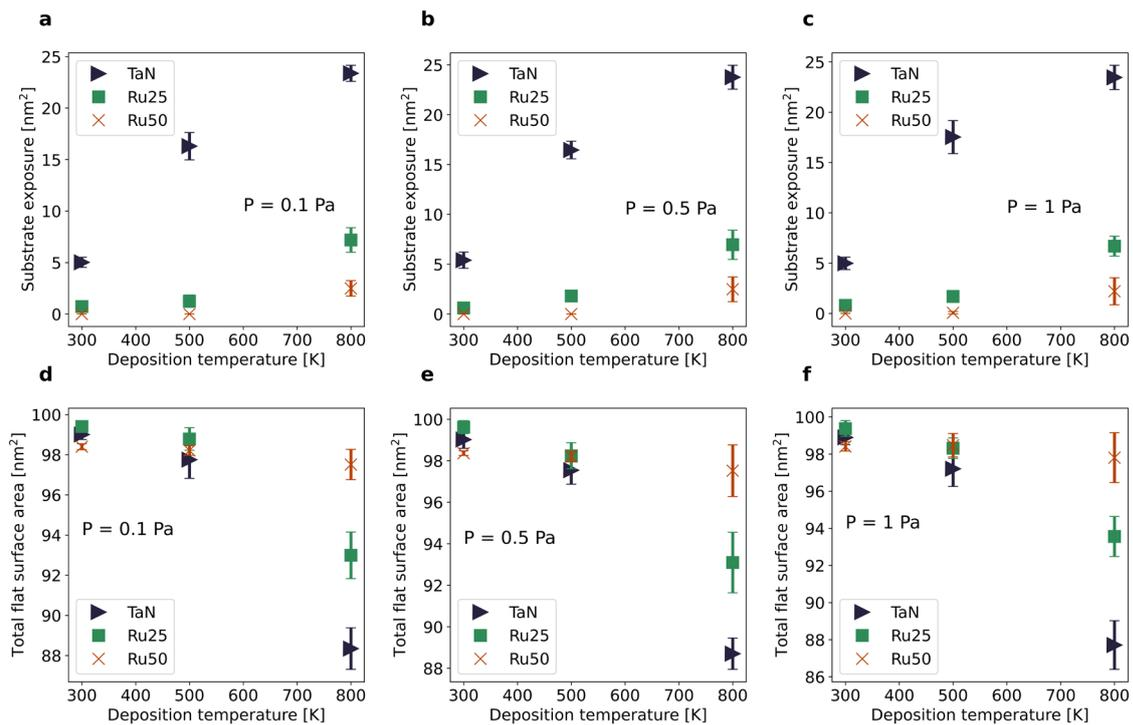
**Figure S13:** Substrate exposure for three partial pressures  $P = 0.1$  Pa (a),  $P = 0.5$  Pa (b) and  $P = 1$  Pa (c). Total uncovered area for three partial pressures  $P = 0.1$  Pa (d),  $P = 0.5$  Pa (e) and  $P = 1$  Pa (f). Ten growth simulations were averaged per data point on TaN, Ru25 and Ru50 at different temperatures (300 K, 500 K and 800 K) across the range of partial pressures. Error bars are the standard deviation.
