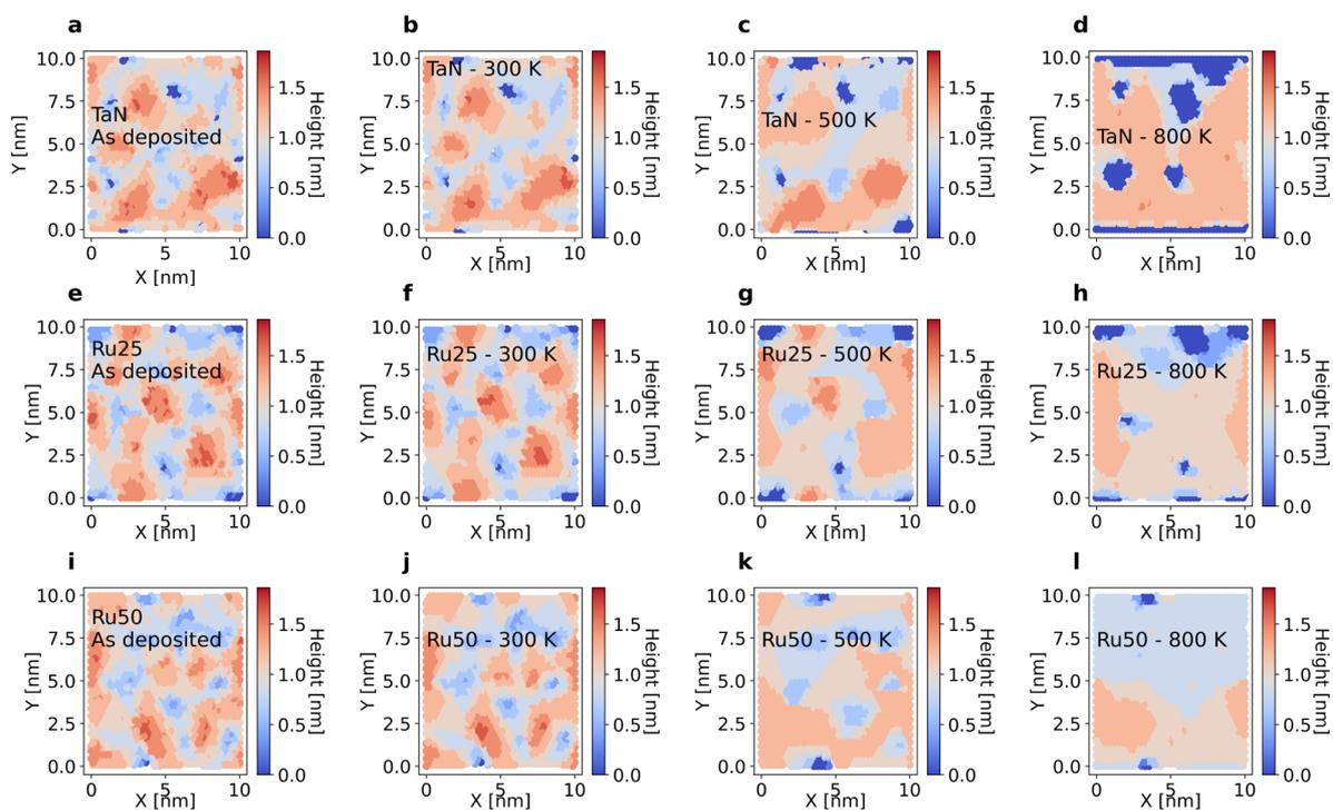
**Figure S16:** Height color maps of deposited Cu employing a partial pressure of  $P=0.5$  Pa. Rows are different substrates: TaN (a, b, c, d), Ru25 (e, f, g, h) and Ru50 (i, j, k, l). First column represent the film deposited at 500 K for the different substrates, while the other columns are the layer surfaces annealed at varying temperature: 300 K (b, f, j), 500 K (c, g, k) and 800 K (d, h, l).
