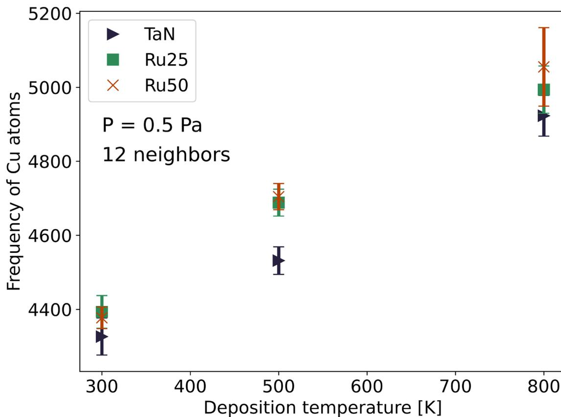
**Figure S14:** Frequency of Cu atoms with 12 nearest neighbors, averaged over 10 simulations, for TaN, Ru25 and Ru50 substrates across temperatures of 300 K, 500 K and 800 K. All simulations were conducted at a partial pressure of  $P = 0.5$  Pa.
