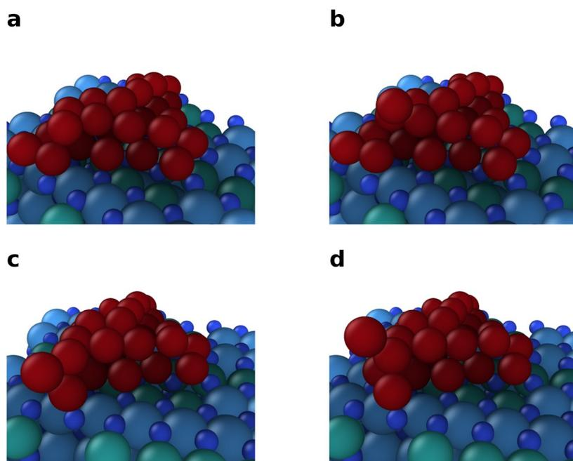
**Figure S6:** Transitions of a Cu atom between adjacent Cu layers deposited on a Ru50 substrate. The transition from state (a) to state (b) requires an activation energy of 0.72 eV, while the transition from state (c) to state (d) requires an activation energy of 0.83 eV.
