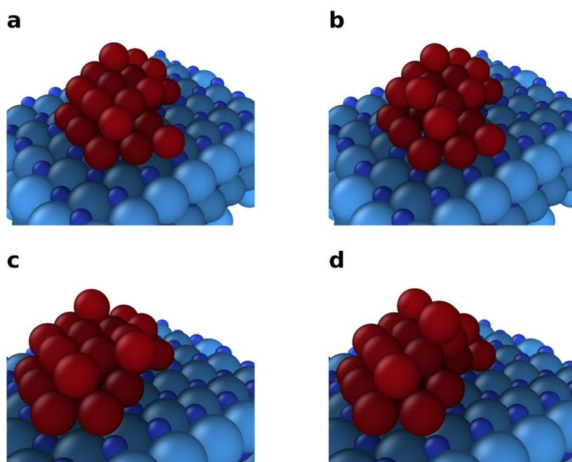
**Figure S4:** Transitions of a Cu atom between adjacent Cu layers deposited on a TaN substrate. The transition from state (a) to state (b) requires an activation energy of 0.69 eV, while the transition from state (c) to state (d) requires an activation energy of 0.22 eV.
