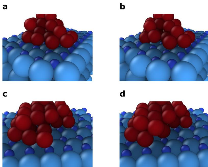
**Figure S1:** Transitions of a Cu atom from the TaN substrate to the upper Cu layer. The transition from state (a) to state (b) requires an activation energy of 0.58 eV, while the transition from state (c) to state (d) requires an activation energy of 0.16 eV.
