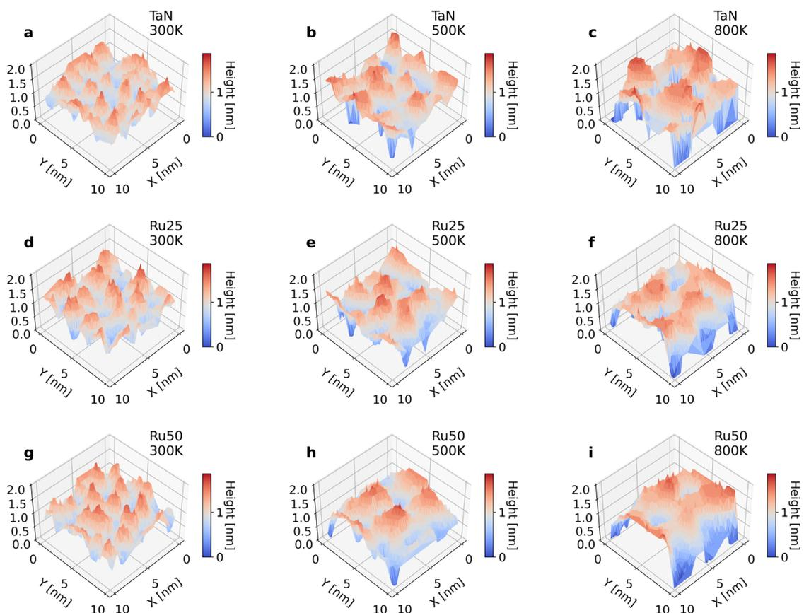
**Figure S7:** Surface of deposited Cu employing a partial pressure of  $P=0.5$  Pa. Rows are different substrates: TaN (a, b, c), Ru25 (d, e, f) and Ru50 (g, h, i). Different columns represent varying temperature: 300 K (a, d, g), 500 K (b, e, h) and 800 K (c, f, i).
