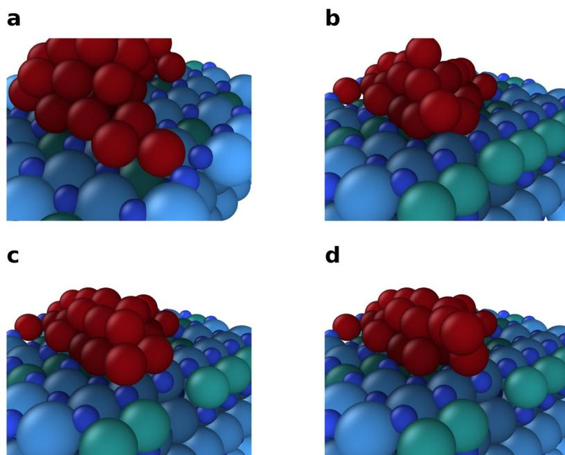
**Figure S3:** Transitions of a Cu atom from the Ru50 substrate to the upper Cu layer. The transition from state (a) to state (b) requires an activation energy of 0.62 eV, while the transition from state (c) to state (d) requires an activation energy of 1.03 eV.
