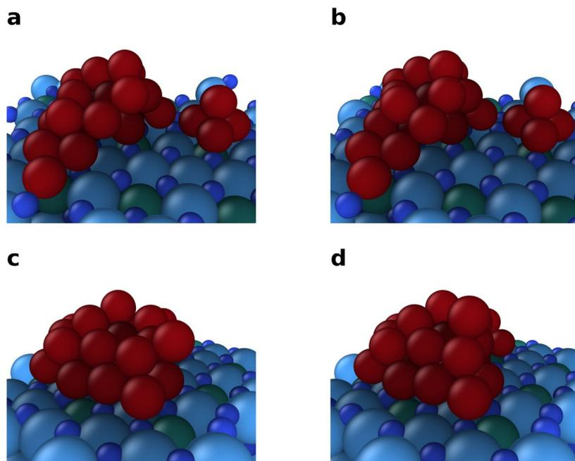
**Figure S5:** Transitions of a Cu atom between adjacent Cu layers deposited on a Ru25 substrate. The transition from state (a) to state (b) requires an activation energy of 0.67 eV, while the transition from state (c) to state (d) requires an activation energy of 0.49 eV.
