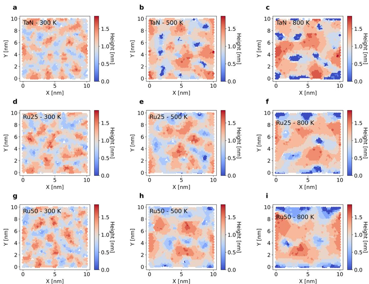
**Figure S8:** Height color maps of deposited Cu employing a partial pressure of  $P=0.5$  Pa. Rows are different substrates: TaN (a, b, c), Ru25 (d, e, f) and Ru50 (g, h, i). Different columns represent varying temperature: 300 K (a, d, g), 500 K (b, e, h) and 800 K (c, f, i).
