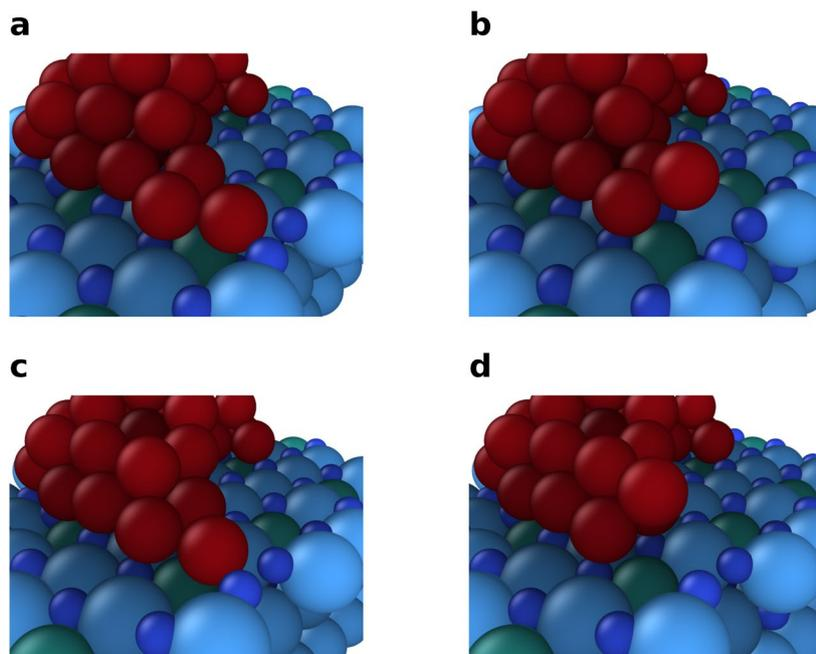
**Figure S2:** Transitions of a Cu atom from the Ru25 substrate to the upper Cu layer. The transition from state (a) to state (b) requires an activation energy of 0.92 eV, while the transition from state (c) to state (d) requires an activation energy of 0.67 eV.
