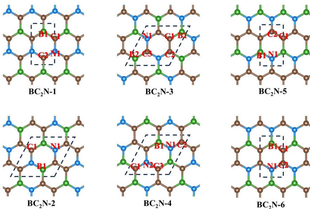
Fig. S1. Position of each atom in unit cell of six BC<sub>2</sub>N structures.
