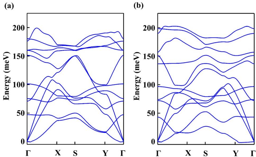
**Fig. S5.** Phonon band structure of (a)  $\text{BC}_2\text{N}$ -5 and (b)  $\text{BC}_2\text{N}$ -6. The phonon band structures of  $\text{BC}_2\text{N}$ -5 and  $\text{BC}_2\text{N}$ -6 do not have obvious phonon imaginary modes in the whole Brillouin zone, which indicates that the monolayer  $\text{BC}_2\text{N}$ -5 and  $\text{BC}_2\text{N}$ -6 are kinetically stable.
