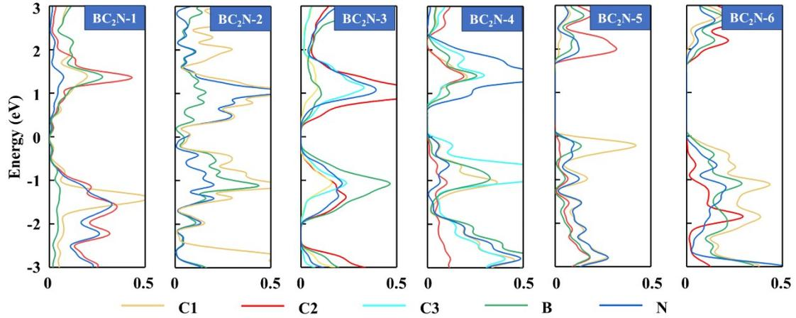
**Fig. S4.** PDOS of six  $\text{BC}_2\text{N}$  structures. The valence band maximum (VBM) of six structures is consisted with B and C atoms. The conduction band minimum (CBM) of  $\text{BC}_2\text{N}$ -1, 2, 3, 4, and 5 is consisted with N and C atoms, while that of  $\text{BC}_2\text{N}$ -6 is contributed by B and C atoms.
