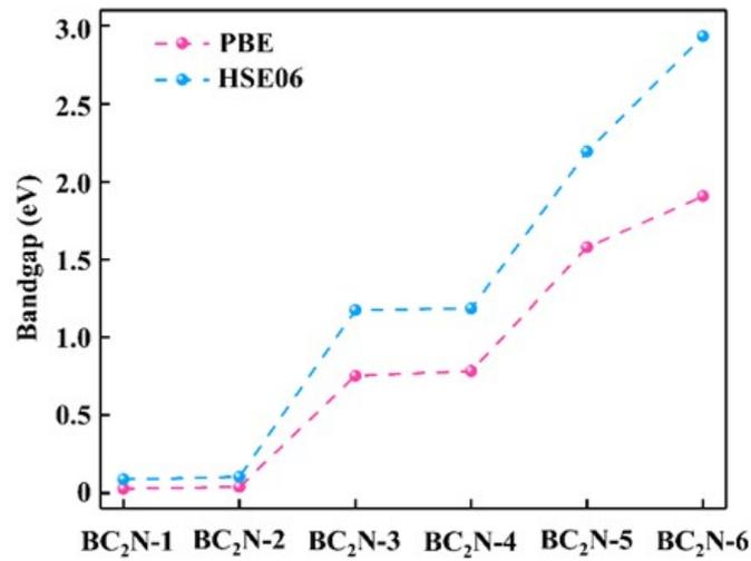
**Fig. S3.** Band gap variation of BC<sub>2</sub>N based PBE and HSE06 calculation. The value of bandgap based HSE calculation is obvious higher than that of PBE calculation, but the trend of bandgap changes obtained by these two methods is consistent.
