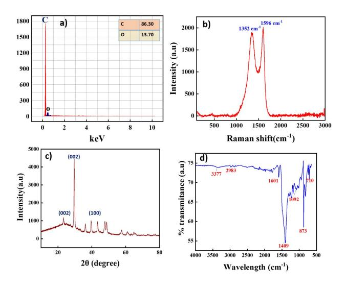
Fig. S1 Characterization of AS900 a) EDS spectra, b) Raman Spectrum, c) XRD d) FTIR analysis.
