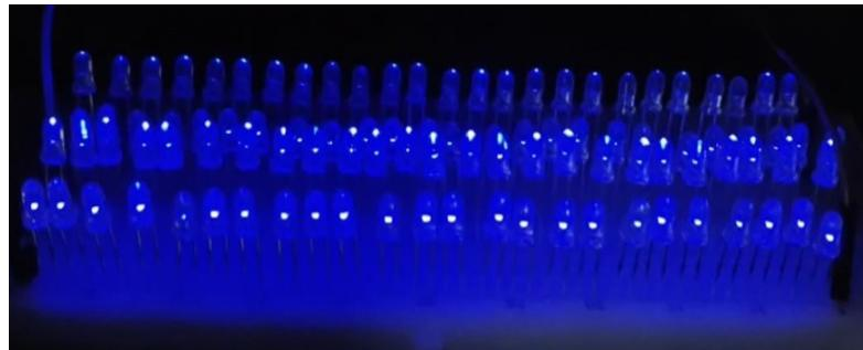
**Fig. S14.** Demonstration experiment of DF-CNF/MXene TENG powering LEDs.
