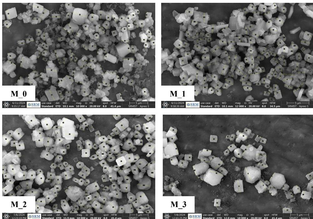
Fig. S2 HRSEM images of pure and doped MOF-5 whose grain size is calculated using imageJ software
