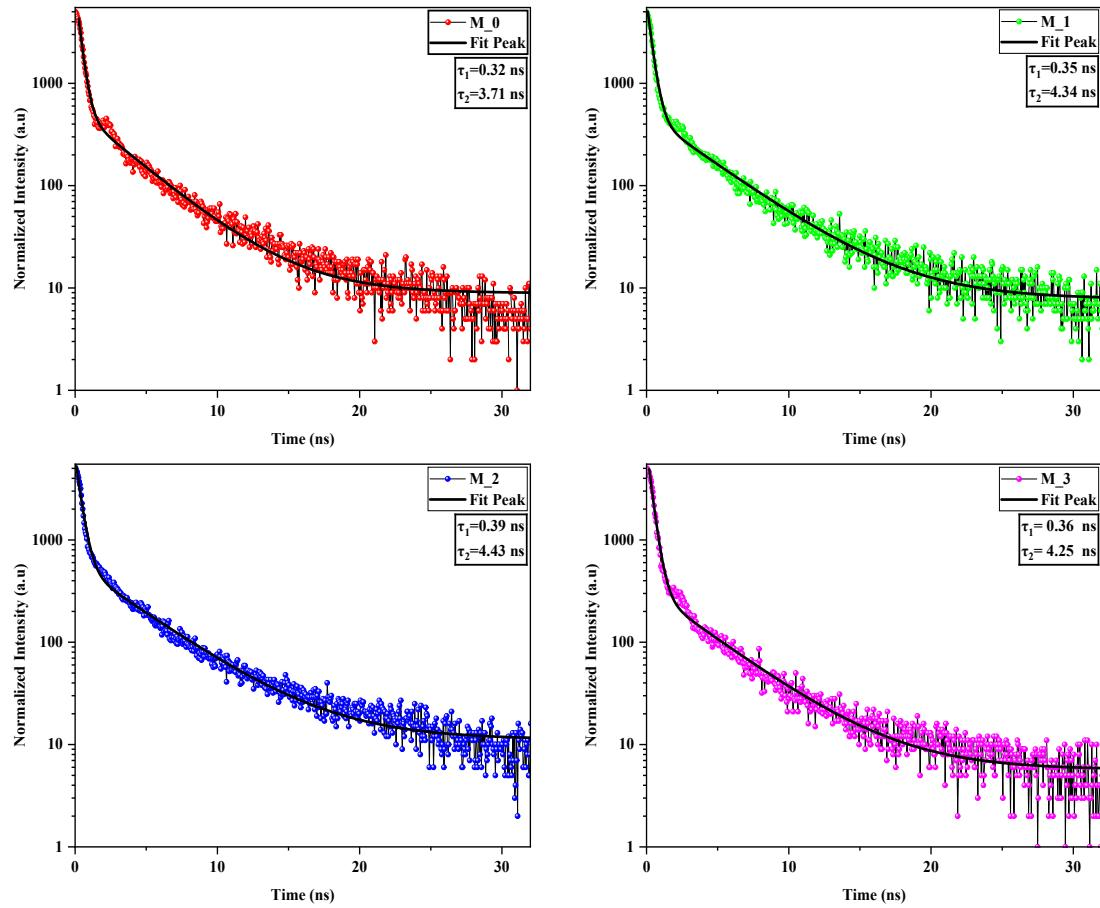
Fig. S6 TR-PL Spectra of the pure and doped MOF-5 samples
