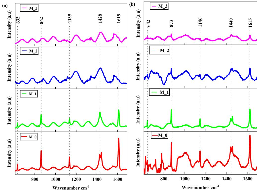
Fig. S5 RAMAN spectra of pure and doped samples (a) using 532 nm, (b) using 633nm
