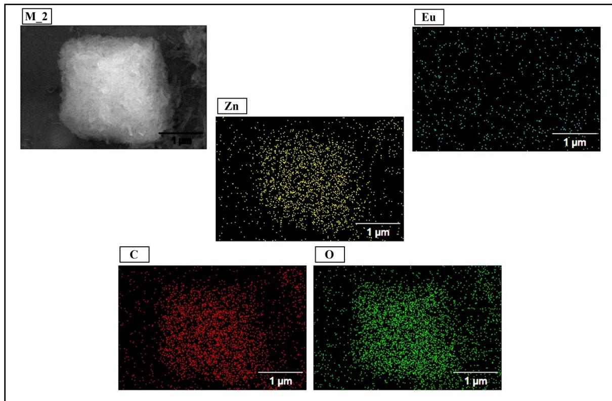
Fig. S3(c) EDS of *M\_2* sample
