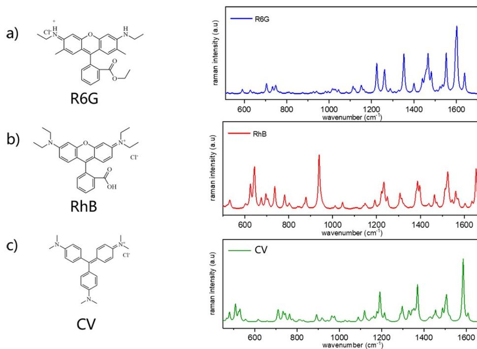
**Figure S3** Molecular Schematics and Raman spectrum of the target molecule calculated using Gaussian. **a.** Simulation of R6G excited by 785 nm light in vacuum. **b.** Simulation of RhB excited by 785 nm light in vacuum. **c.** Simulation of CV excited by 785 nm light in vacuum.
