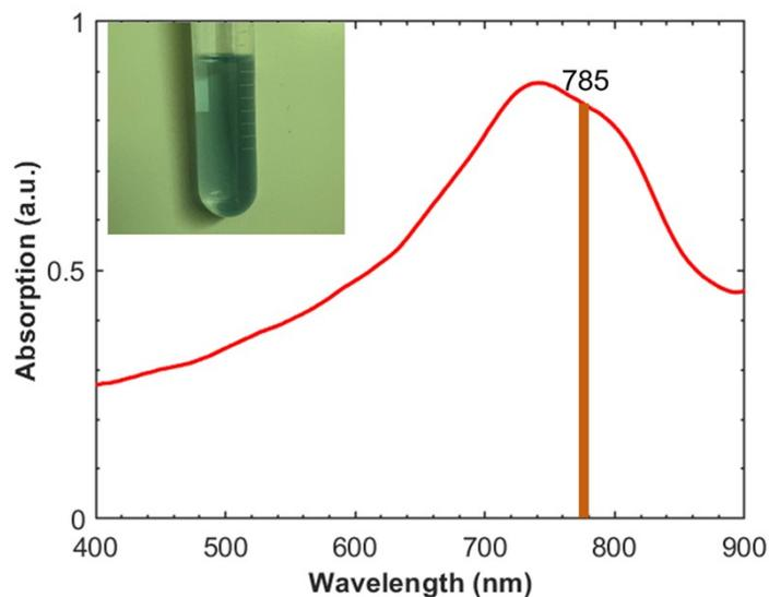
**Figure S2** UV-Vis spectra of the hollow gold nanoparticles
