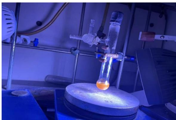
Figure S2. Reaction setup for the sulfonation reactions
