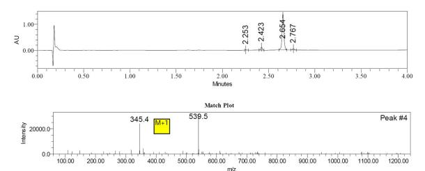
Base Peak 539.49 Channel Description 1: QDa Positive(+) Scan (60.00-1240.00)Da, Centroid, CV=10 - AVG (0.0:1.6;3.5:4.0) x 20.000 Th: 0.010 Retention Time 2.617
