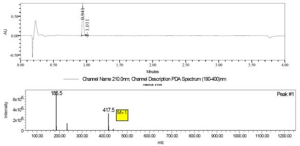
Base Peak 185.48 Channel Description 2: QDa Positive(+) Scan (50.00-1250.00)Da, Centroid, CV=30 - AVG  $(1.4:3.9;0.1:0.8) \times 30.000$  Retention Time 0.965
