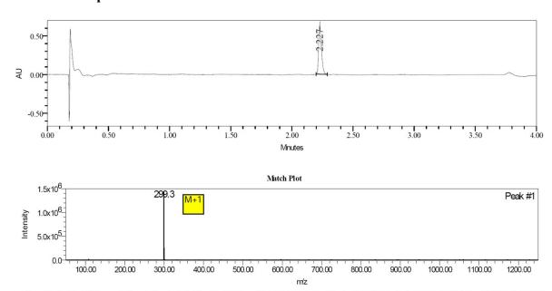
Base Peak 299.25 Channel Description 1: QDa Positive(+) Scan (50.00-1250.00)Da, Centroid, CV=10 - AVG (2.4:3.9;0.3:2.1) x 20.000 Th: 0.200 Retention Time 2.258
