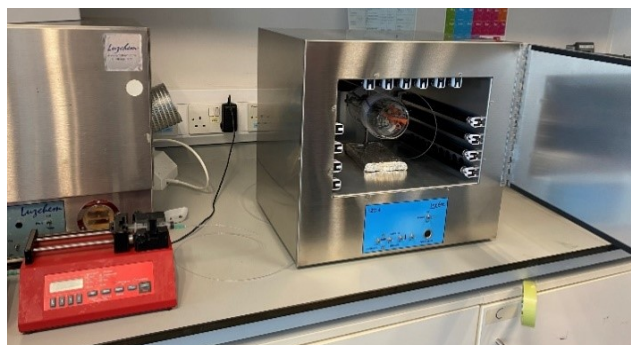
Dual syringe pump, FEP coil in UV oven.
