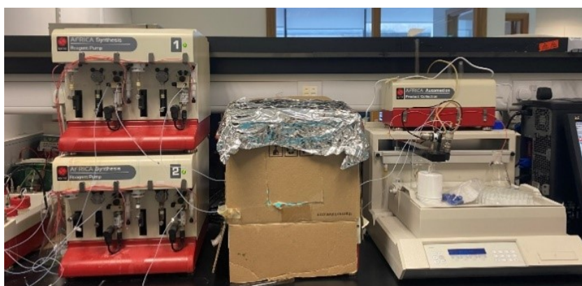
Figure S1: Integrated Syrris Ltd. continuous flow system located in O'Shea Laboratory (Royal College of Surgeons in Ireland, RCSI, York House, York Street, Dublin 2, Ireland) on which initial radical mediated thiol-ene chemistry optimisation was carried out.
