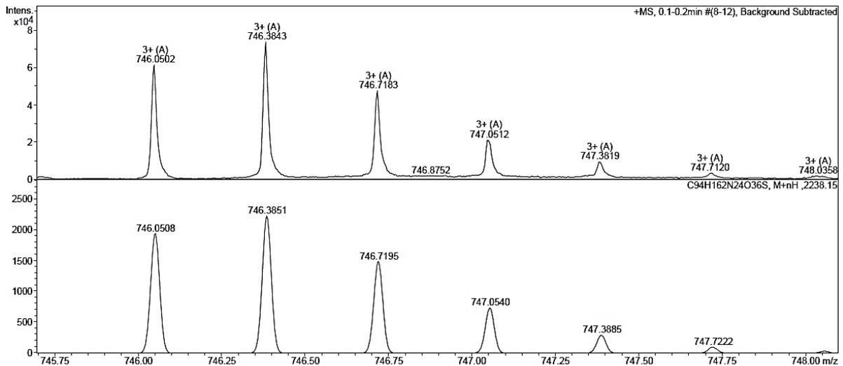
Figure S11: HR-MS spectrum of Pep1-CML (I) ( $[M+3H]^{3+}$ ).
