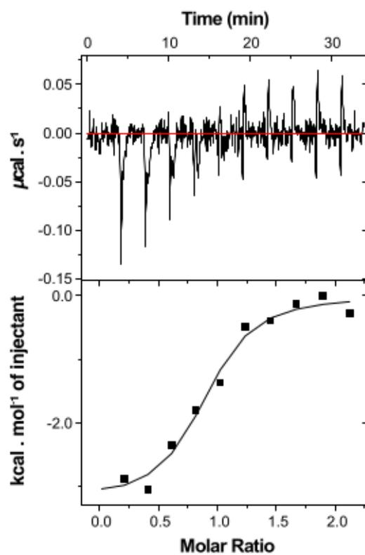
Figure S2. Isothermal titration calorimetry of octyl-SQ titrated into SmoF from *Agrobacterium tumefaciens*. SmoF was at 30  $\mu\text{M}$ .
