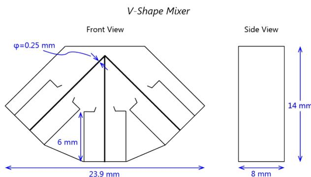
**Fig. S-1.** V-shape mixers used in this study
