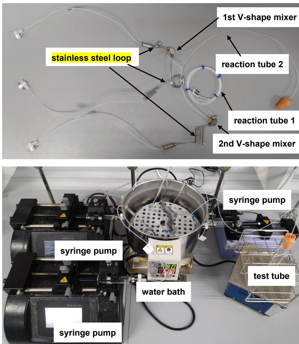
Fig. S-2. Microflow reactor setup
