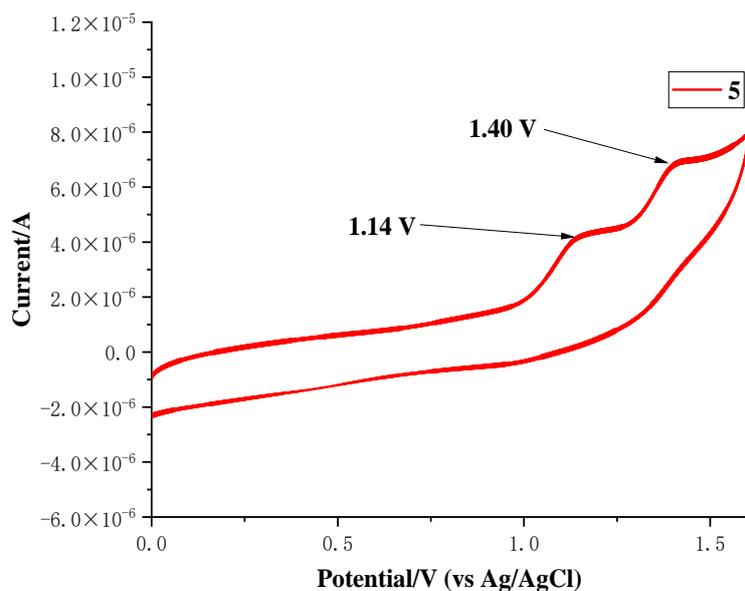
**Figure S5:** Cyclic voltammograms of **5** (2-isothiocyanatonaphthalene) following IUPAC convention. A three-electrode configuration having a glassy carbon as a working electrode, platinum wire as a counter electrode, and Ag/AgCl as a reference electrode in 0.1 M  $n\text{Bu}_4\text{NBF}_4$  in DMF (6 mL) was used. Scan rate: 0.1 V/s.
