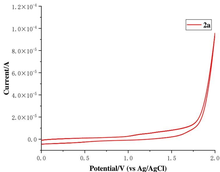
**Figure S3:** Cyclic voltammograms of **2a** (elemental sulfur) following IUPAC convention. A three-electrode configuration having a glassy carbon as a working electrode, platinum wire as a counter electrode, and Ag/AgCl as a reference electrode in 0.1 M  $n\text{Bu}_4\text{NBF}_4$  in DMF (6 mL) was used. Scan rate: 0.1 V/s.
