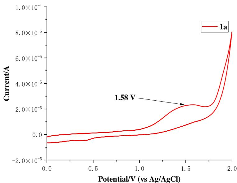
**Figure S2:** Cyclic voltammograms of **1a** (2-isocyanonaphthalene) following IUPAC convention. A three-electrode configuration having a glassy carbon as a working electrode, platinum wire as a counter electrode, and Ag/AgCl as a reference electrode in 0.1 M <sup>n</sup>Bu<sub>4</sub>NBF<sub>4</sub> in DMF (6 mL) was used. Scan rate: 0.1 V/s.
