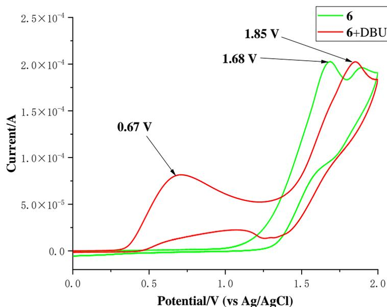
**Figure S6:** Cyclic voltammograms of **6** (1,1-diethyl-3-(naphthalen-2-yl)thiourea) following IUPAC convention. A three-electrode configuration having a glassy carbon as a working electrode, platinum wire as a counter electrode, and Ag/AgCl as a reference electrode in 0.1 M  $n\text{Bu}_4\text{NBF}_4$  in DMF (6 mL) was used. Scan rate: 0.1 V/s.
