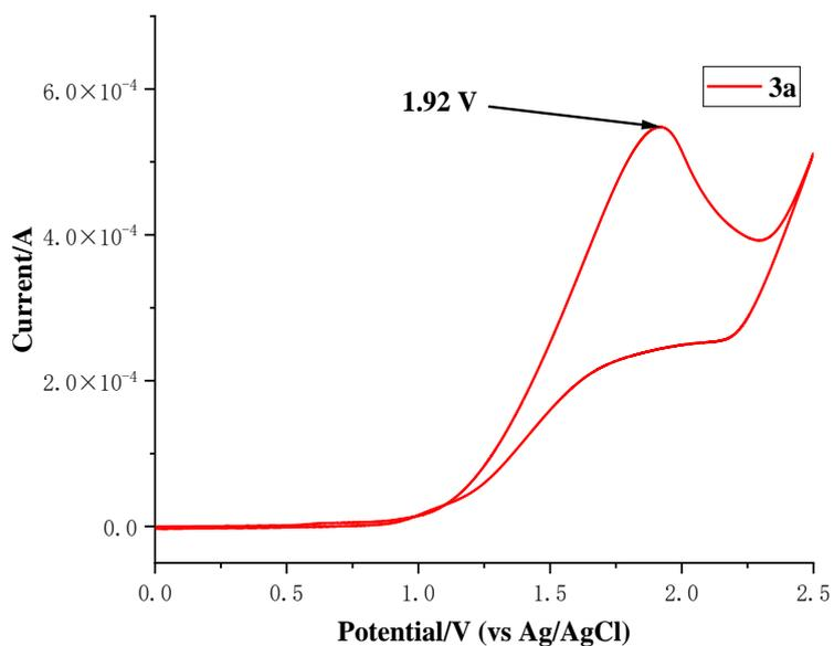
**Figure S4:** Cyclic voltammograms of **3a** (diethylamine) following IUPAC convention. A three-electrode configuration having a glassy carbon as a working electrode, platinum wire as a counter electrode, and Ag/AgCl as a reference electrode in 0.1 M  $n\text{Bu}_4\text{NBF}_4$  in DMF (6 mL) was used. Scan rate: 0.1 V/s.
