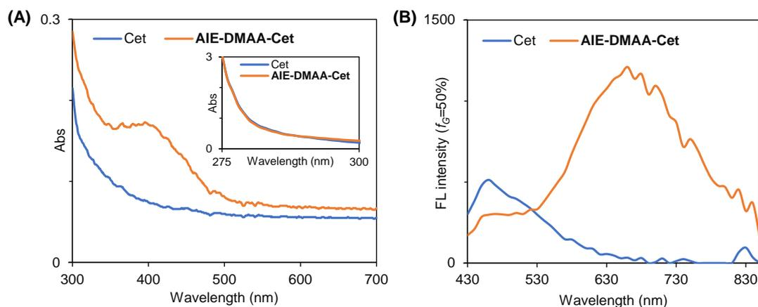
**Fig. S1** Characterizing the successful labeling of AIEgen in **AIE-DMAA-Cet** according to the (A) absorption (in PBS) and (B) emission spectra (PBS/glycerol = 1:1) in comparison with the non-labeled cetuximab (Cet for short). **AIE-DMAA-Cet** and Cet at the same protein concentration (with identical absorption at 280 nm as shown in the inset of (A)) were analyzed in parallel.
