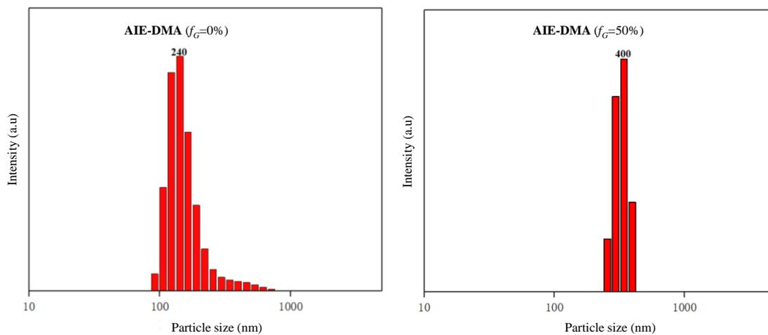
**Fig. S2** Hydrodynamic particle size of **AIE-DMA** in the water/glycerol (G) mixture with  $f_G = 0\%$  or  $50\%$  as measured by the method of dynamic light scattering (DLS).
