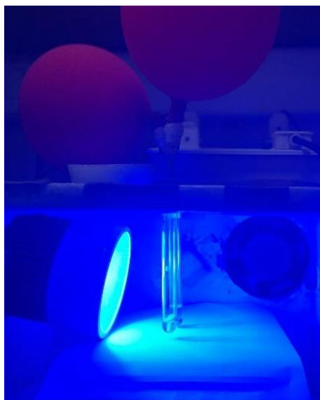
Fig S1: (a) Blue LED photoreactor setup with magnetic stirring plate. (b) Emission profile of the LED.
