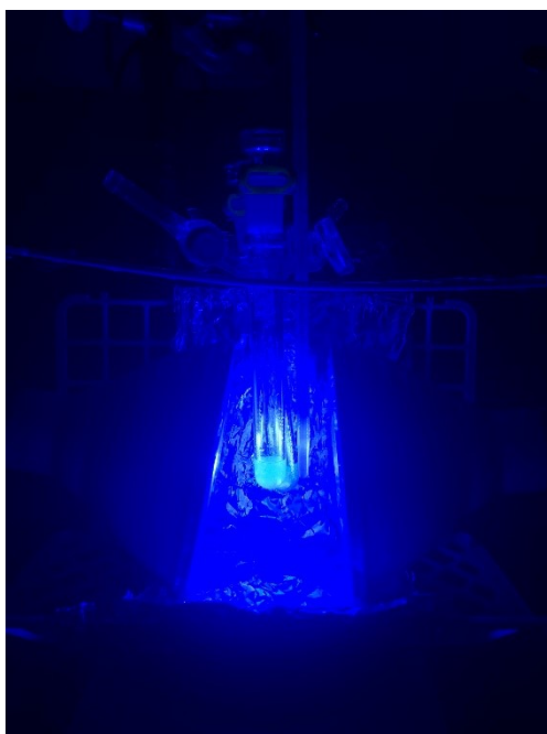
Figure S1 Photo of reaction setup with two 8 W blue LED bulbs.
