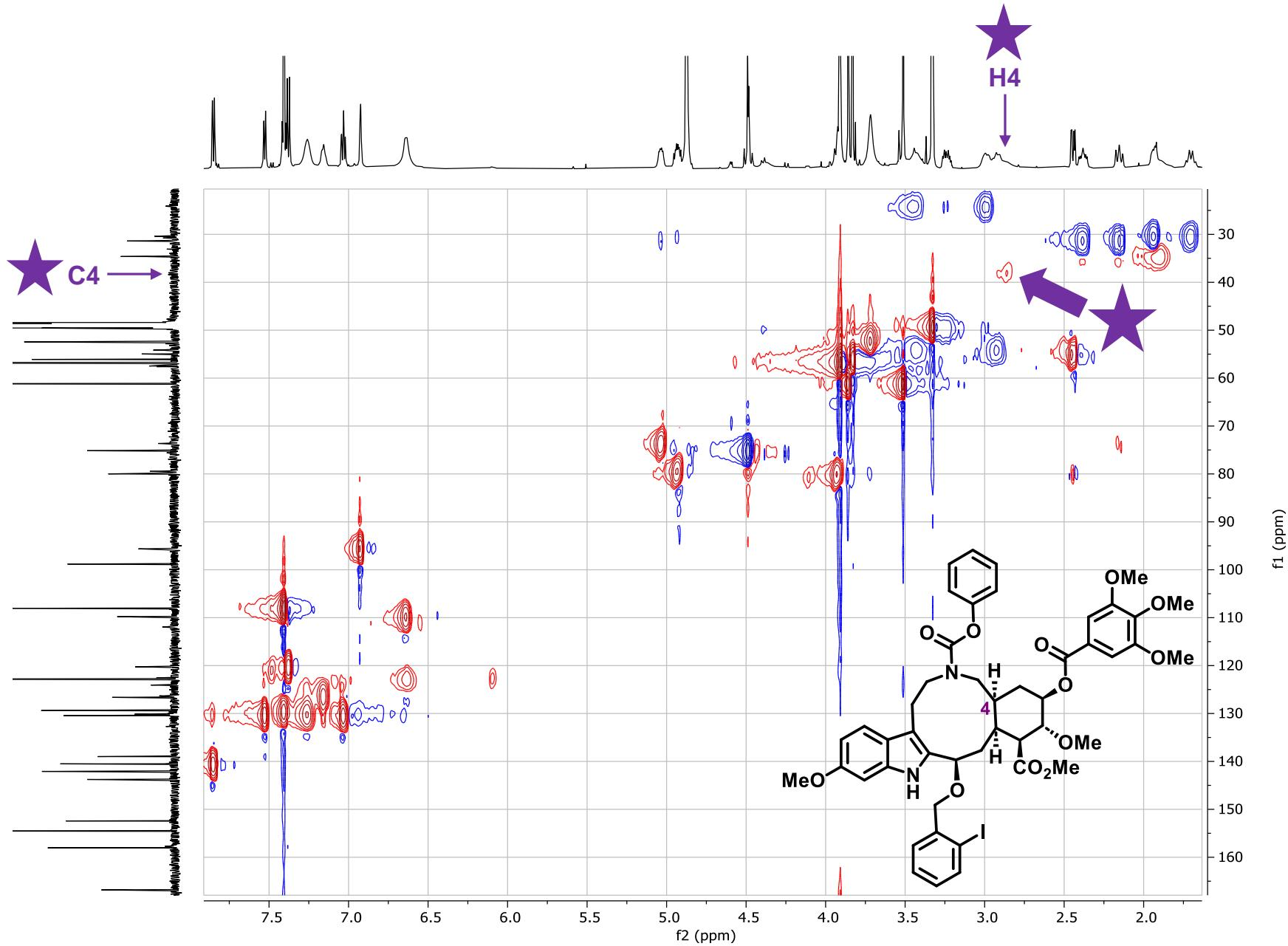
**Compound 40:** HSQC, MeOD-*d*4 (full, increased signal intensity to characterize the C13 signal for C4)
