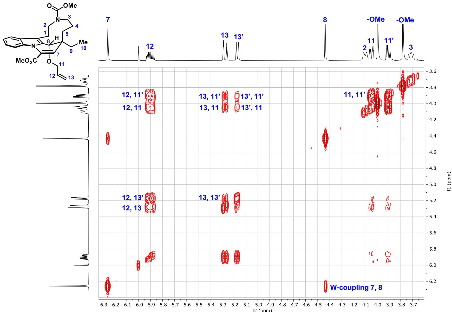
Compound 72: COSY,  $T = 100\text{ }^{\circ}\text{C}$ ,  $\text{C}_2\text{D}_2\text{Cl}_4$  (zoomed in, version 1). Allylic coupling observed between protons at 11 and 13.
