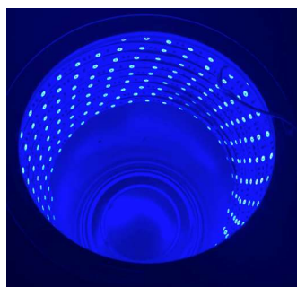
Figure S5. LED strip setup used for irradiation experiments (blue-light photoreactor for irradiation at 467 nm).
