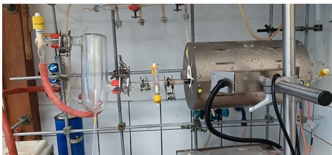
Picture 2 Apparatus for the flash Vacuum Thermolysis of allylamines 4a-4d at 800°C
