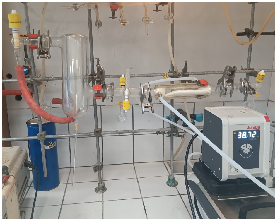
Picture 1 Apparatus for the gas solid reaction of \alpha -aminonitriles 2a-2d on KOH heated to 90°C
