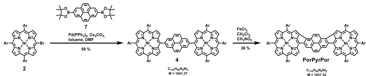
**Scheme S4.** Synthesis of fused bis-porphyrin-pyrene **PorPyrPor**.
