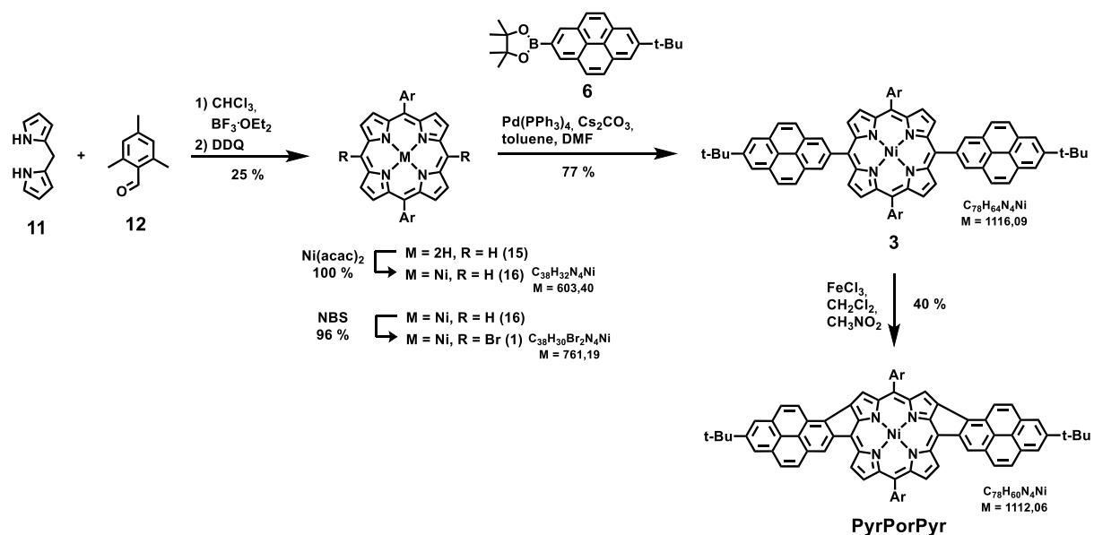
**Scheme S3.** Synthesis of double-fused Bis-Pyrene-Porphyrin **PyrPorPyr**.
