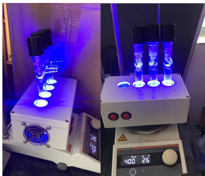
Figure S1 Photoreactor used in this research (6 W blue LEDs, \lambda_{\text{max}} = 450 \text{ nm} ) 1
