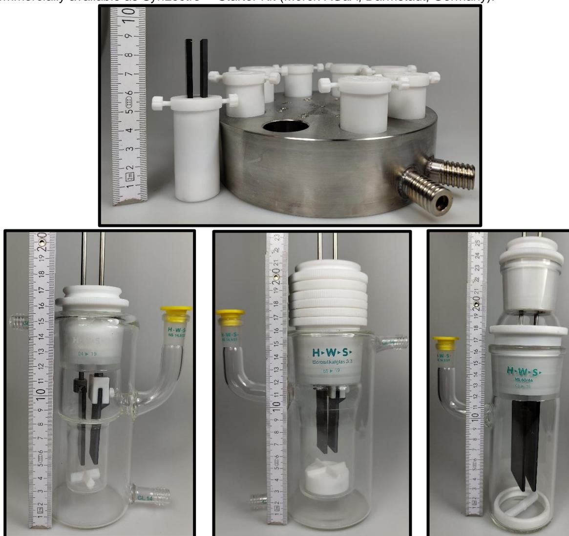
Figure S3: Different batch-type cells; size compared to a ruler: top: 5 mL undivided Teflon™ screening cells with glassy carbon and BDD electrodes and screening cell holder with integrated radiator loop; bottom left: 25 mL undivided glass cell with glassy carbon and BDD electrodes; bottom centre: 100 mL undivided glass cell with glassy carbon and BDD electrodes; bottom right: 300 mL divided glass cell with glassy carbon and BDD electrodes.<sup>3</sup>
