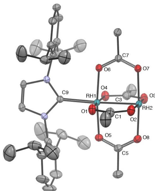
ORTEP drawing with thermal ellipsoids drawn at the 30% probability level. Hydrogens were omitted for clarity. Selected bond distances and angles are presented: Rh1–Rh2 = 2.427(2) Å, Rh1–C9 = 2.143(10) Å; All of the coordination angles are around 90°.
