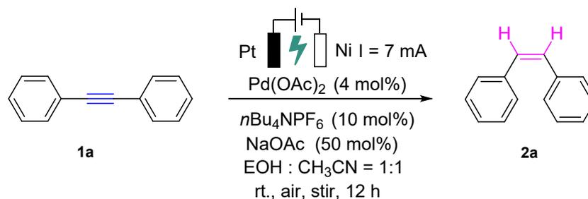
**Standard condition:** 1,2-diphenylethyne (1.0 mmol), Pd(OAc)<sub>2</sub> (0.04 mmol), *n*BuNPF<sub>6</sub> (0.5 mmol), NaOAc (0.5 mmol), platinum plate electrodes (10 × 10 × 0.2 mm) as anode, nickel plate electrodes (10 × 10 × 0.2 mm) as cathode. 10 mL ethanol acetonitrile mixed solvent (MeCN : EtOH = 1 : 1) is used as the reaction solvent in undivided cell. At room temperature, the reaction was carried out for 12 hours at 7 mA constant current (3.1 F/mol).
