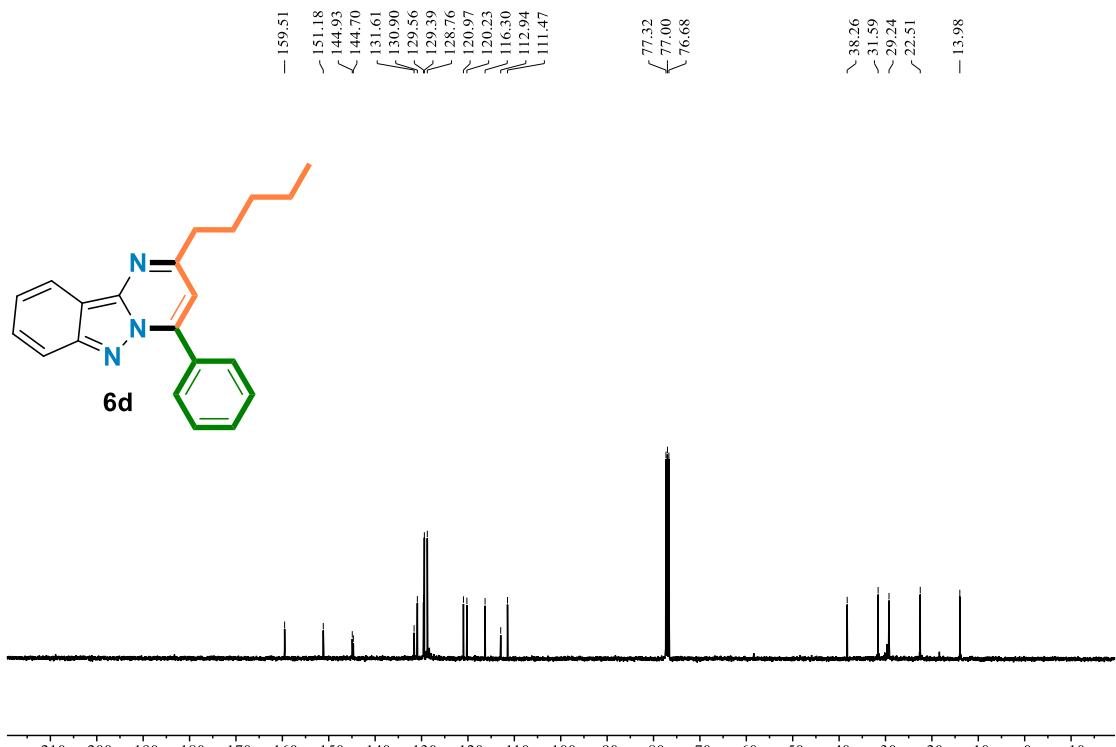
13C{<sup>1</sup>H} NMR Spectrum of Compound **6d** (100 MHz, CDCl<sub>3</sub>)
