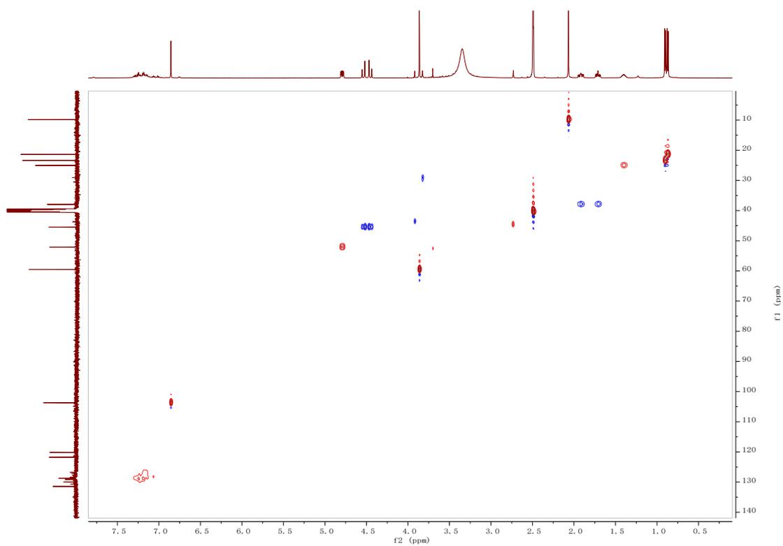
**Figure S10.** HSQC spectrum of leucylchlorine (**2**).
