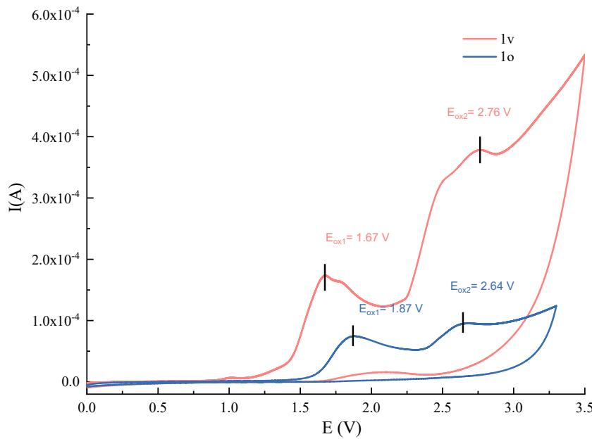
**Figure S2.** Cyclic voltammetry experiments of **1o** and **1v** in DCM:HFIP (5:1) with 0.1 M  $\text{Bu}_4\text{NBF}_4$ , the scan rate is 0.1 V/s. The working electrode was a glassy carbon electrode, the counter electrode was a platinum wire, and the reference electrode was a  $\text{Ag}/\text{AgCl}$  electrode.
