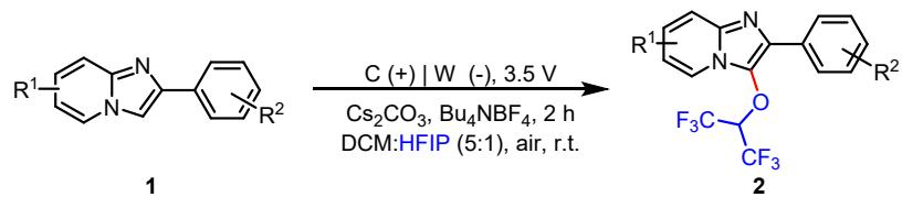
The Electrasyn vial cap was connected to the Electrasyn 2.0 and the reaction mixture was electrolyzed under a constant voltage of 3.5 V. Graphite plate was used as the anode, and
