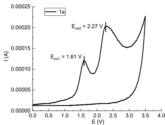
**Figure S1.** Cyclic voltammetry experiments of **1a** in DCM:HFIP (5:1) with 0.1 M  $Bu_4NBF_4$ , the scan rate is 0.1 V/s. The working electrode was a glassy carbon electrode, the counter electrode was a platinum wire, and the reference electrode was a Ag/AgCl electrode.
