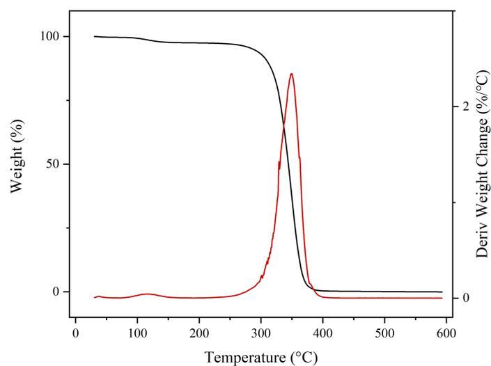
**Fig. S15.** TGA and DTG curves for P[(C6DO)<sub>800</sub>-co-(L-LA)<sub>200</sub>] obtained by [C6DO]/[L-LA]/[Zn1]/[I] = 800/200/1/1,  $T_{d,5\%} = 287\text{ }^{\circ}\text{C}$ ,  $T_{\text{max}} = 350\text{ }^{\circ}\text{C}$ .
