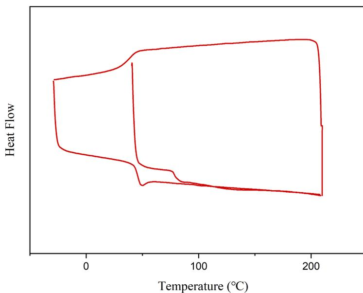
**Fig. S18.** DSC curves for P[(C6DO)<sub>500</sub>-co-(L-LA)<sub>500</sub>] obtained by [C6DO]/[L-LA]/[Zn1]/[I] = 500/500/1/1,  $T_g = 46$  °C.
