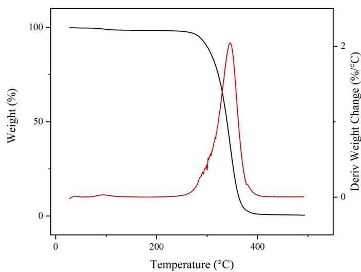
**Fig. S13.** TGA and DTG curves for P[(C6DO)<sub>500</sub>-co-(L-LA)<sub>500</sub>] obtained by [C6DO]/[L-LA]/[Zn1]/[I] = 500/500/1/1,  $T_{d,5\%} = 284\text{ }^{\circ}\text{C}$ ,  $T_{\max} = 345\text{ }^{\circ}\text{C}$ .
