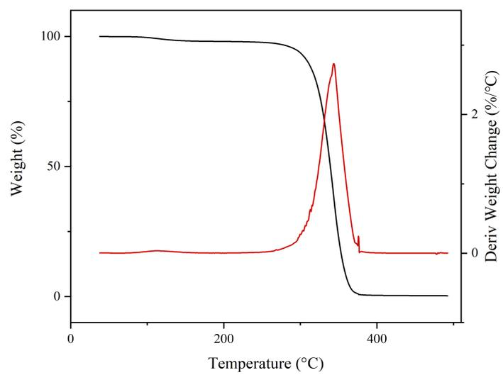
**Fig. S16.** TGA and DTG curves for P[(C6DO)<sub>900</sub>-co-(L-LA)<sub>100</sub>] obtained by [C6DO]/[L-LA]/[Zn1]/[I] = 900/100/1/1,  $T_{d,5\%} = 294$  °C,  $T_{max} = 344$  °C.
