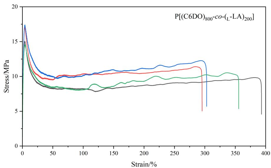
**Fig. S27.** Stress-strain curves of P[(C6DO)<sub>800</sub>-co-(L-LA)<sub>200</sub>].
