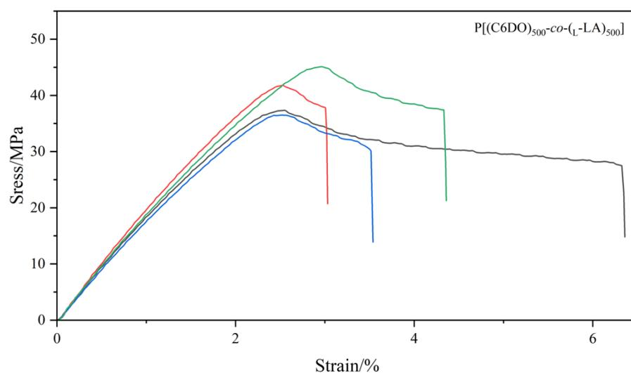
**Fig. S25.** Stress-strain curves of P[(C6DO)<sub>500</sub>-co-(L-LA)<sub>500</sub>].
