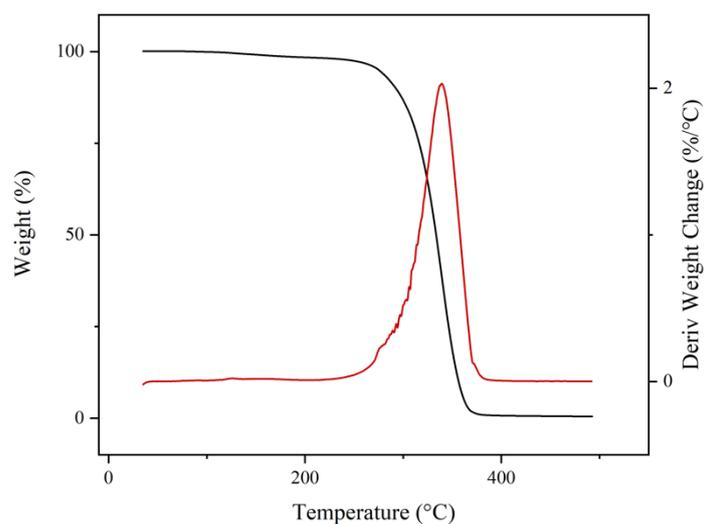
**Fig. S14.** TGA and DTG curves for P[(C6DO)<sub>667</sub>-co-(L-LA)<sub>333</sub>] obtained by [C6DO]/[L-LA]/[Zn1]/[I] = 667/333/1/1,  $T_{d,5\%} = 275\text{ }^{\circ}\text{C}$ ,  $T_{\text{max}} = 339\text{ }^{\circ}\text{C}$ .
