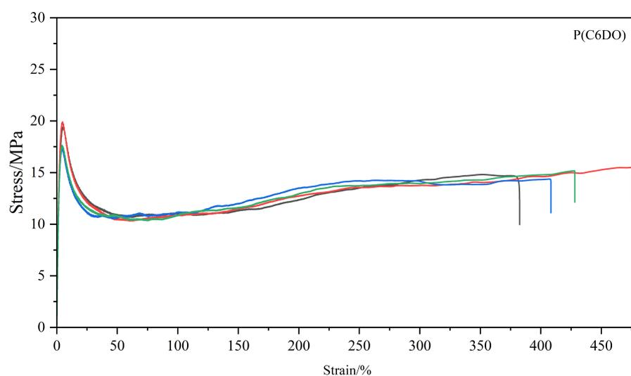
**Fig. S24.** Stress-strain curves of P(C6DO).
