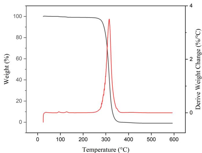
**Fig. S12.** TGA and DTG curves for P(C6DO) obtained by [C6DO]/[Zn1]/[I] = 100/1/1,  $T_{d,5\%} = 283\text{ }^{\circ}\text{C}$ ,  $T_{\max} = 316\text{ }^{\circ}\text{C}$ .
