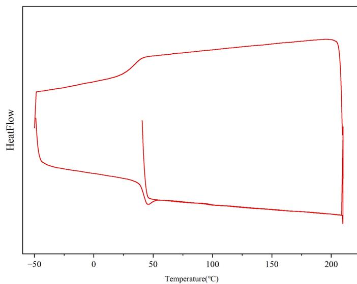
**Fig. S20.** DSC curves for P[(C6DO)<sub>800</sub>-co-(L-LA)<sub>200</sub>] obtained by [C6DO]/[L-LA]/[Zn1]/[I] = 800/200/1/1,  $T_g = 42$  °C.
