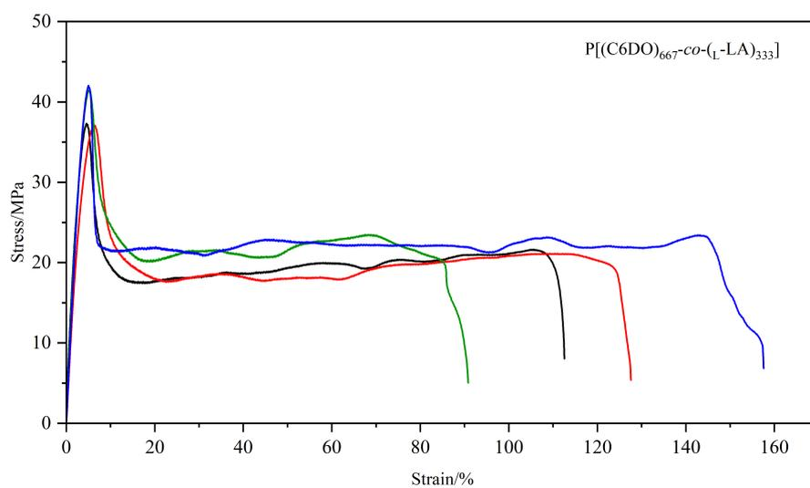
**Fig. S26.** Stress-strain curves of P[(C6DO)<sub>667</sub>-co-(L-LA)<sub>333</sub>].
