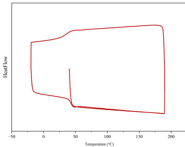
**Fig. S19.** DSC curves for P[(C6DO)<sub>667</sub>-co-(L-LA)<sub>333</sub>] obtained by [C6DO]/[L-LA]/[Zn1]/[I] = 667/333/1/1,  $T_g = 43$  °C.
