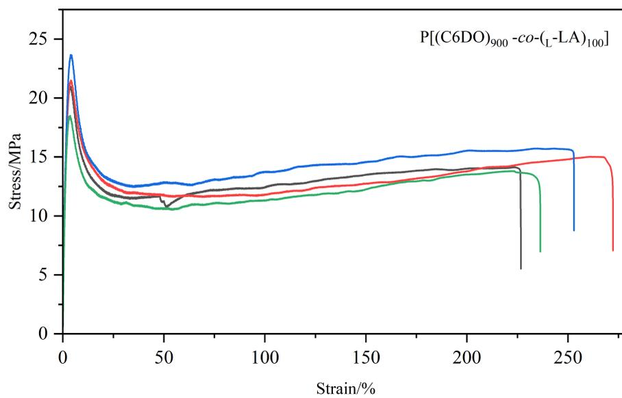
**Fig. S28.** Stress-strain curves of P[(C6DO)<sub>900</sub>-co-(L-LA)<sub>100</sub>].
