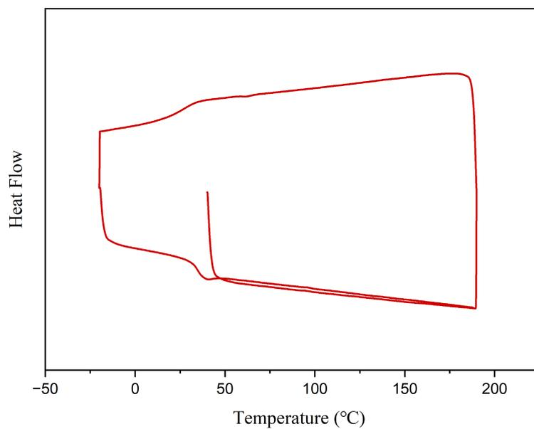
**Fig. S21.** DSC curves for P[(C6DO)<sub>900</sub>-co-(L-LA)<sub>100</sub>] obtained by [C6DO]/[L-LA]/[Zn1]/[I] = 900/100/1/1,  $T_g = 42$  °C.
