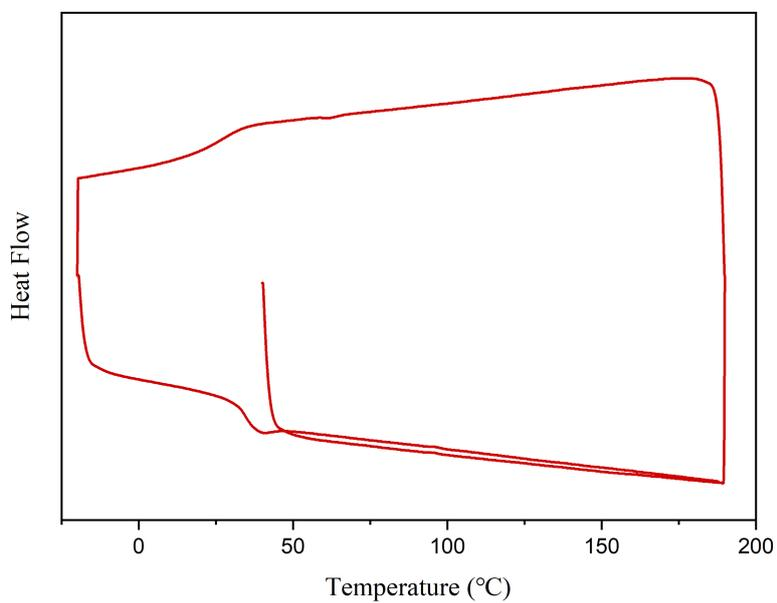
**Fig. S17** DSC curves for P(C6DO) obtained by [C6DO]/[Zn1]/[I] = 100/1/1,  $T_g = 35$  °C.
