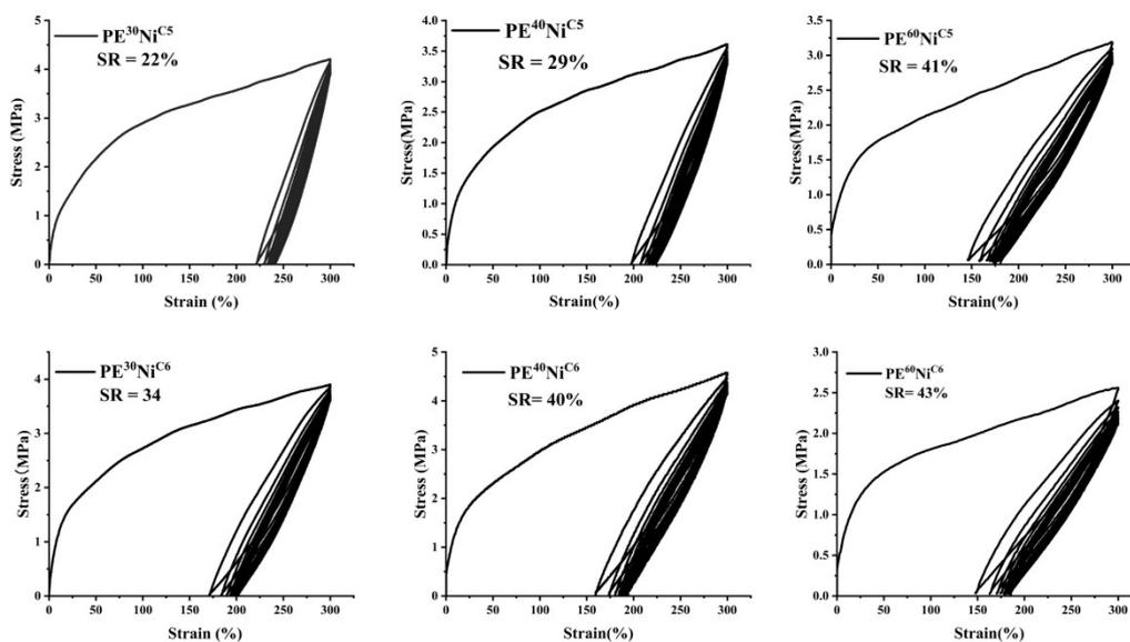
**Figure S28** Strain recovery measurements of PE samples prepared by  $\text{Ni}^{\text{C}5}$  and  $\text{Ni}^{\text{C}6}$  at  $30\text{ }^\circ\text{C}$ ,  $40\text{ }^\circ\text{C}$  and  $60\text{ }^\circ\text{C}$ .
