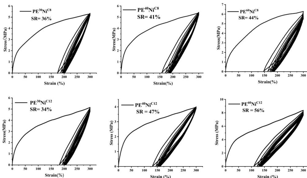
**Figure S29** Strain recovery measurements of PE samples prepared by  $\text{Ni}^{\text{C8}}$  and  $\text{Ni}^{\text{C12}}$  at 30 °C, 40 °C and 60 °C.
