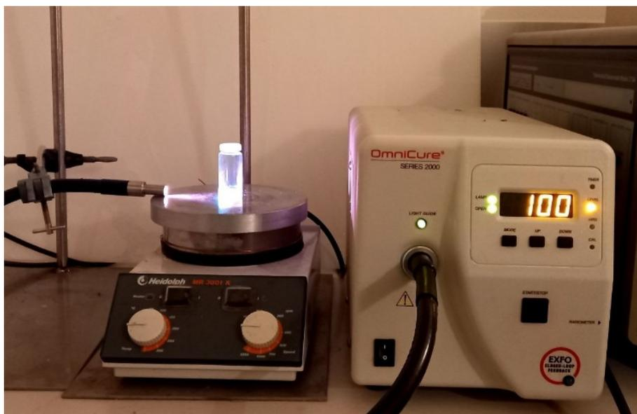
Figure S13. Photopolymerization setup using Omnicure series 2000, 200 W.
