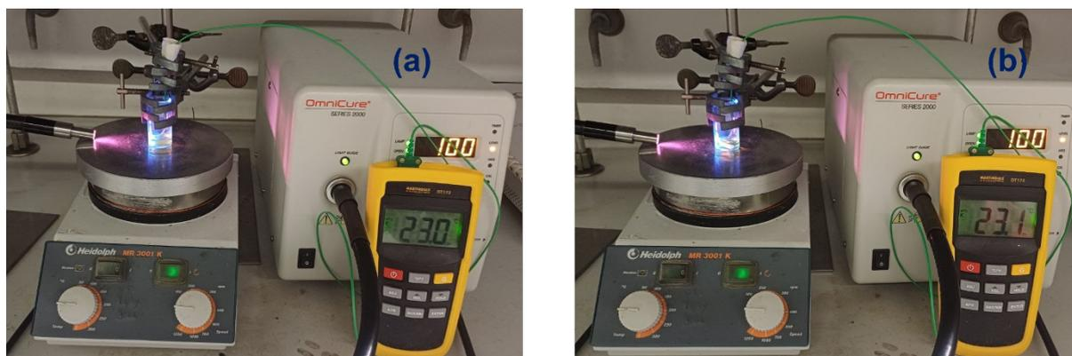
Figure S14. Photopolymerization apparatus, featuring an Omnicure series 2000, 200 W system integrated with a thermostat unit, (a) at the beginning ; (b) after 24 h of reaction
