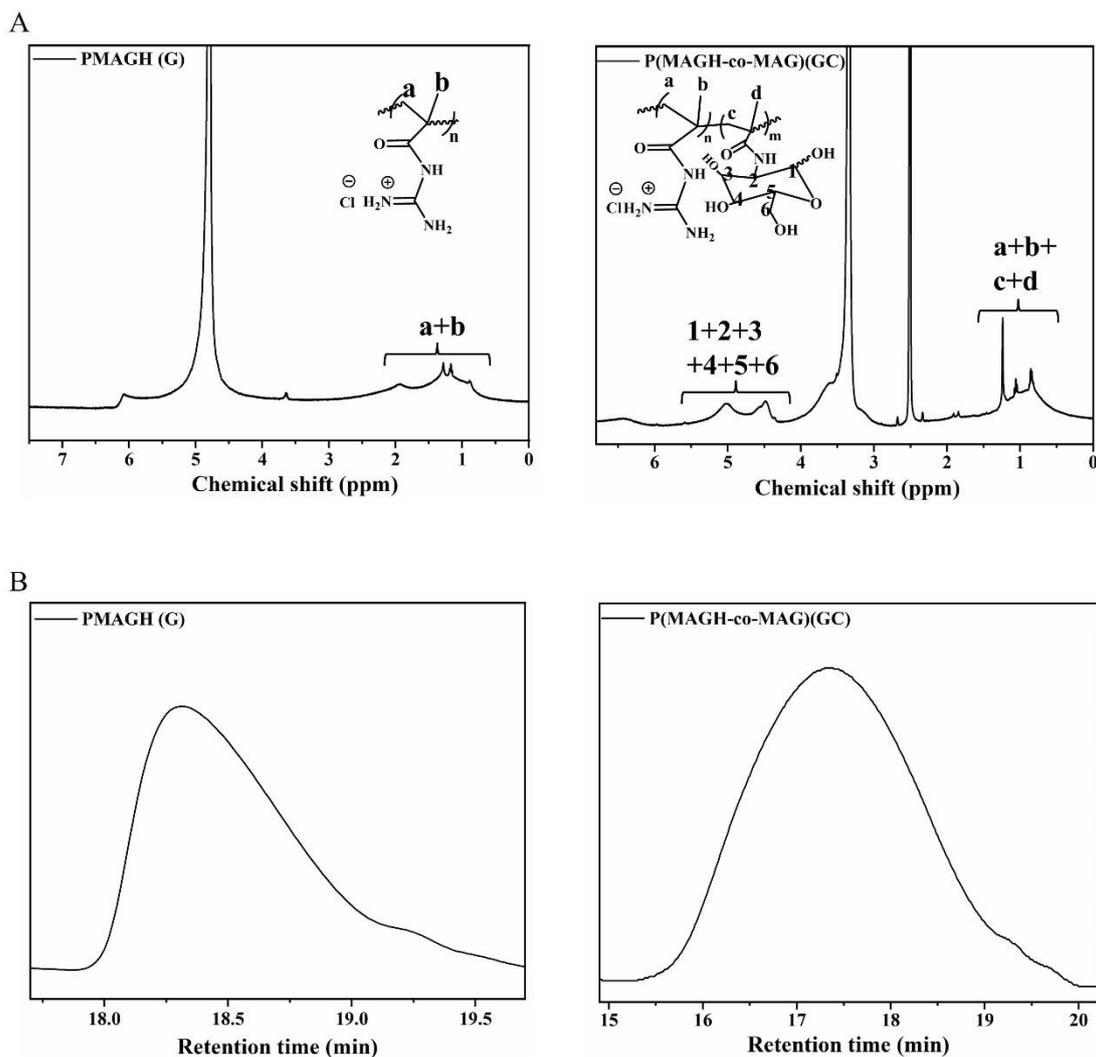
**Fig. S5.** (A)  $^1\text{H}$  NMR of PMAGH (G) in  $\text{D}_2\text{O}$  and P(MAGH-co-MAG) (GC) in  $\text{DMSO-d}_6$ . (B) SEC traces of PMAGH (G) and P(MAGH-co-MAG) (GC), Mobile phase: 0.3 mol/L sodium acetate, pH 3.0. Flow rate: 1 mL/min. Temperature: 35 °C.
