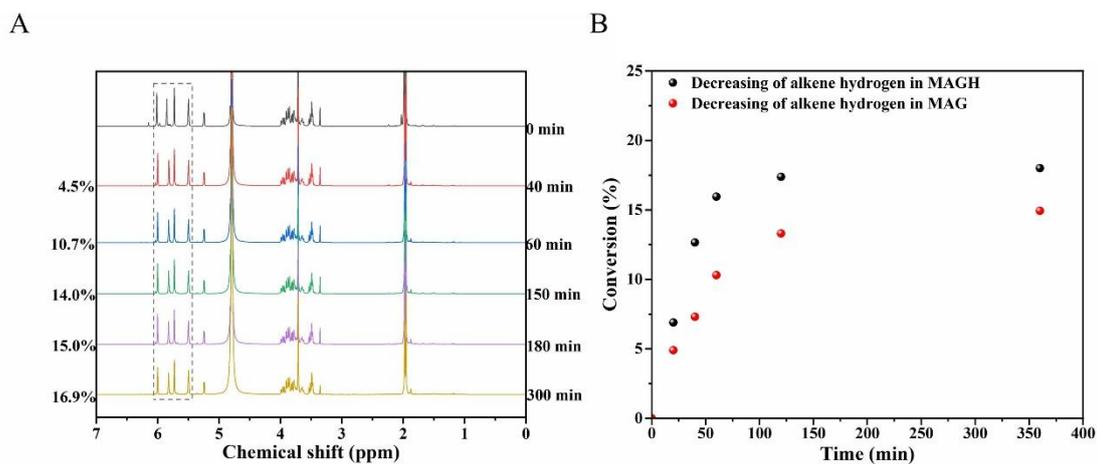
**Fig. S6.** (A) <sup>1</sup>H NMR of reaction solution for the synthesis of ZnO-GC at different polymerization time in D<sub>2</sub>O.
