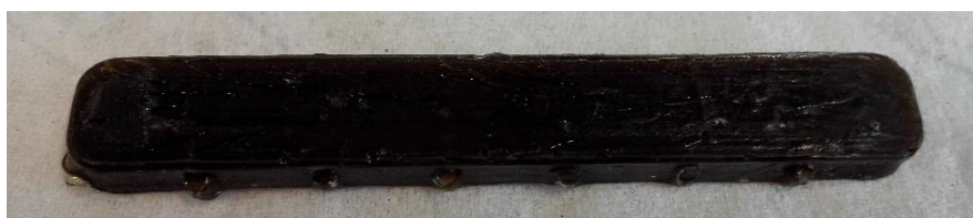
Figure S4: Picture of a cured polymer sample consisting of 1.0 mol% TTMSS, 0.5 mol% BPO, 0.1 mol% PAG and BADGE.
