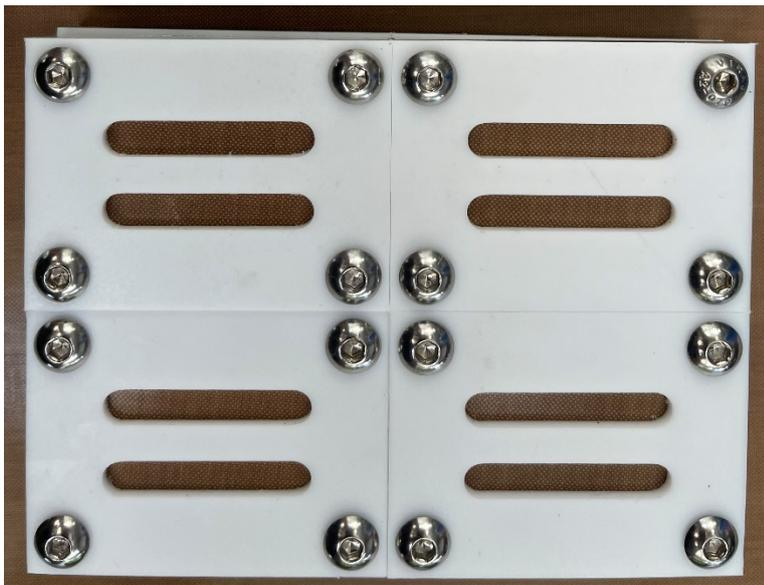
*Figure S9: Molds used for the preparation of the DMA samples.*
