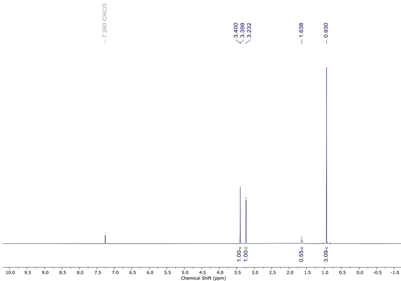
**Figure S75.**  $^1\text{H}$  NMR (600 MHz,  $\text{CDCl}_3$ , 23  $^\circ\text{C}$ ) spectrum of 3-azido-2,2-dimethyl-1-propanol (**5-OH**).
