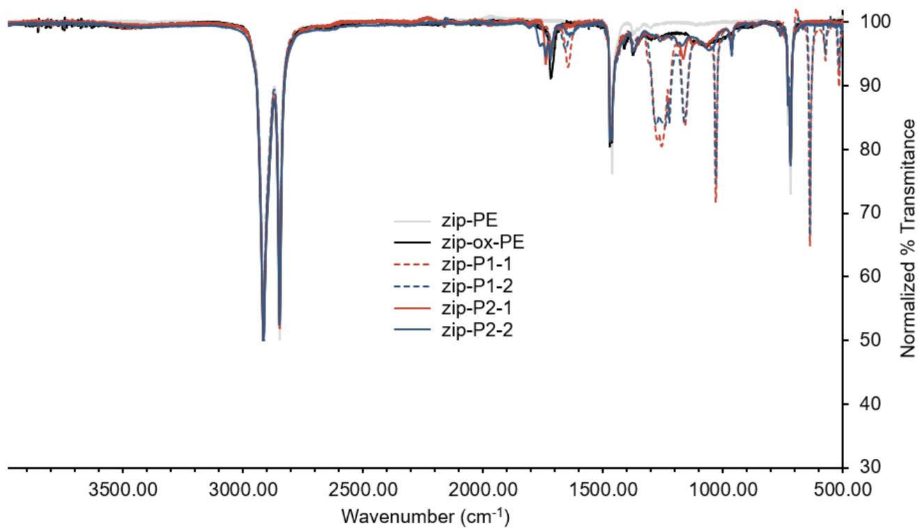
**Figure S63.** Full FTIR spectra for commercial **zip-PE**, **zip-ox-PE**, and **zip-P1** and **zip-P2** polymers sourced from commercial LDPE.
