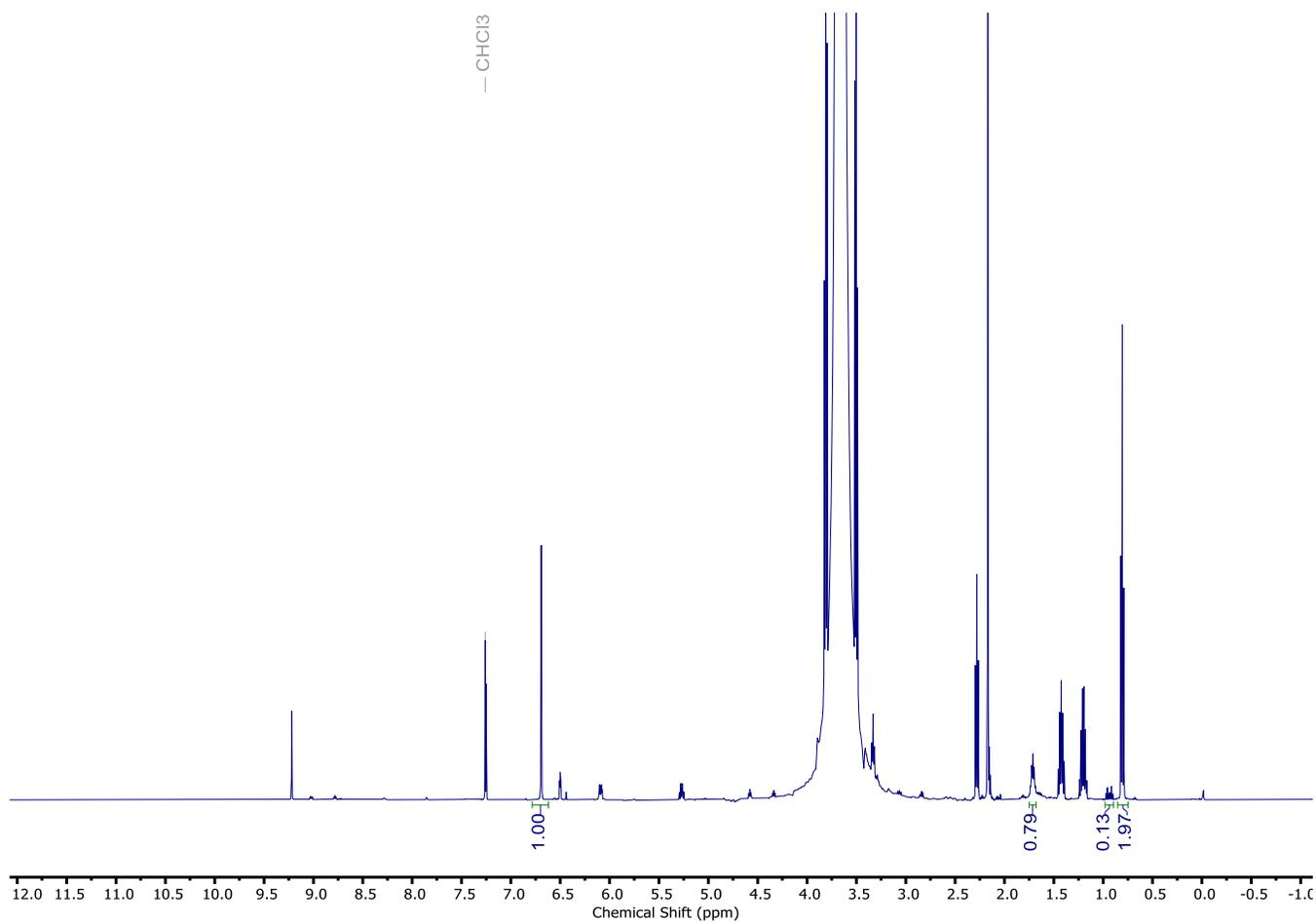
**Figure S16.**  $^1\text{H}$  NMR (500 MHz,  $\text{CDCl}_3$ , 23 °C) spectrum of aliquot of reaction of 5-nonanone with **1-OH** and tropylium tetrafluoroborate
