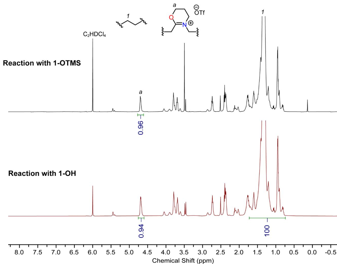
**Figure S45.**  $^1H$  NMR (500 MHz, 1,1,2,2-tetrachloroethane- $d_2$ , 90-94°C) of **P1-1** formed from reaction with **1-OH** and **1-OTMS**. The integral of the resonance from  $-CH_2-CH_2-$  repeat units ( $\sim 0.7$ – $1.7$  ppm) was set to 100 for all spectra.
