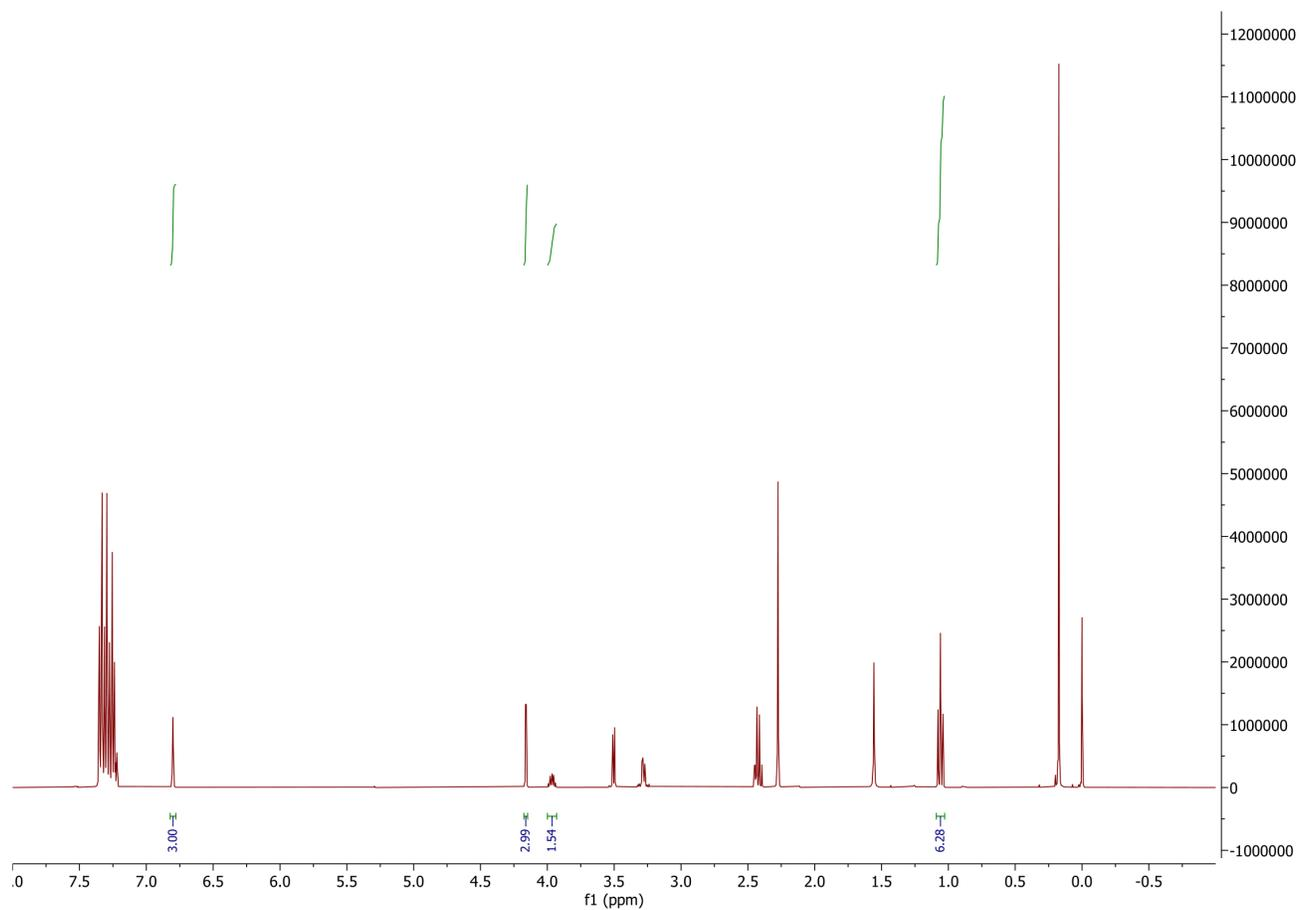
**Figure S39.**  $^1\text{H}$  NMR (400 MHz,  $\text{ACN-d}_3$ , 23  $^\circ\text{C}$ ) spectrum of stock solution of 3-pentanone, *rac*-4-OTMS, and mesitylene in chlorobenzene (900 mmolar w.r.t. 3-pentanone) used for **Table 1 entry 13**.
