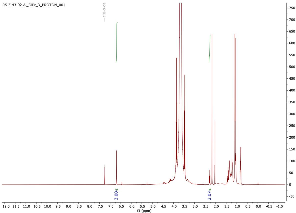
**Figure S20.**  $^1\text{H}$  NMR (400 MHz,  $\text{CDCl}_3$ , 23  $^\circ\text{C}$ ) spectrum of aliquot of reaction of 5-nonanone with **1-OH** and  $\text{Al}(\text{O}^i\text{Pr})_3$
