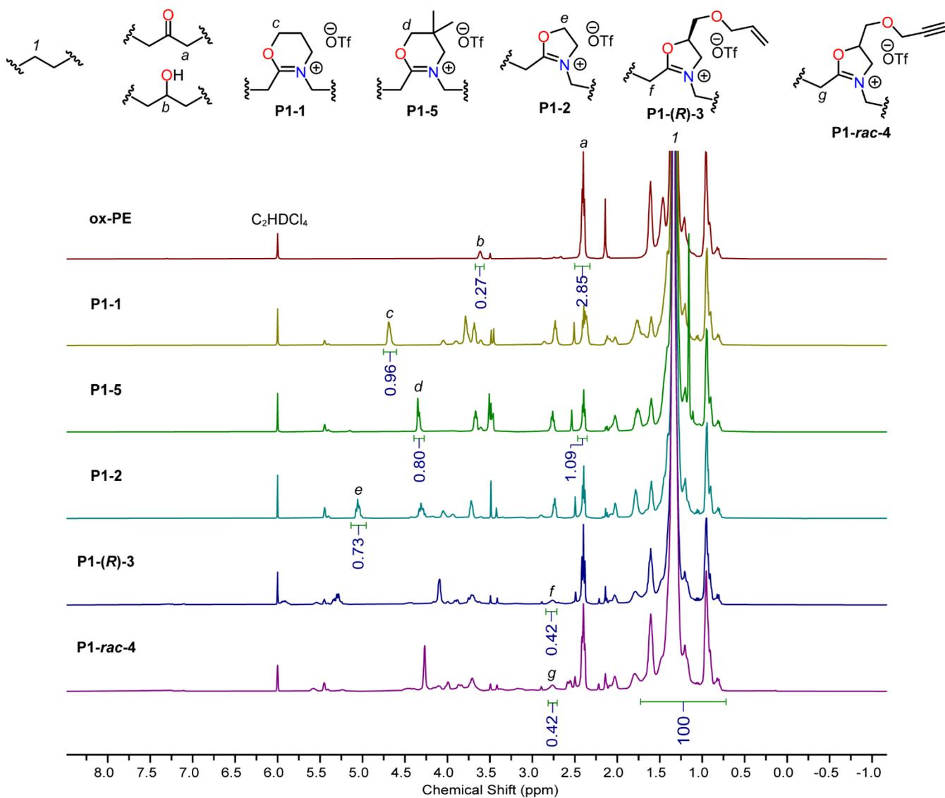
**Figure S31.**  $^1\text{H}$  NMR (400 or 500 MHz, 1,1,2,2-tetrachloroethane- $d_2$ , 90-94 °C) of ox-PE and P1 series (Table 1, entries 9, 14–17). The integral of the resonance from  $-\text{CH}_2-\text{CH}_2-$  repeat units ( $\sim 0.7$ – $1.7$  ppm) was set to 100 for all spectra.
