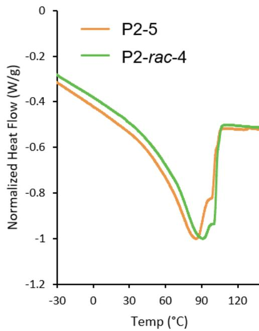
**Figure S61.** DSC traces for **P2-5** and **P2-rac-4**.
