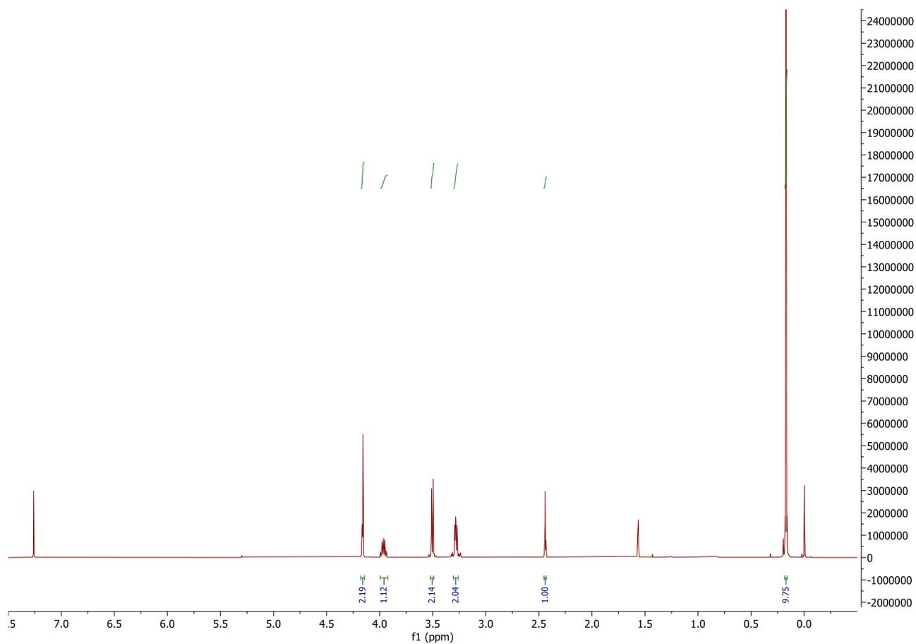
**Figure S86.** <sup>1</sup>H NMR (400 MHz, CDCl<sub>3</sub>, 23 °C) spectrum of ((1-azido-3-(prop-2-yn-1-yloxy)propan-2-yl)oxy)trimethylsilane (*rac*-4-OTMS)
