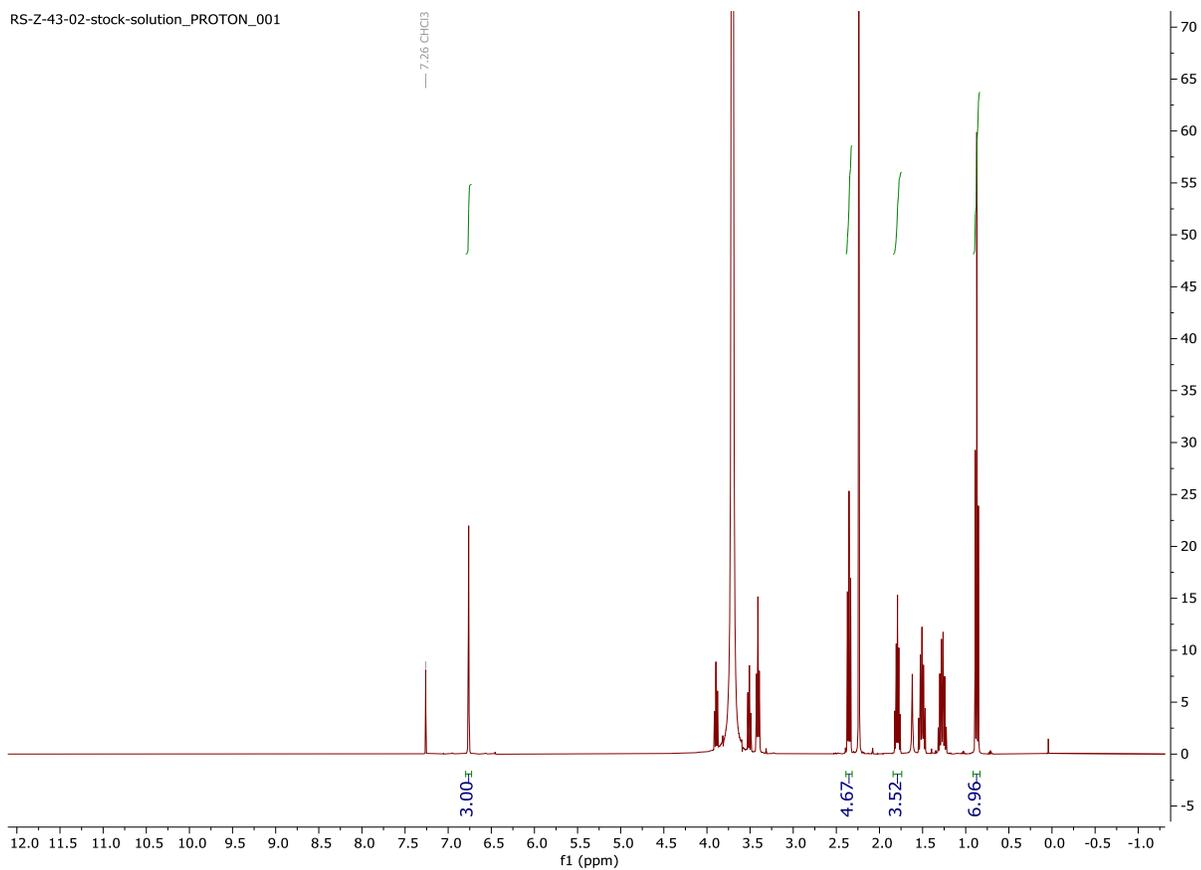
**Figure S18.** <sup>1</sup>H NMR (400 MHz, CDCl<sub>3</sub>, 23 °C) spectrum of stock solution of 5-nonanone, **1-OH**, and mesitylene in DCE for reactions with BiCl<sub>3</sub>, Al(O<sup>i</sup>Pr)<sub>3</sub>, AlCl<sub>3</sub>, Bi(OTf)<sub>3</sub>, and Sc(OTf)<sub>3</sub>.
