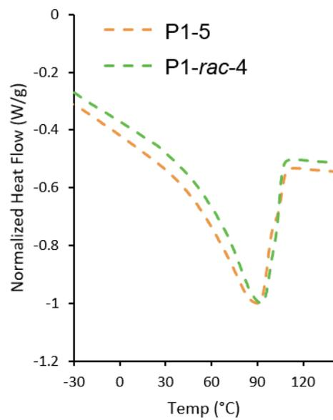
**Figure S48.** DSC traces for **P1-5** and **P1-rac-4**.
