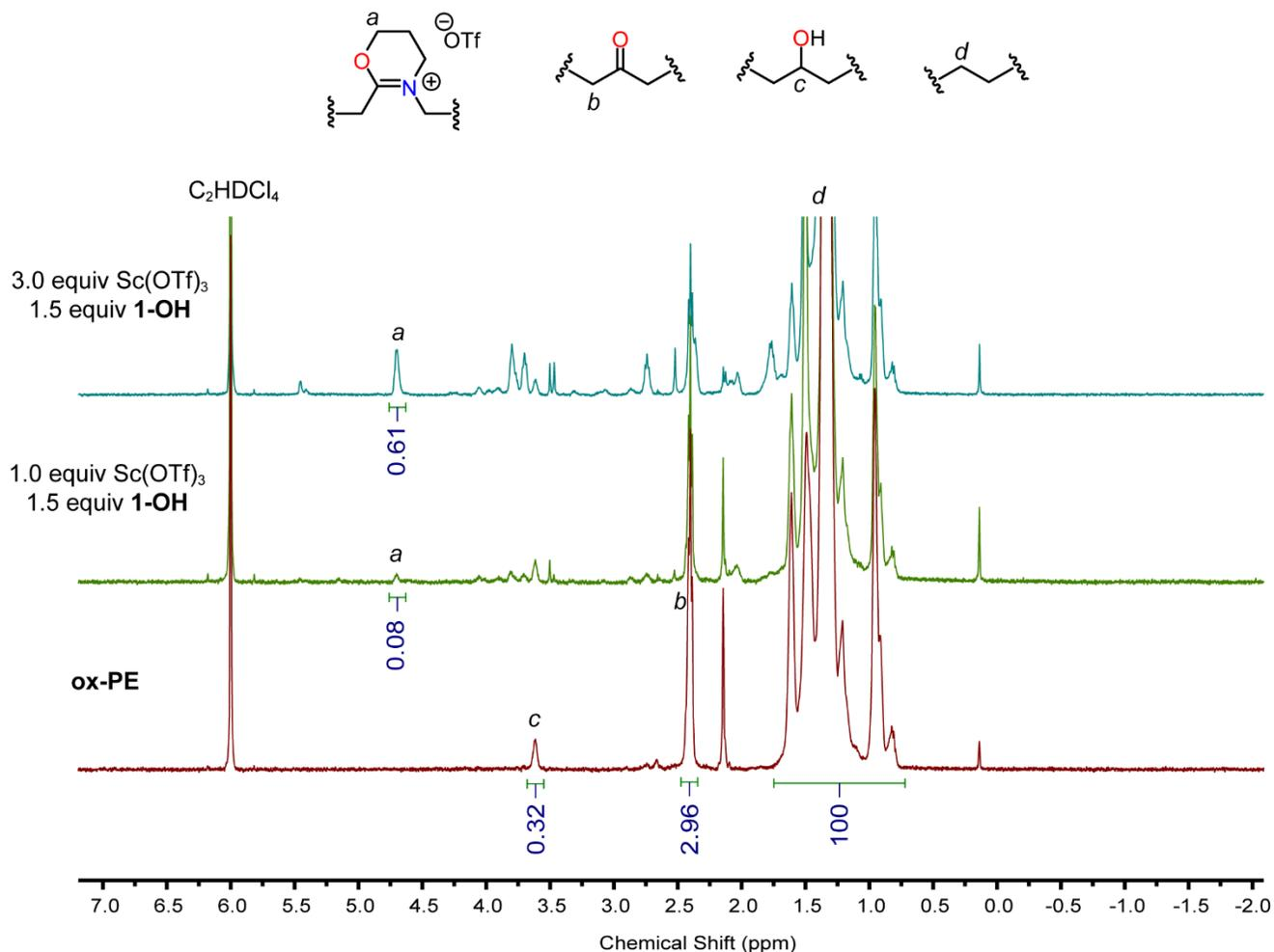
**Figure S29.**  $^1H$  NMR (500 MHz, 1,1,2,2-tetrachloroethane- $d_2$ , 92-94 °C) of **ox-PE** and products of reactions of **ox-PE** with 1.5 equiv **1-OH** and varying equivalents of  $Sc(OTf)_3$  (Table 1, entries 5–6). The integral of the resonance from  $-CH_2-CH_2-$  repeat units ( $\sim 0.7-1.7$  ppm) was set to 100 for all spectra.
