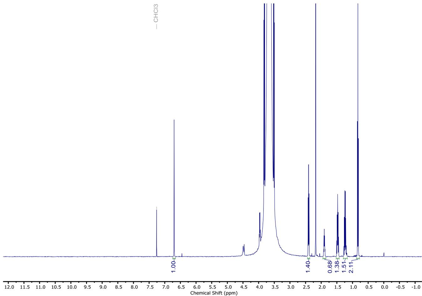
**Figure S11.** <sup>1</sup>H NMR (500 MHz, CDCl<sub>3</sub>, 23 °C) spectrum of aliquot of reaction of 5-nonanone with **1-OH** and Mg(ClO<sub>4</sub>)<sub>2</sub>
