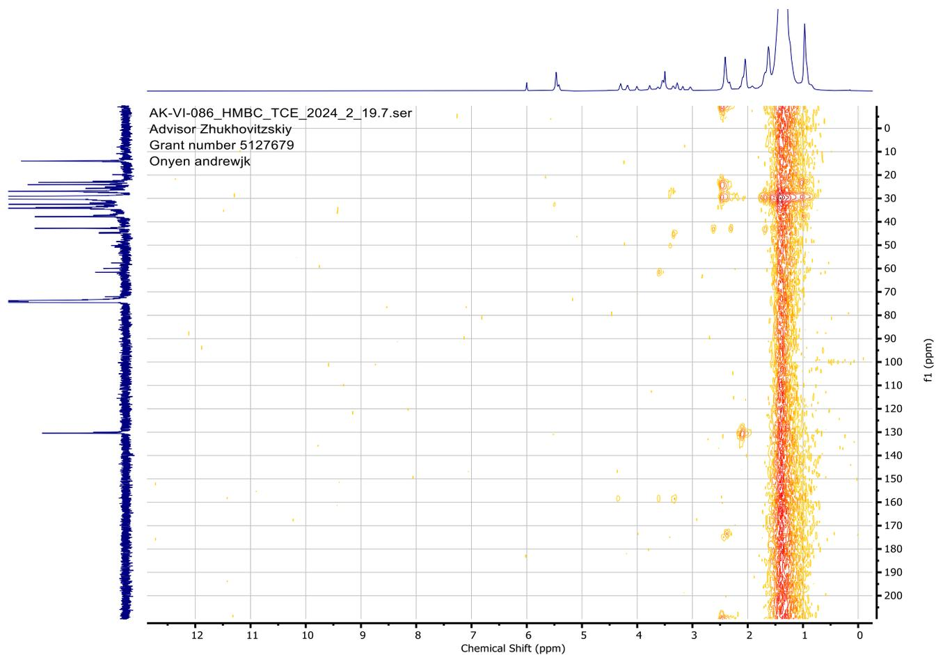
**Figure S68.**  $^1\text{H}-^{13}\text{C}\{^1\text{H}\}$  HMBC NMR (1,1,2,2-tetrachloroethane- $d_2$ , 111 °C) spectrum of **zip-P2-2** sourced from LDPE
