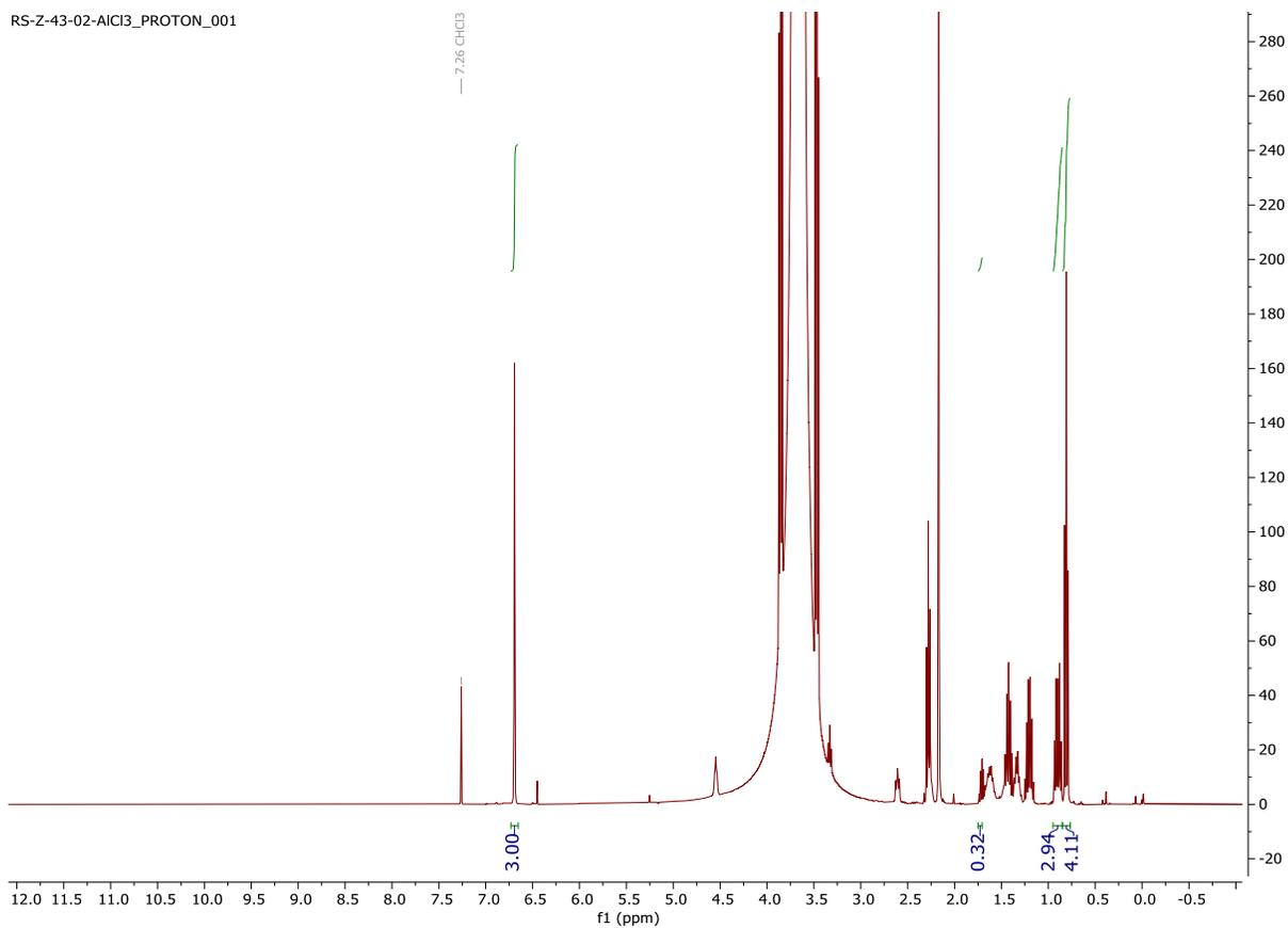
**Figure S21.**  $^1\text{H}$  NMR (400 MHz,  $\text{CDCl}_3$ , 23  $^\circ\text{C}$ ) spectrum of aliquot of reaction of 5-nonanone with **1-OH** and  $\text{AlCl}_3$
