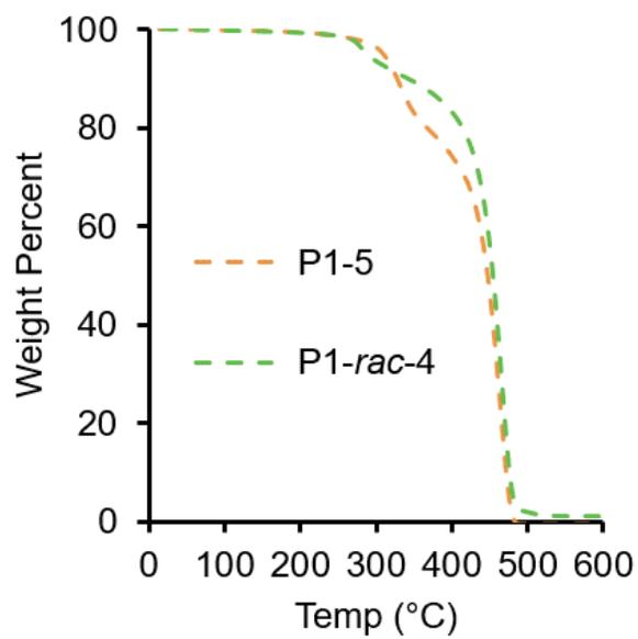
**Figure S49.** TGA traces for **P1-5** and **P1-rac-4**.
