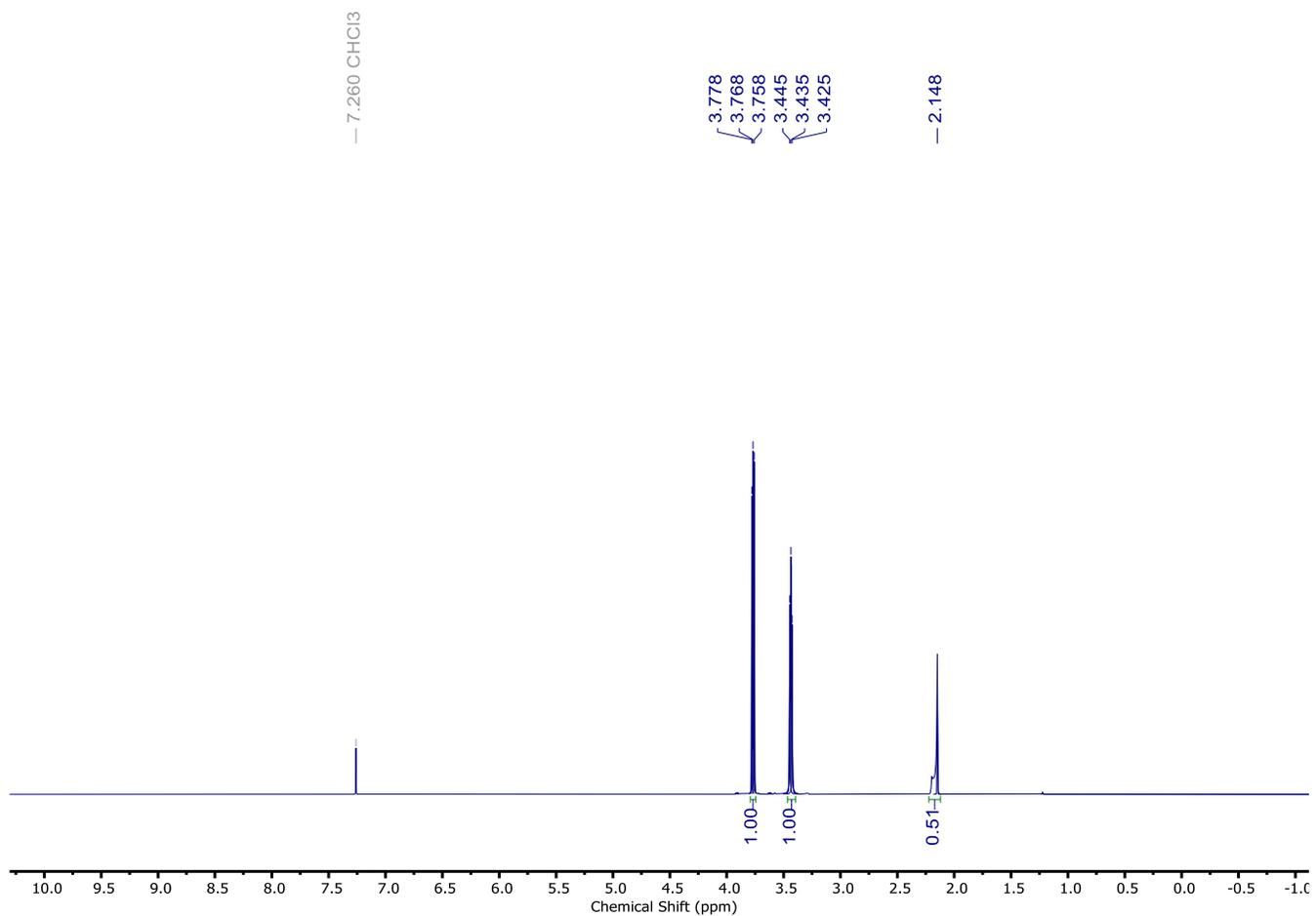
**Figure S76.** <sup>1</sup>H NMR (500 MHz, CDCl<sub>3</sub>, 23 °C) spectrum of 2-azido-1-propanol (**2-OH**).
