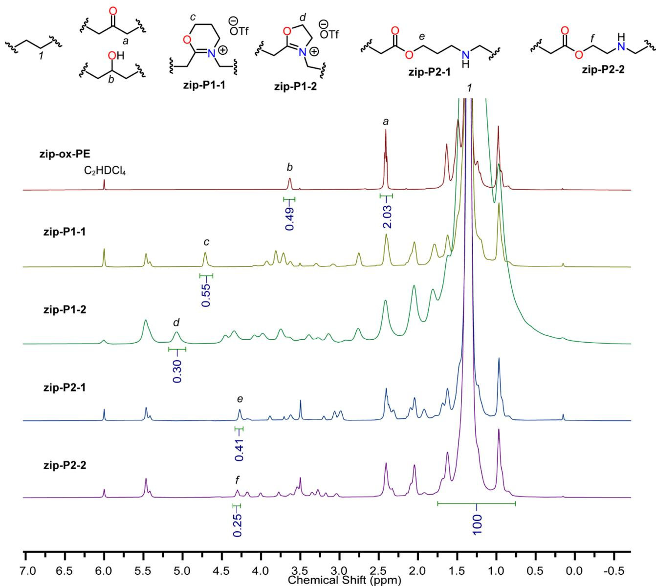
**Figure S64.**  $^1\text{H}$  NMR (400 or 500 MHz, 1,1,2,2-tetrachloroethane- $d_2$ , 111–118  $^\circ\text{C}$ ) of **zip-ox-PE**, **zip-P1-1**, **zip-P1-2**, **zip-P2-1**, and **zip-P2-2** (sourced from LDPE). The integral of the resonance from  $-\text{CH}_2-\text{CH}_2-$  repeat units ( $\sim 0.7$ – $1.7$  ppm) was set to 100 for all spectra.
