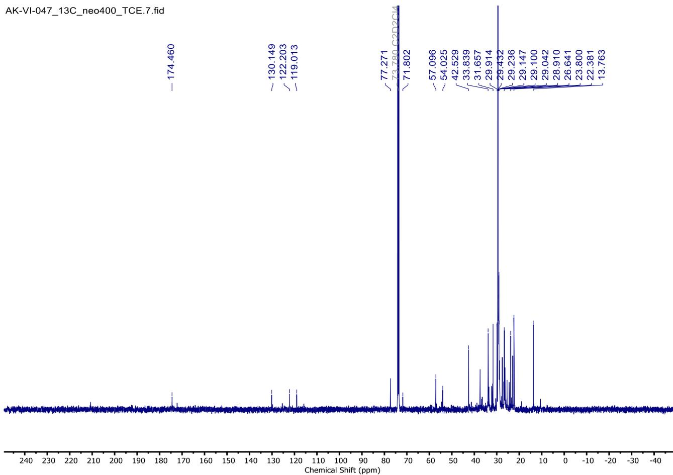
**Figure S44.**  $^{13}\text{C}$  NMR (101 MHz, 1,1,2,2-tetrachloroethane- $\text{d}_2$ ,  $\sim 90^\circ\text{C}$ ) of **P1-5**
