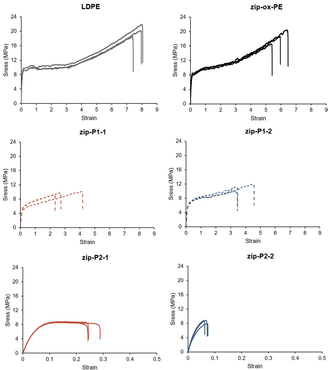
**Figure S69.** Triplicate uniaxial tensile tests for materials sourced from commercial **LDPE** (Note: strain axis has different scale for **zip-P2-1** and **zip-P2-2** to allow for better visualization of the data).
