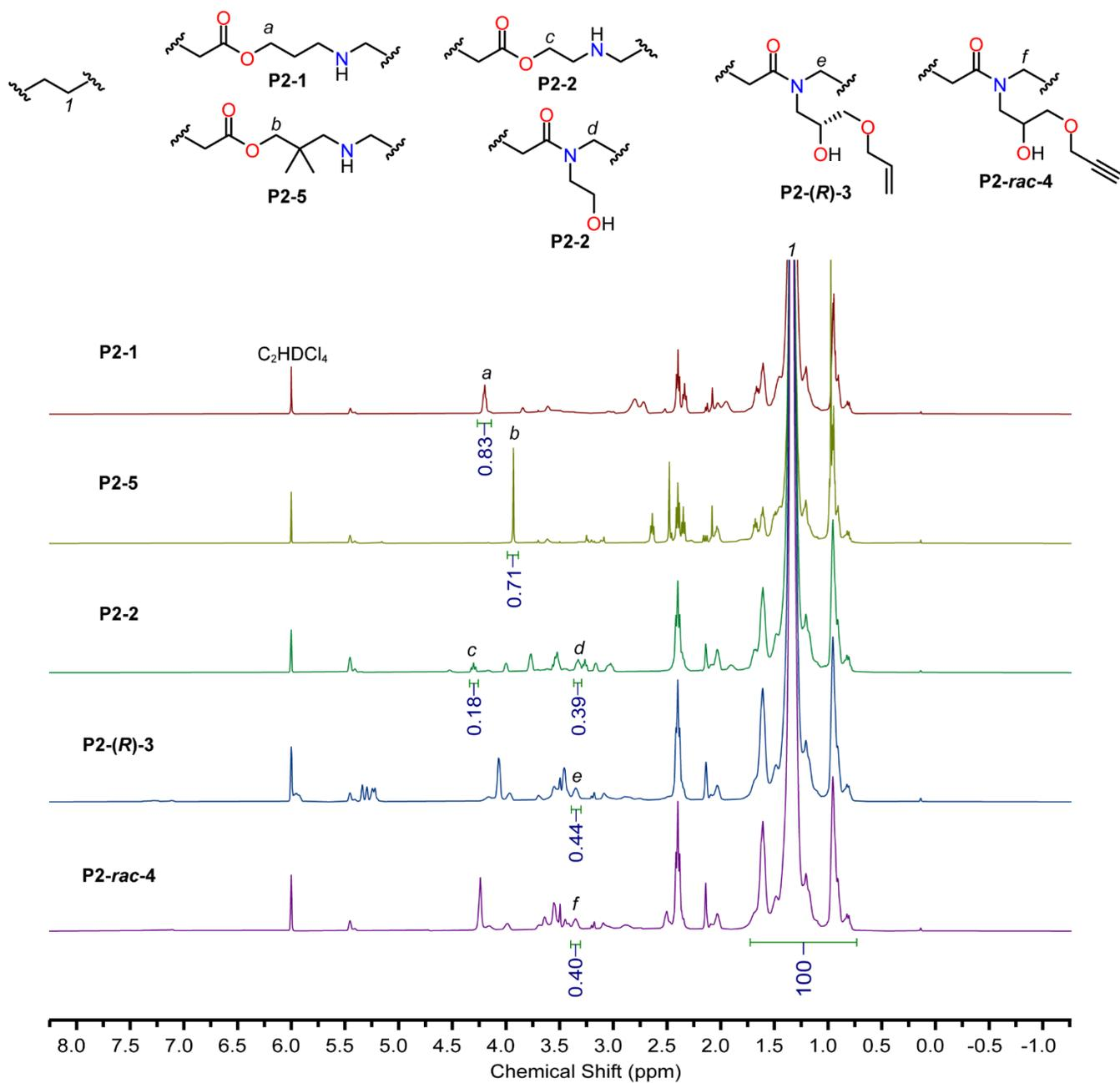
**Figure S53.**  $^1\text{H}$  NMR (400 or 500 MHz, 1,1,2,2-tetrachloroethane- $\text{d}_2$ , 90-94  $^\circ\text{C}$ ) of ox-PE and P2 series. The integral of the resonance from  $-\text{CH}_2-\text{CH}_2-$  repeat units ( $\sim 0.7-1.7$  ppm) was set to 100 for all spectra.
