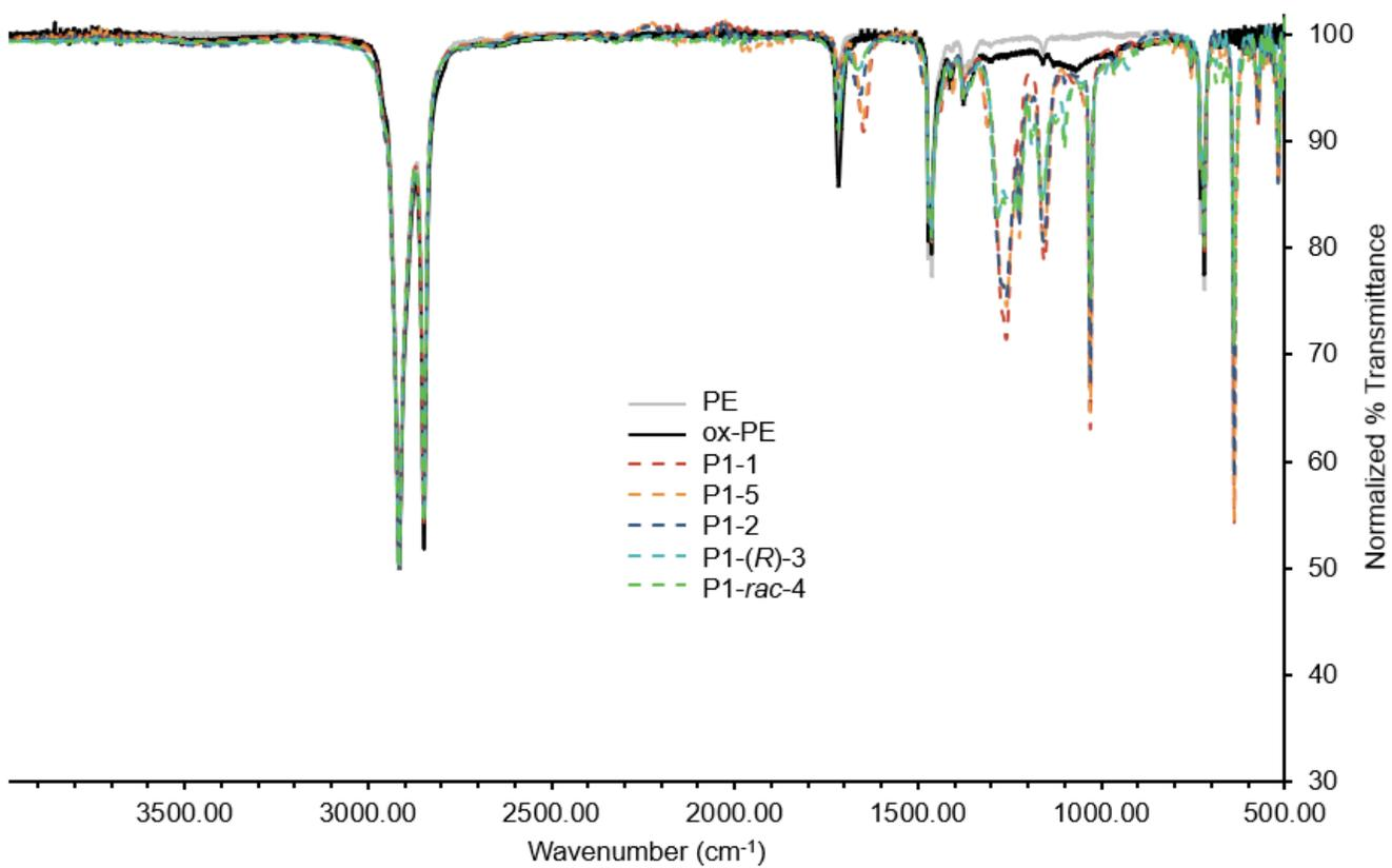
**Figure S46.** Full FTIR spectra for **PE**, **ox-PE**, and the **P1** series sourced from PE with  $M_n = 1.7$  kg/mol.
