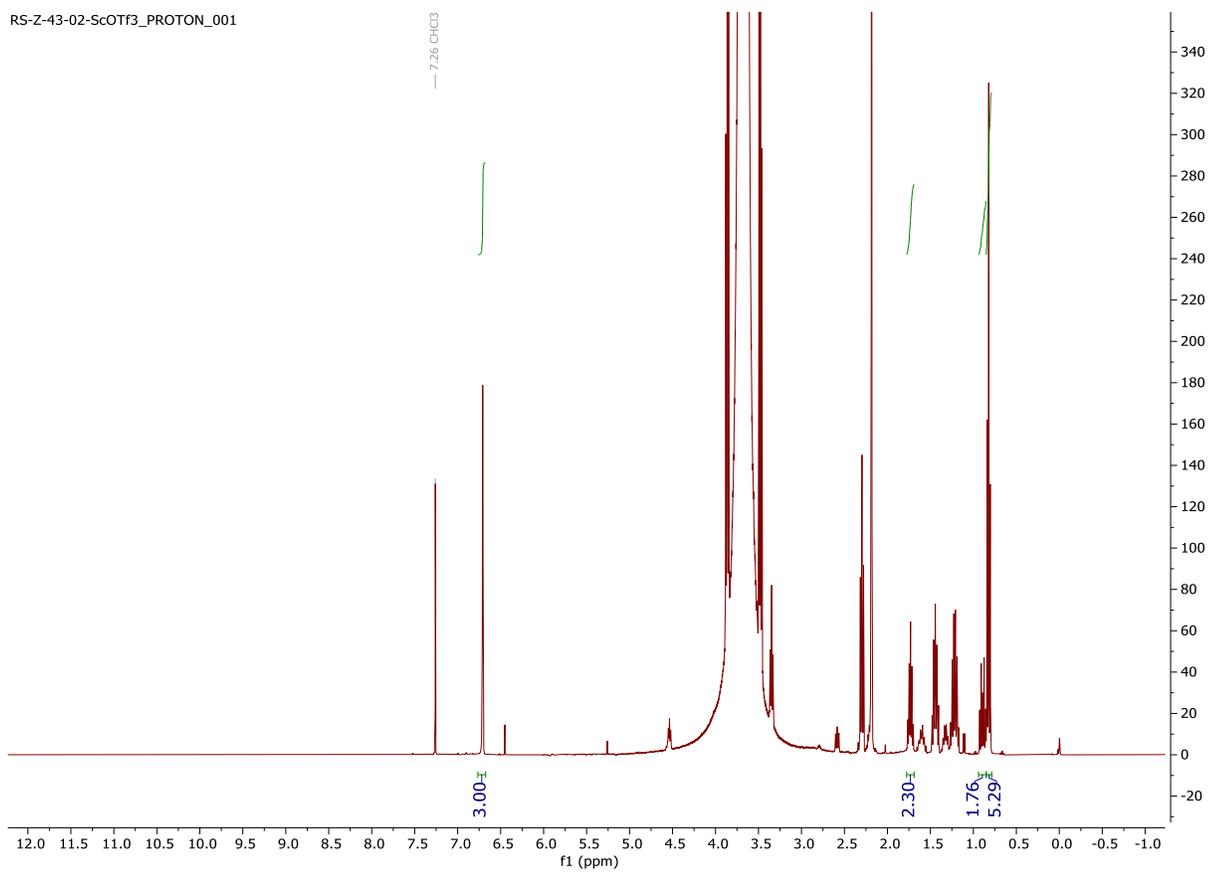
**Figure S23.**  $^1\text{H}$  NMR (400 MHz,  $\text{CDCl}_3$ , 23  $^\circ\text{C}$ ) spectrum of aliquot of reaction of 5-nonanone with **1-OH** and  $\text{Sc}(\text{OTf})_3$
