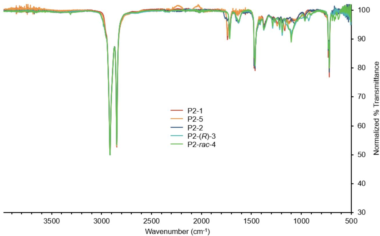
**Figure S51.** Full FTIR spectra for the **P2** series sourced from PE with  $M_n = 1.7$  kg/mol.
