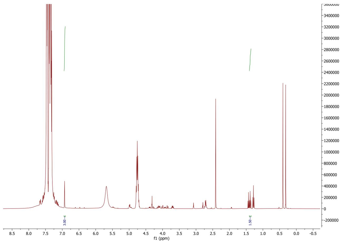
**Replicate 3 Figure S40.** <sup>1</sup>H NMR (400 MHz, ACN-d<sub>3</sub>, 23 °C) spectra for triplicate results described in **Table 1 entry 13**. Yield is calculated from integration of methyl resonance of product iminium ether at ~1.3 ppm. Yield from each replicate (tabulated in **Table S2**) is averaged. The average is tabulated in **Table 1**.
