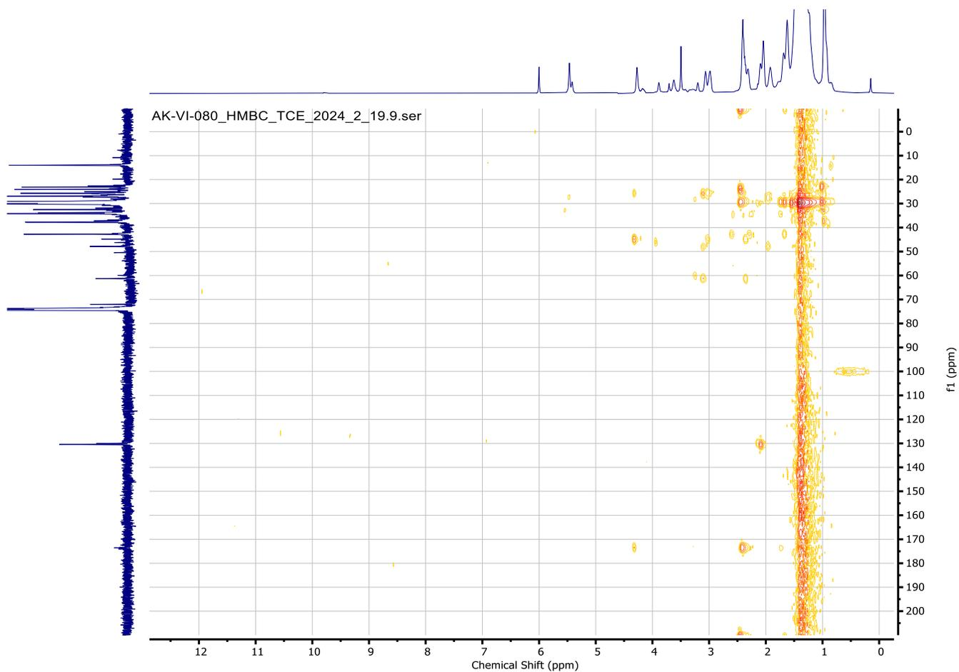
**Figure S67.**  $^1\text{H}$ - $^{13}\text{C}\{^1\text{H}\}$  HMBC NMR (1,1,2,2-tetrachloroethane- $d_2$ , 111 °C) spectrum of **zip-P2-1** sourced from LDPE
