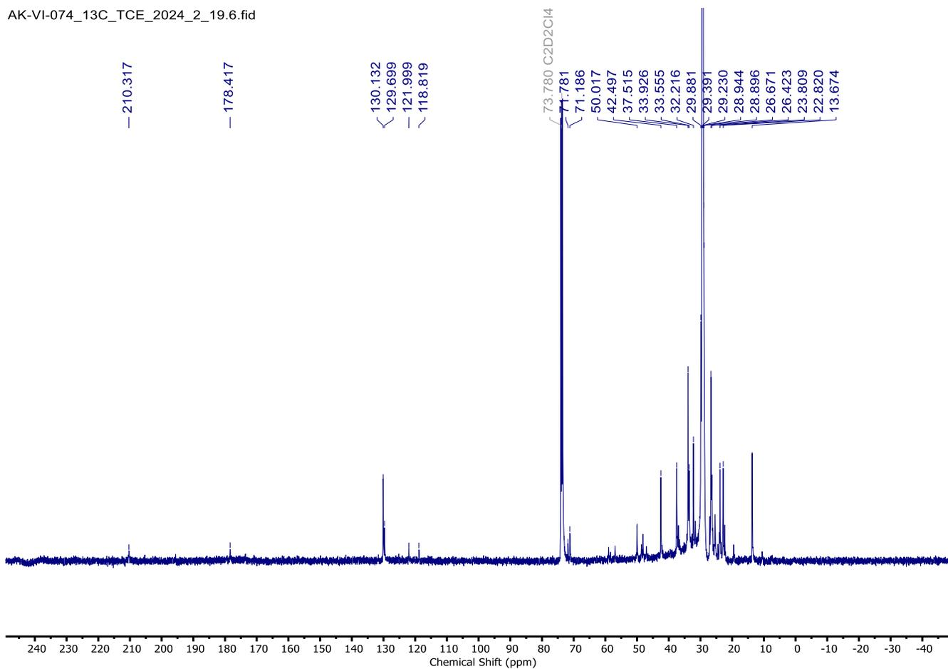
**Figure S66.**  $^{13}\text{C}$  NMR (101 MHz, 1,1,2,2-tetrachloroethane- $d_2$ , 111  $^{\circ}\text{C}$ ) of **zip-P1-2** sourced from LDPE.
