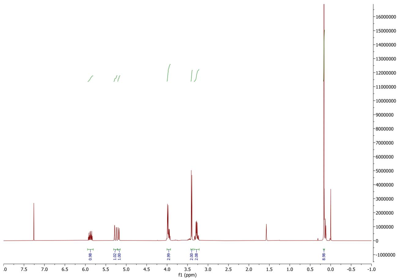
**Figure S77.**  $^1\text{H}$  NMR (400 MHz,  $\text{CDCl}_3$ , 23  $^\circ\text{C}$ ) spectrum of (S)-((1-(allyloxy)-3-azidopropan-2-yl)oxy)trimethylsilane ((S)-3-OTMS)
