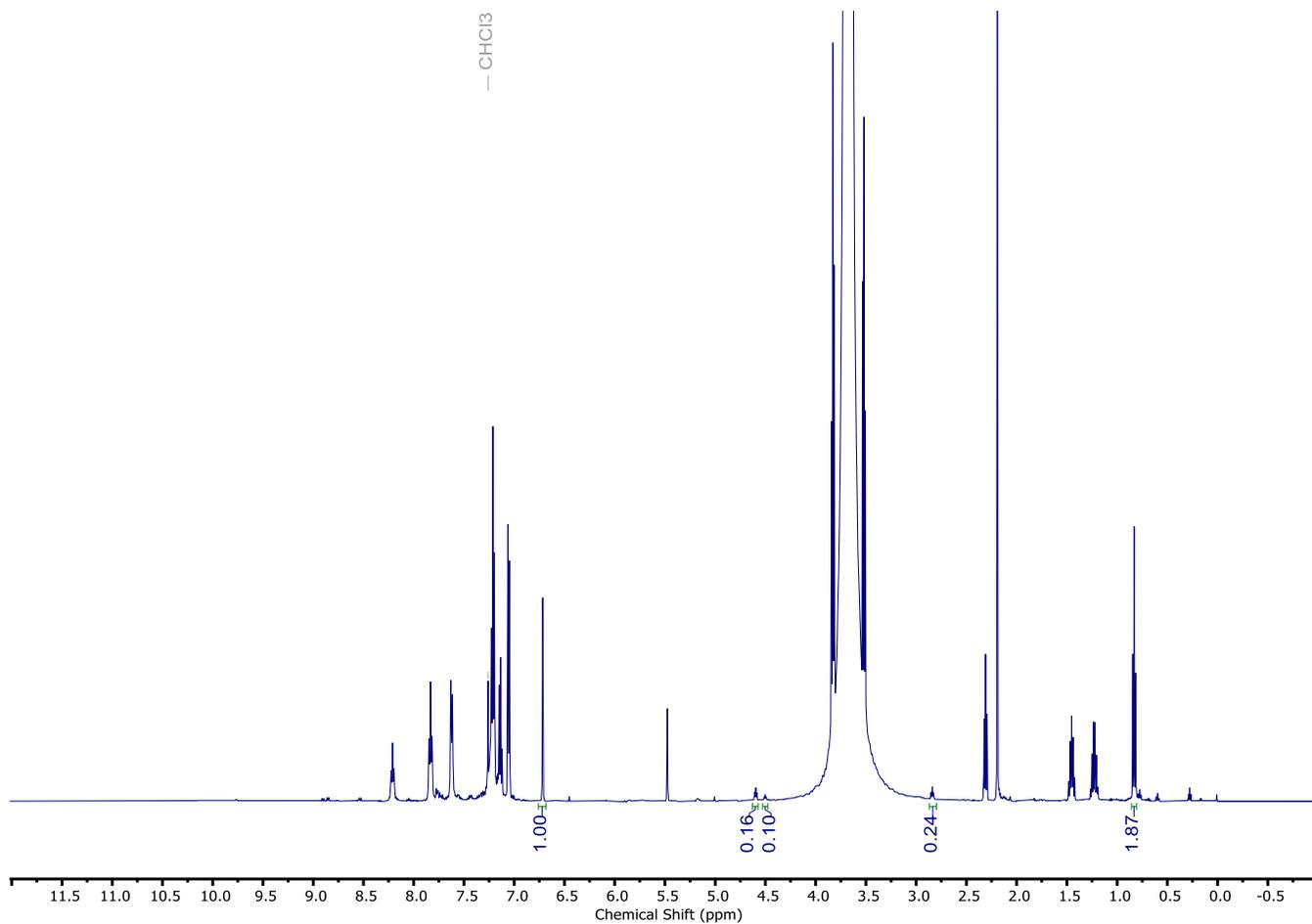
**Figure S17.**  $^1\text{H}$  NMR (500 MHz,  $\text{CDCl}_3$ , 23  $^\circ\text{C}$ ) spectrum of aliquot of reaction of 5-nonanone with **1-OH** and tritylium tetrafluoroborate
