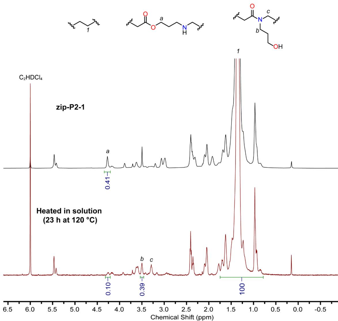
**Figure S72.**  $^1\text{H}$  NMR (500 MHz, 1,1,2,2-tetrachloroethane- $\text{d}_2$ , 112 °C) of **zip-P2-1** (sourced from LDPE) and isomerized **zip-P2-1**. The integral of the resonance from  $-\text{CH}_2-\text{CH}_2-$  repeat units ( $\sim 0.7\text{--}1.7$  ppm) was set to 100 for all spectra.
