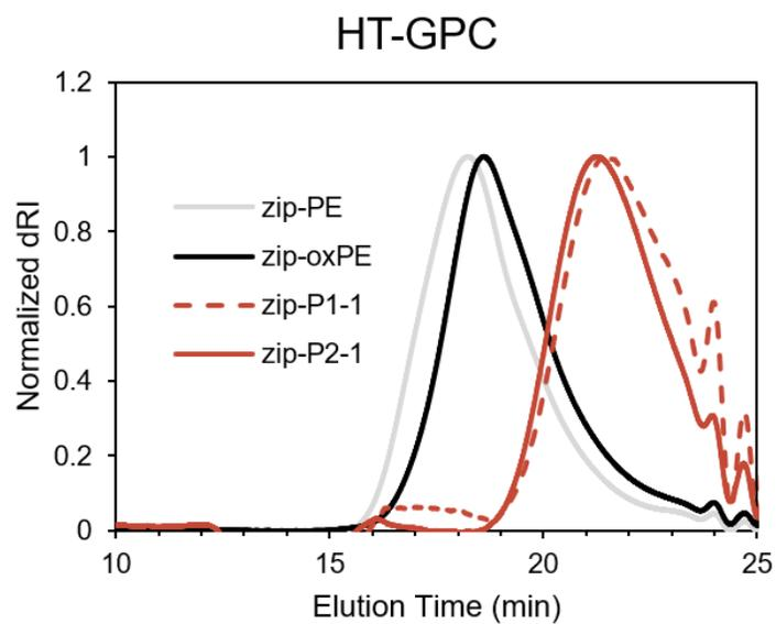
**Figure S70.** HT-GPC (140 °C, 1,2,4-trichlorobenzene) traces for **zip-PE**, **zip-ox-PE**, **zip-P1-1**, and **zip-P2-1**.
