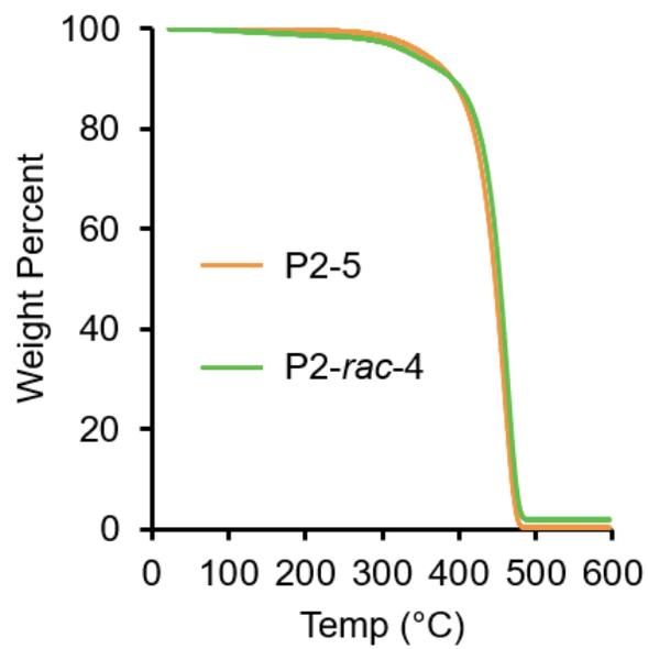
**Figure S62.** TGA traces for **P2-5** and **P2-rac-4**.
