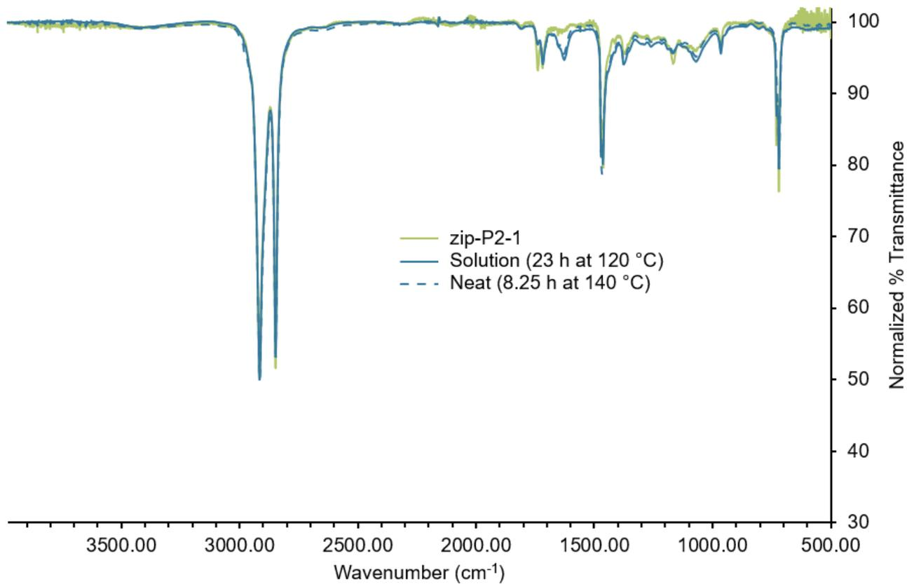
**Figure S71.** Full FTIR spectra for **zip-P2-1** and products of isomerization.
