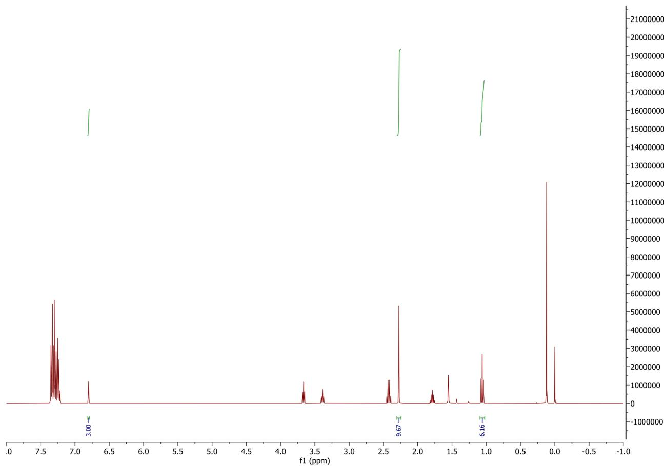
**Figure S33.** <sup>1</sup>H NMR (400 MHz, CDCl<sub>3</sub>, 23 °C) spectrum of stock solution of 3-pentanone, 1-OTMS, and mesitylene in chlorobenzene (900 mmolar w.r.t. 3-pentanone) used for **Table 1 entry 10**.
