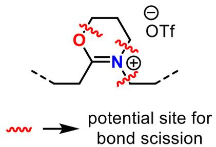
**Figure S50.** Hypothesized sites for thermal chain-cleavage in iminium ether containing polymers during TGA analysis. Structure shown is from **P1-1**
