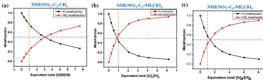
**Figure S7:** The quality of fitting and change in the mole fraction of free polymer to the complexed fraction with an increasing amount of added external folding agent obtained from NMR titration experiments.
