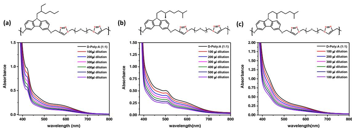
**Figure S8:** Variation of CT band intensity of different polymers upon serial dilution with acceptor folding agent,  $NMI(NO_2)_2-C_3-NH_3^+ClO_4^-$ . The measurements were performed in a mixture of  $CHCl_3:CH_3CN$  (1:2) solvents.
