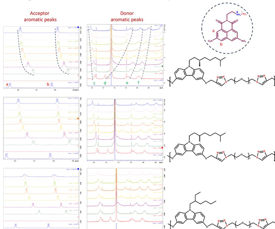
**Figure S3:** Variation in the aromatic region of the  $^1\text{H}$ -NMR spectra of the polymer as a function of increasing amount of acceptor containing folding agent,  $\text{NMI}(\text{NO}_2)_2\text{-C}_2\text{-NH}_3^+\text{ClO}_4^-$ . The measurements were performed in a mixture of  $\text{CDCl}_3:\text{CH}_3\text{CN}$  (1:2) solvent.
