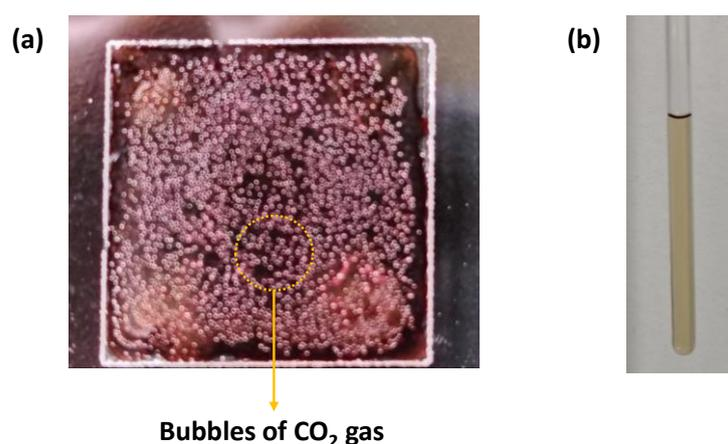
**Figure S10:** (a) The effervescence of  $CO_2$  gas, due to neutralization of ammonium functional group with aqueous  $NaHCO_3$  solution. (b) Brownish colour solution obtained by dissolving the merlot colour film in  $CDCl_3$  and  $CH_3CN$  (1:2) solvent mixture.
