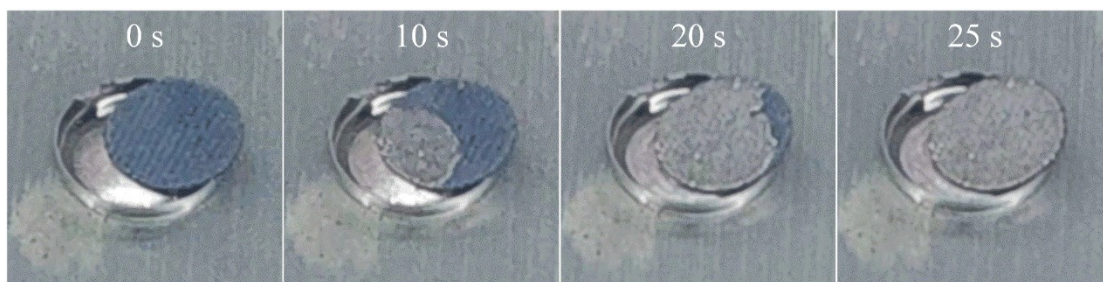
Fig. S6 Photographs of the evolution of ZnO/CC to Li@ZnO/CC composite through thermal infusion process of molten Li.
