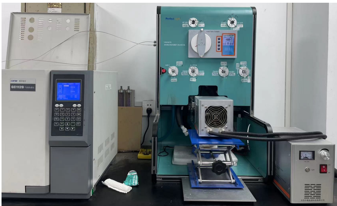
Fig. S11 Photocatalysis equipment picture for the photocatalytic hydrogen evolution test.
