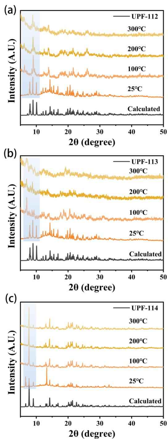
**Figure S12.** Ex-situ variable temperature powder X-ray diffraction (VT-PXRD) patterns of (a) UPF-112, (b) UPF-113, and (c) UPF-114 taken with a Cu K $\alpha$  radiation source.
