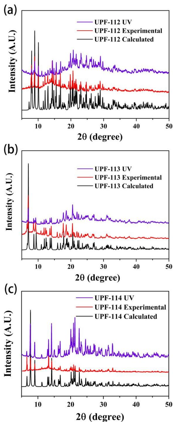
**Figure S11.** Powder X-ray diffraction (PXRD) patterns of calculated (black), experimental (red) and UV irradiated (violet) for **UPF-112**, **UPF-113** and **UPF-114**.
