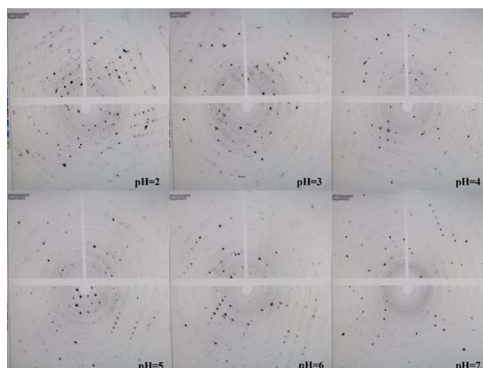
Figure S20. X-ray single crystal diffraction points of AIOC-136 after soaking in the aqueous solution over a pH range of 2-7 for 48 h.
