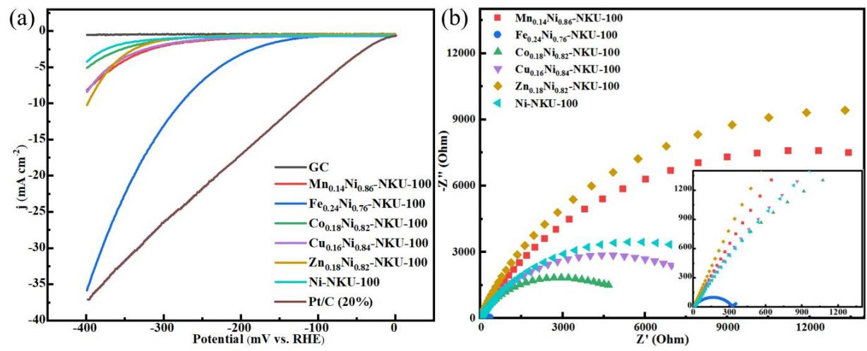
**Fig. S13** (a) LSV curves at a scan rate of 5 mV·s<sup>-1</sup> and (b) EIS Nyquist plots of M<sub>x</sub>Ni<sub>1-x</sub>-NKU-100 (M = Mn, Fe, Co, Cu, Zn) in 1 M NaOH electrolyte.
