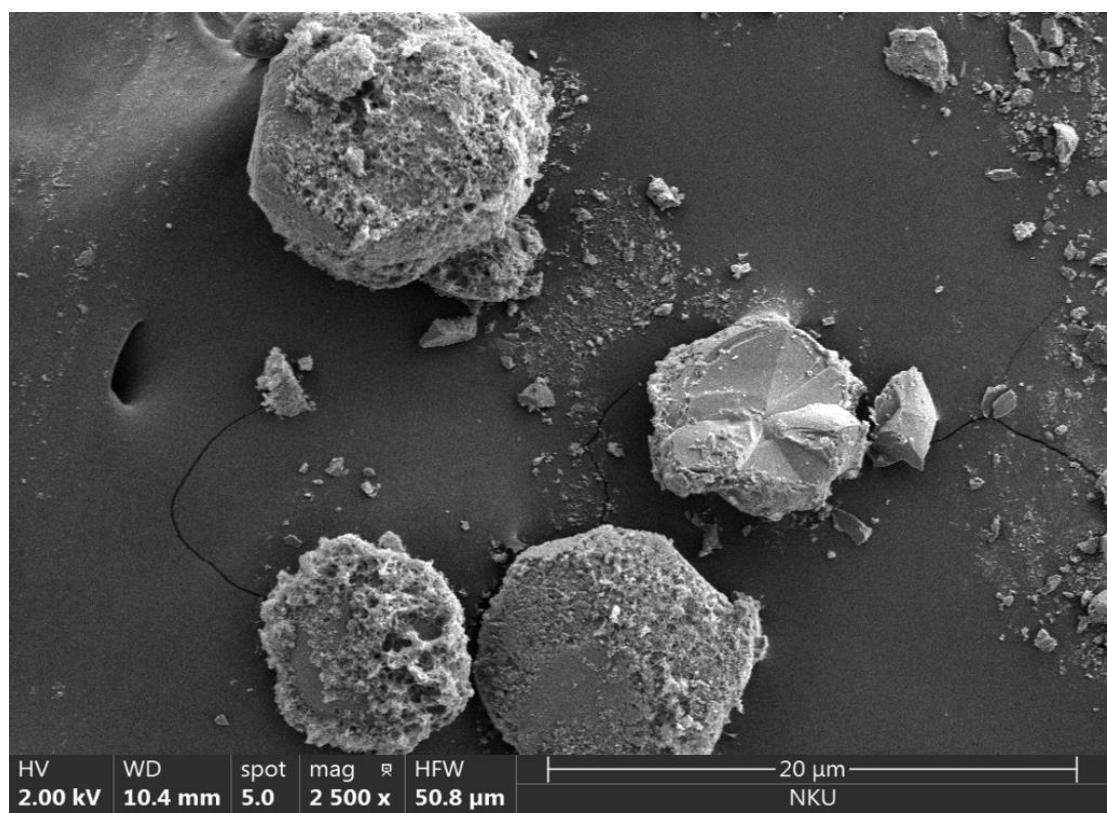
**Fig. S7** SEM images of Cu<sub>0.22</sub>Ni<sub>0.78</sub>-NKU-100 after long-time electrocatalytic test in 0.5 M H<sub>2</sub>SO<sub>4</sub> electrolyte.
