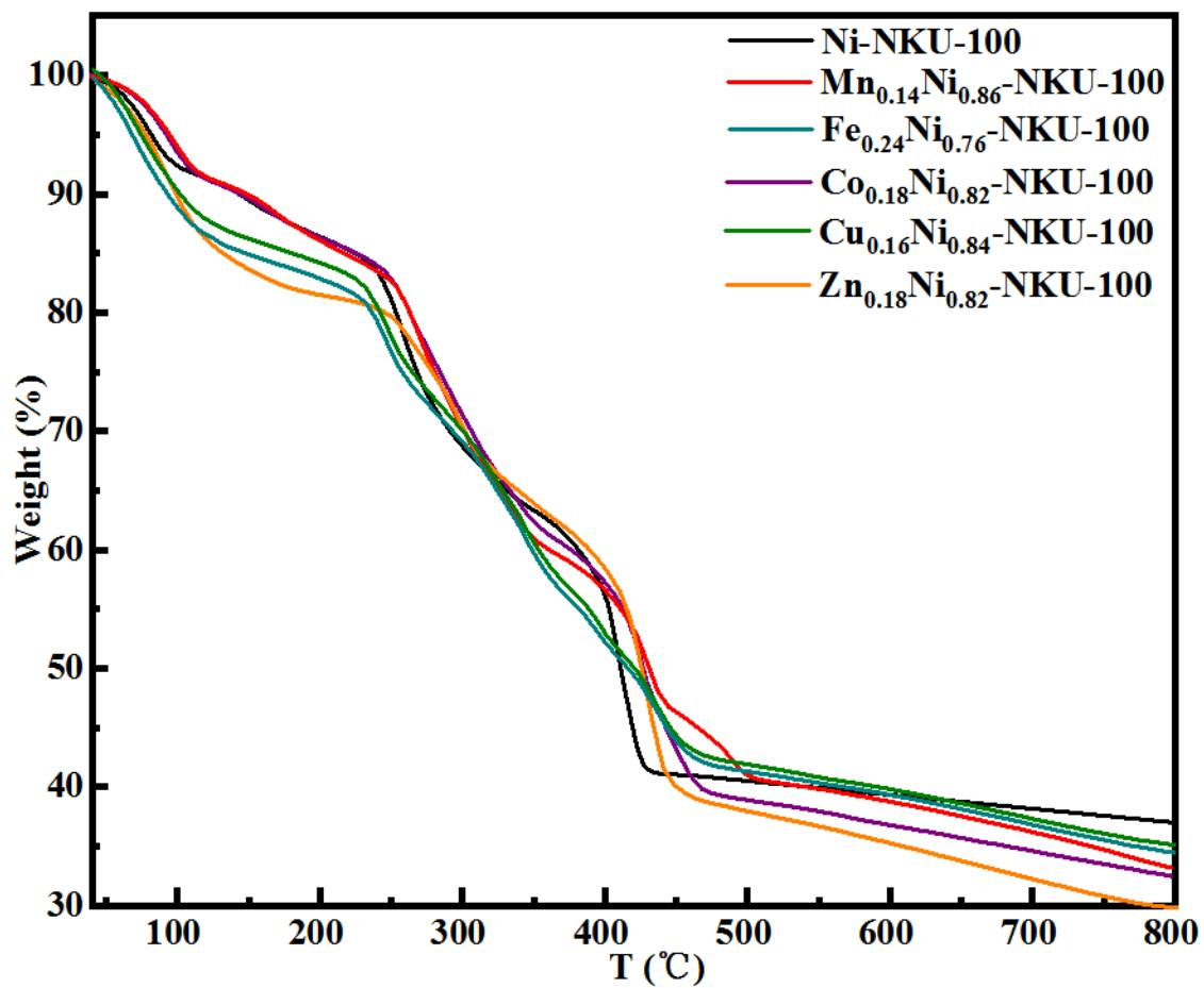
**Fig. S1** Thermogravimetric analysis of Ni-NKU-100 and M<sub>x</sub>Ni<sub>1-x</sub>-NKU-100 (M = Mn, Fe, Co, Cu, Zn).
