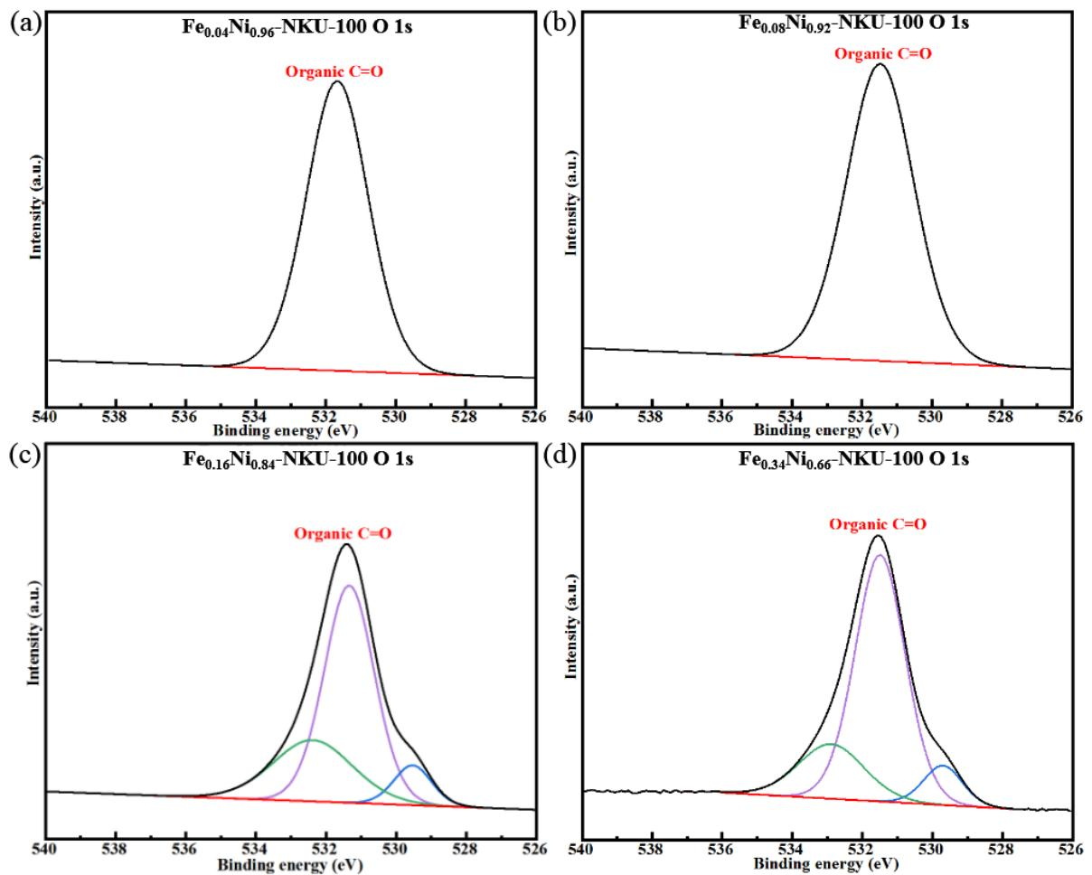
**Fig. S20** High-resolution XPS of O 1s for (a)  $\text{Fe}_{0.04}\text{Ni}_{0.96}$ -NKU-100, (b)  $\text{Fe}_{0.08}\text{Ni}_{0.92}$ -NKU-100, (c)  $\text{Fe}_{0.16}\text{Ni}_{0.84}$ -NKU-100 and (d)  $\text{Fe}_{0.34}\text{Ni}_{0.66}$ -NKU-100.
