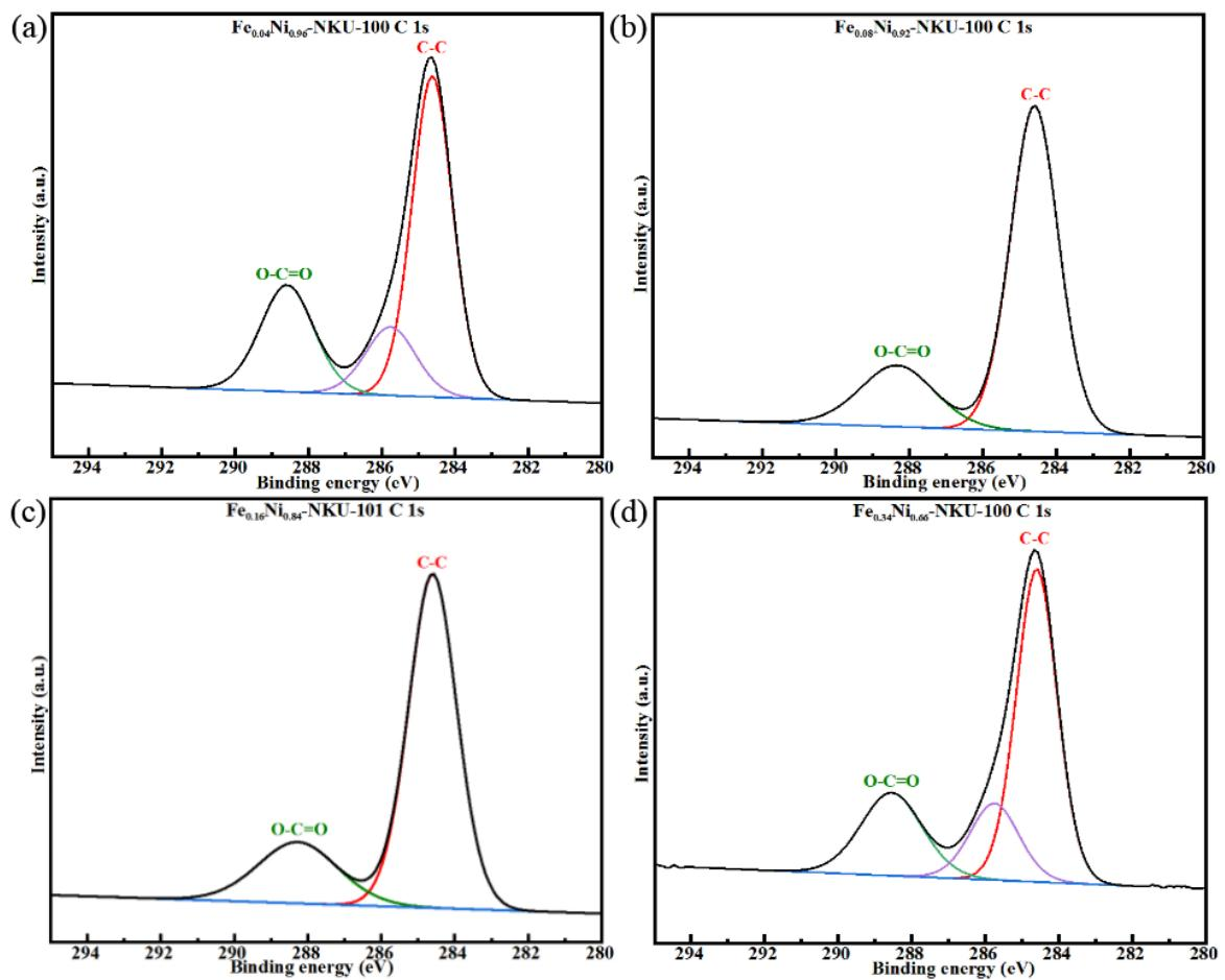
**Fig. S19** High-resolution XPS of C 1s for (a) Fe<sub>0.04</sub>Ni<sub>0.96</sub>-NKU-100, (b) Fe<sub>0.08</sub>Ni<sub>0.92</sub>-NKU-100, (c) Fe<sub>0.16</sub>Ni<sub>0.84</sub>-NKU-100 and (d) Fe<sub>0.34</sub>Ni<sub>0.66</sub>-NKU-100.
