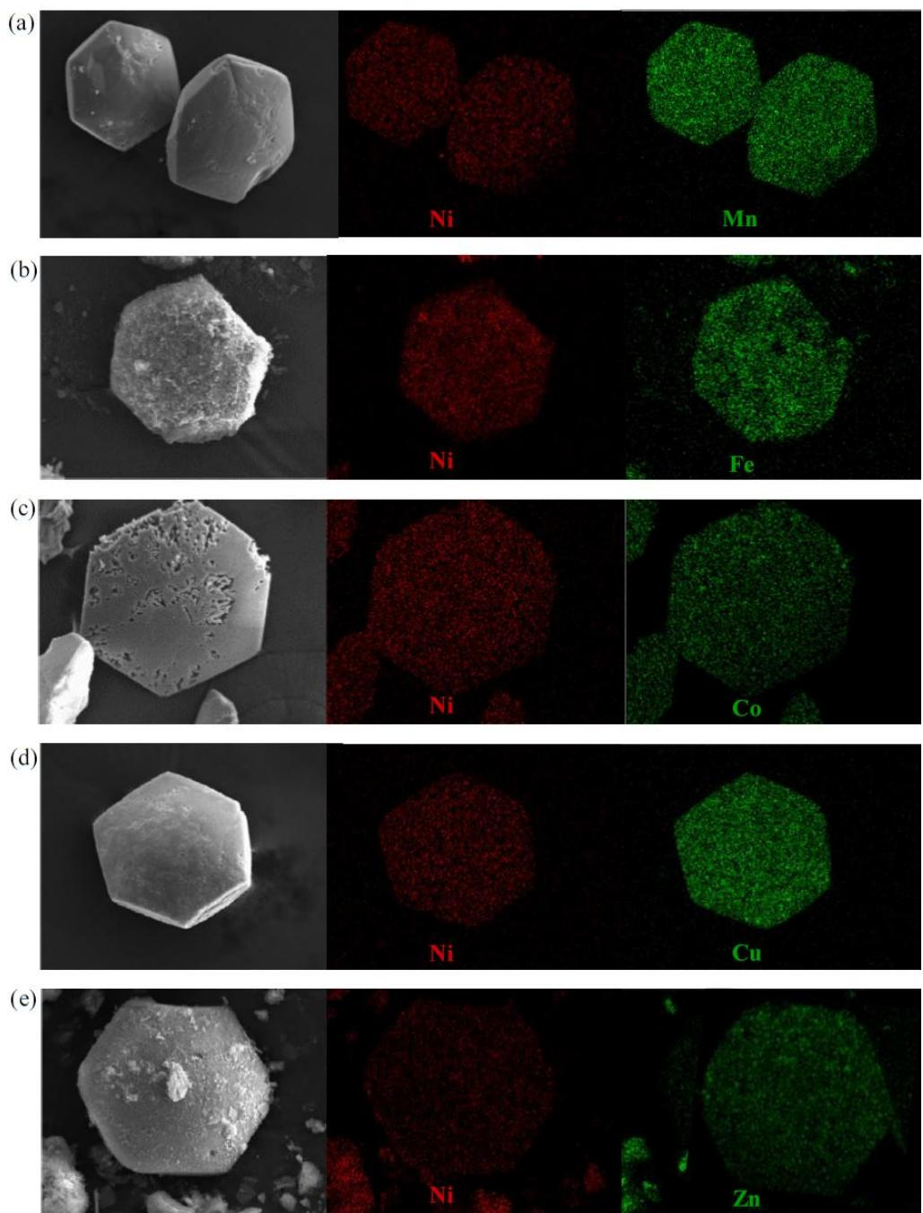
**Fig. S3** SEM images and EDS elemental mappings of  $\text{Mn}_{0.14}\text{Ni}_{0.86}$ -NKU-100 (a),  $\text{Fe}_{0.24}\text{Ni}_{0.76}$ -NKU-100 (b),  $\text{Co}_{0.18}\text{Ni}_{0.82}$ -NKU-100 (c),  $\text{Cu}_{0.16}\text{Ni}_{0.84}$ -NKU-100 (d), and  $\text{Zn}_{0.18}\text{Ni}_{0.82}$ -NKU-100 (e).
