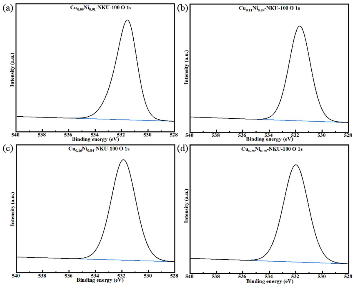
**Fig. S12** High-resolution XPS of O 1s for (a)  $\text{Cu}_{0.09}\text{Ni}_{0.91}\text{-NKU-100}$ , (b)  $\text{Cu}_{0.11}\text{Ni}_{0.89}\text{-NKU-100}$ , (c)  $\text{Cu}_{0.16}\text{Ni}_{0.84}\text{-NKU-100}$  and (d)  $\text{Cu}_{0.25}\text{Ni}_{0.75}\text{-NKU-100}$ .
