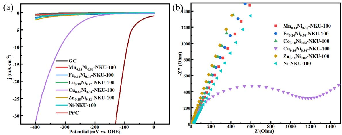
**Fig. S4** (a) LSV curves at a scan rate of  $5 \text{ mV}\cdot\text{s}^{-1}$  and (b) EIS Nyquist plots of  $\text{M}_x\text{Ni}_{1-x}\text{-NKU-100}$  ( $\text{M} = \text{Mn, Fe, Co, Cu, Zn}$ ) in  $0.5 \text{ M H}_2\text{SO}_4$  electrolyte.
