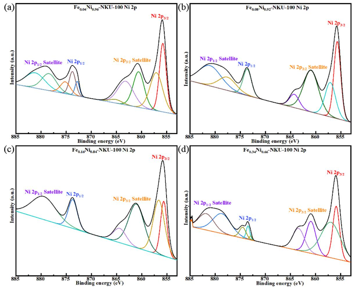
**Fig. S17** High-resolution XPS of Ni 2p for (a)  $\text{Fe}_{0.04}\text{Ni}_{0.96}$ -NKU-100, (b)  $\text{Fe}_{0.08}\text{Ni}_{0.92}$ -NKU-100, (c)  $\text{Fe}_{0.16}\text{Ni}_{0.84}$ -NKU-100 and (d)  $\text{Fe}_{0.34}\text{Ni}_{0.66}$ -NKU-100.
