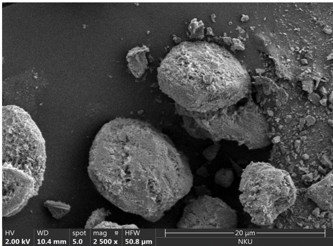
**Fig. S15** SEM images of Fe<sub>0.24</sub>Ni<sub>0.76</sub>-NKU-100 after long-time electrocatalytic test in 1 M NaOH electrolyte.
