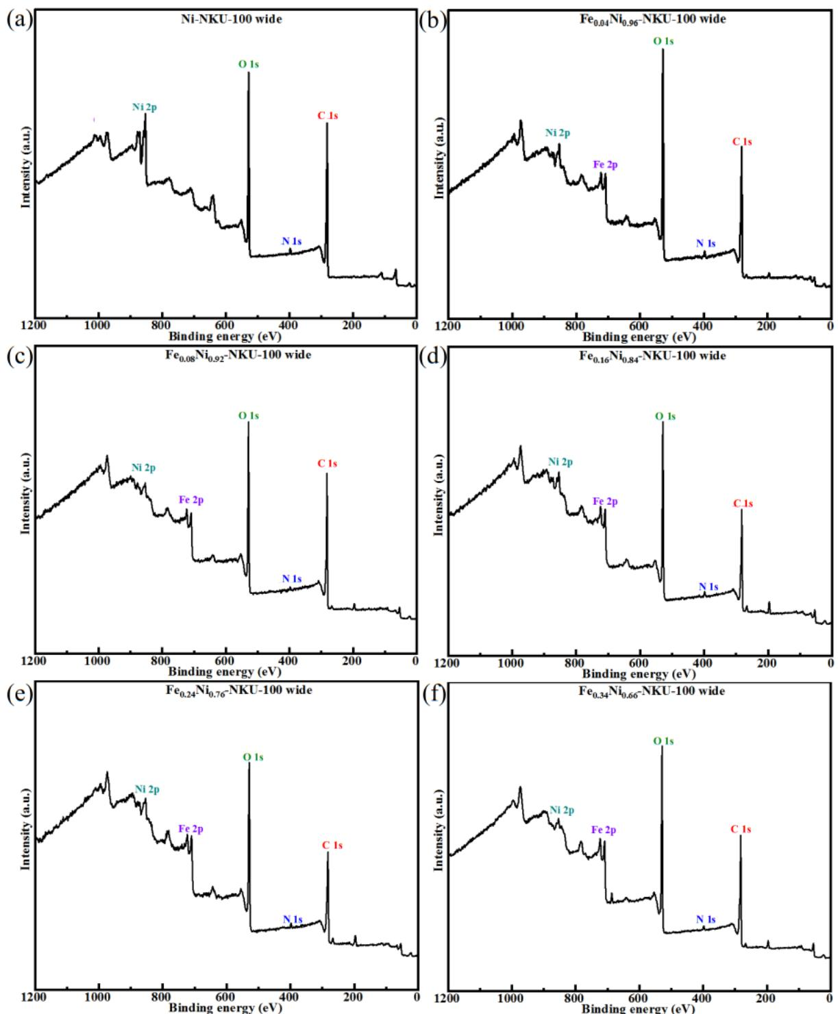
**Fig. S16** XPS wide spectra of (a) Ni-NKU-100, (b)  $\text{Fe}_{0.04}\text{Ni}_{0.96}$ -NKU-100, (c)  $\text{Fe}_{0.08}\text{Ni}_{0.92}$ -NKU-100, (d)  $\text{Fe}_{0.16}\text{Ni}_{0.84}$ -NKU-100, (e)  $\text{Fe}_{0.24}\text{Ni}_{0.76}$ -NKU-100 and (f)  $\text{Fe}_{0.34}\text{Ni}_{0.66}$ -NKU-100.
