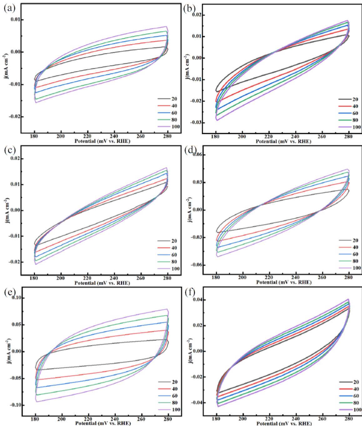
**Fig. S6** CV curves of (a) Ni-NKU-100, (b)  $\text{Cu}_{0.09}\text{Ni}_{0.91}\text{-NKU-100}$ , (c)  $\text{Cu}_{0.11}\text{Ni}_{0.89}\text{-NKU-100}$ , (d)  $\text{Cu}_{0.16}\text{Ni}_{0.84}\text{-NKU-100}$ , (e)  $\text{Cu}_{0.22}\text{Ni}_{0.78}\text{-NKU-100}$  and (f)  $\text{Cu}_{0.25}\text{Ni}_{0.75}\text{-NKU-100}$  at the scan rate range from 20 to 100  $\text{mV s}^{-1}$  in 0.5 M  $\text{H}_2\text{SO}_4$  electrolyte.
