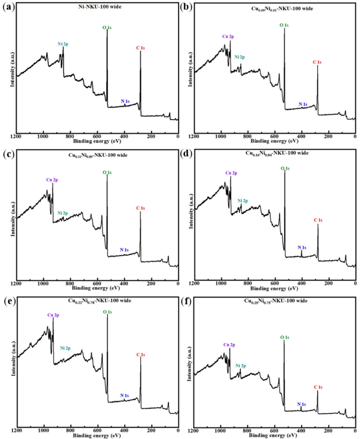
**Fig. S8** XPS wide spectra of (a) Ni-NKU-100, (b) Cu<sub>0.09</sub>Ni<sub>0.91</sub>-NKU-100, (c) Cu<sub>0.11</sub>Ni<sub>0.89</sub>-NKU-100, (d) Cu<sub>0.16</sub>Ni<sub>0.84</sub>-NKU-100, (e) Cu<sub>0.22</sub>Ni<sub>0.78</sub>-NKU-100 and (f) Cu<sub>0.25</sub>Ni<sub>0.75</sub>-NKU-100.
