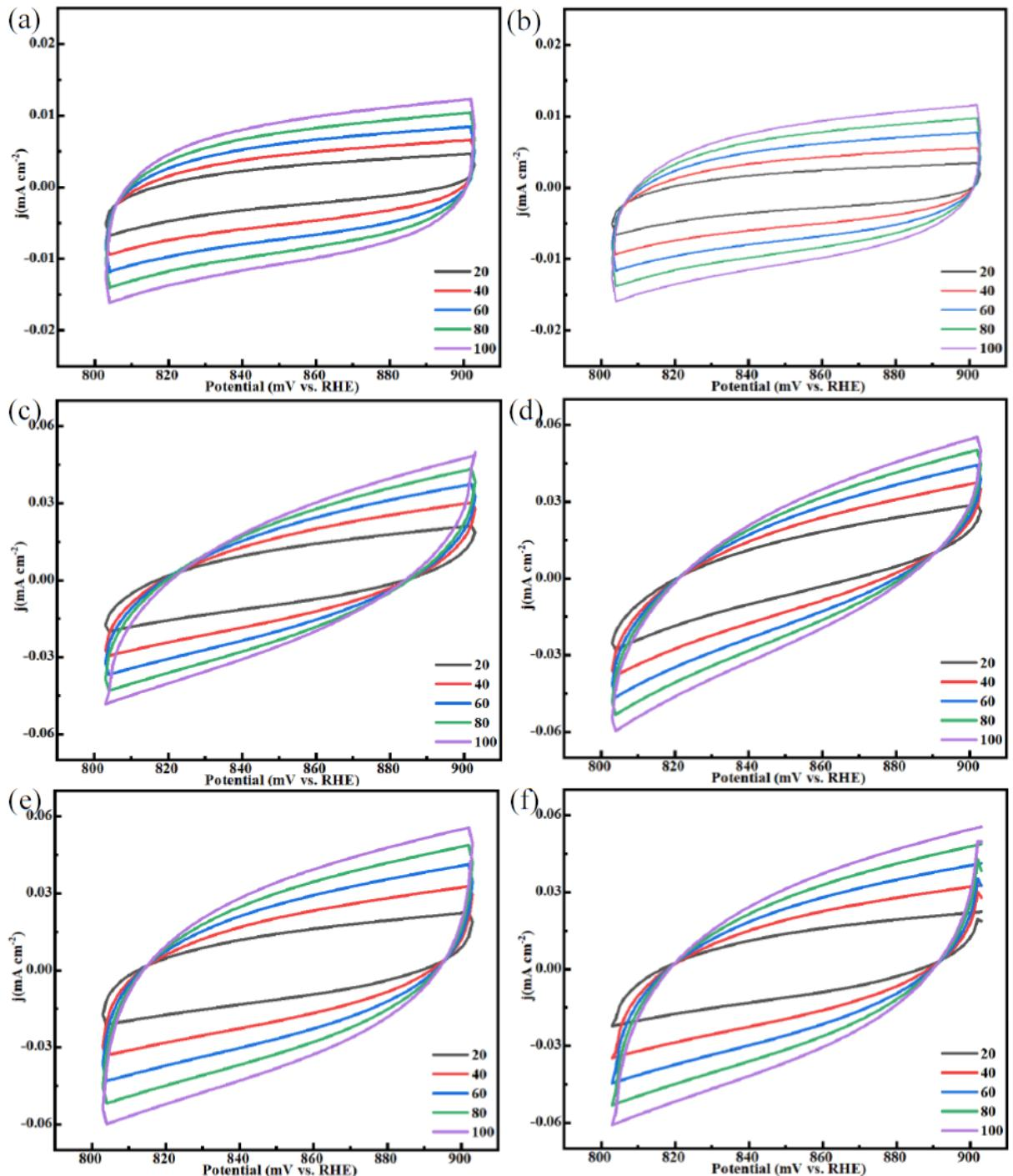
**Fig. S14** CV curves of (a) Ni-NKU-100, (b)  $\text{Fe}_{0.04}\text{Ni}_{0.96}$ -NKU-100, (c)  $\text{Fe}_{0.08}\text{Ni}_{0.92}$ -NKU-100, (d)  $\text{Fe}_{0.16}\text{Ni}_{0.84}$ -NKU-100, (e)  $\text{Fe}_{0.24}\text{Ni}_{0.76}$ -NKU-100 and (f)  $\text{Fe}_{0.34}\text{Ni}_{0.66}$ -NKU-100 at the scan rate range from 20 to 100  $\text{mV s}^{-1}$  in 1 M NaOH electrolyte.
