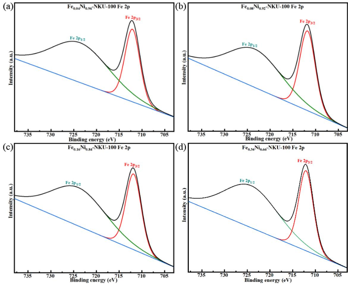
**Fig. S18** High-resolution XPS of Fe 2p for (a)  $\text{Fe}_{0.04}\text{Ni}_{0.96}$ -NKU-100, (b)  $\text{Fe}_{0.08}\text{Ni}_{0.92}$ -NKU-100, (c)  $\text{Fe}_{0.16}\text{Ni}_{0.84}$ -NKU-100 and (d)  $\text{Fe}_{0.34}\text{Ni}_{0.66}$ -NKU-100.
