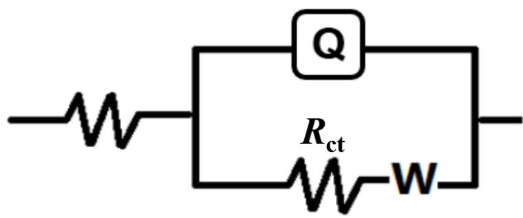
**Fig. S5** The equivalent circuit for fitting electrochemical impedance.
