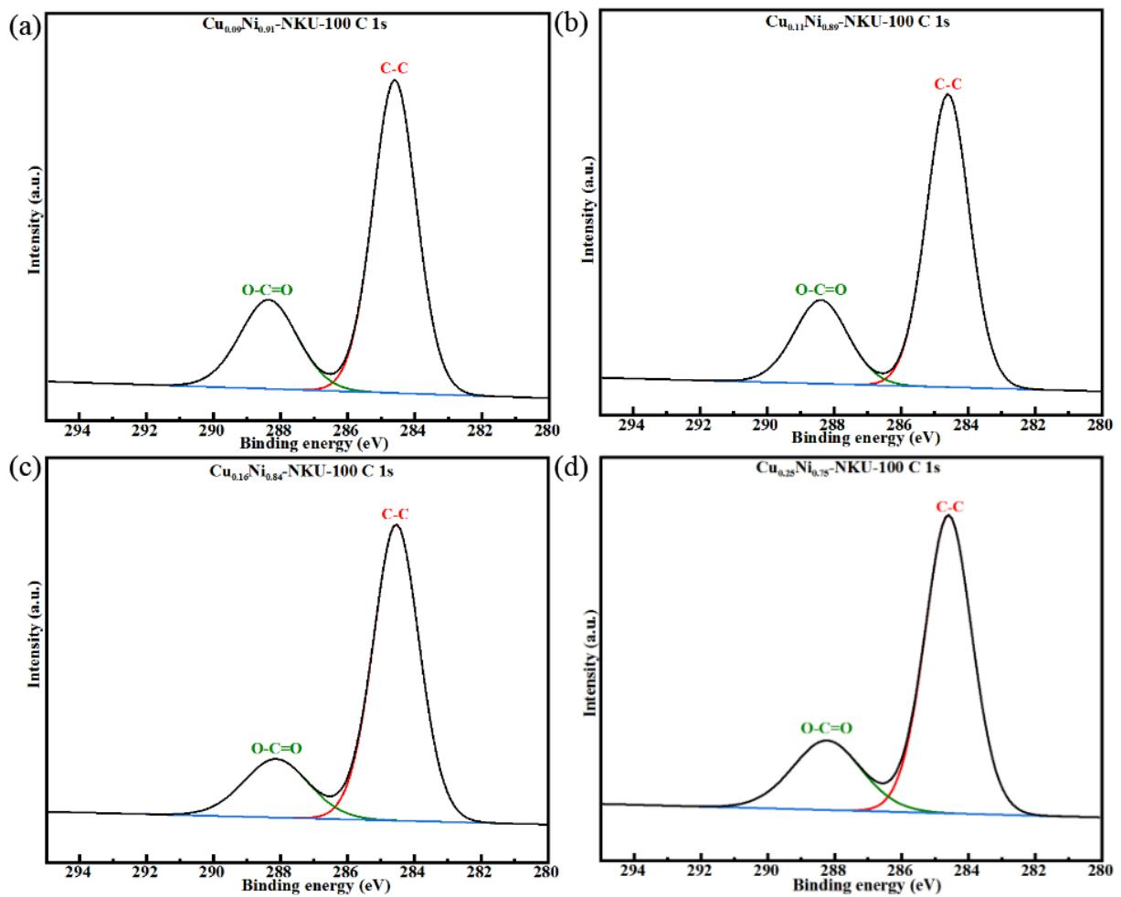
**Fig. S11** High-resolution XPS of C 1s for (a)  $\text{Cu}_{0.09}\text{Ni}_{0.91}$ -NKU-100, (b)  $\text{Cu}_{0.11}\text{Ni}_{0.89}$ -NKU-100, (c)  $\text{Cu}_{0.16}\text{Ni}_{0.84}$ -NKU-100 and (d)  $\text{Cu}_{0.25}\text{Ni}_{0.75}$ -NKU-100.
