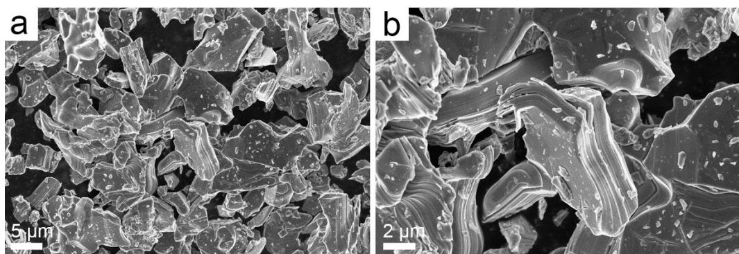
**Fig. S1** Representative SEM images of bulk  $\text{Ti}_3\text{AlC}_2$  at different magnifications.
