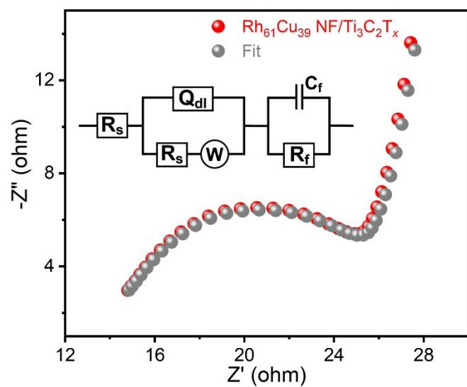
**Fig. S14** Nyquist plots of EIS and fitting curve of the Rh<sub>61</sub>Cu<sub>39</sub> NF/Ti<sub>3</sub>C<sub>2</sub>T<sub>x</sub> electrode.
