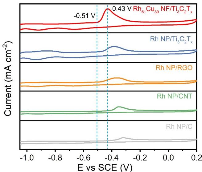
**Fig. S12** CO stripping voltammograms for the Rh<sub>61</sub>Cu<sub>39</sub> NF/Ti<sub>3</sub>C<sub>2</sub>T<sub>x</sub>, Rh NP/Ti<sub>3</sub>C<sub>2</sub>T<sub>x</sub>, Rh NP/RGO,
