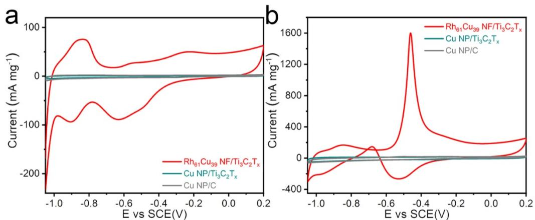
**Fig. S8** CV curves of Rh<sub>61</sub>Cu<sub>39</sub> NF/Ti<sub>3</sub>C<sub>2</sub>T<sub>x</sub>, Cu NP/Ti<sub>3</sub>C<sub>2</sub>T<sub>x</sub> and Cu NP/C in (a) 1 mol L<sup>-1</sup> KOH and (b) 1 mol L<sup>-1</sup> KOH with 1 mol L<sup>-1</sup> CH<sub>3</sub>OH solution at 50 mV s<sup>-1</sup>.
