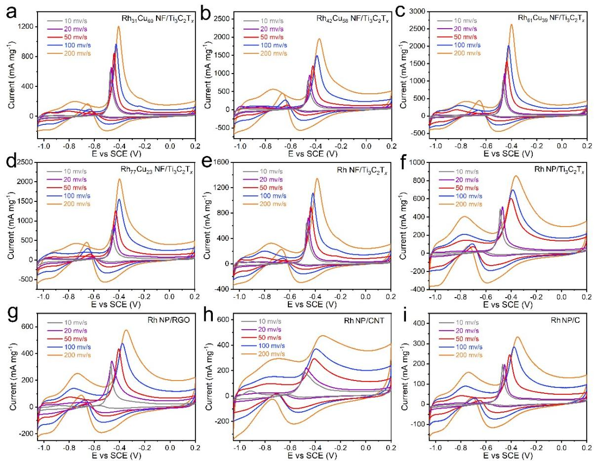
**Fig. S11** The corresponding mass activities curves of (a-e) RhCu NF/Ti<sub>3</sub>C<sub>2</sub>T<sub>x</sub> catalysts with different Rh/Cu ratios and (f-i) Rh NP/Ti<sub>3</sub>C<sub>2</sub>T<sub>x</sub>, Rh NP/RGO, Rh NP/CNT and Rh NP/C.
