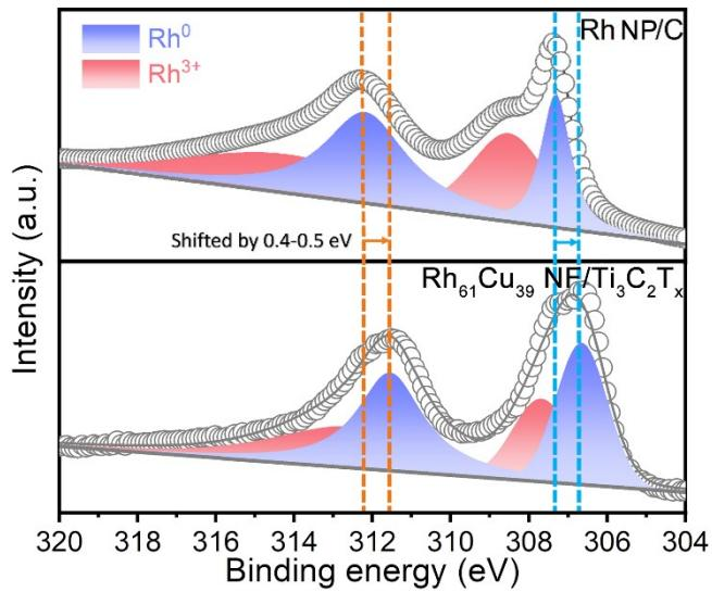
**Fig. S7** Comparison of the binding energies for Rh 3d spectra of the Rh<sub>61</sub>Cu<sub>39</sub> NF/Ti<sub>3</sub>C<sub>2</sub>T<sub>x</sub> and Rh NP/C samples.
