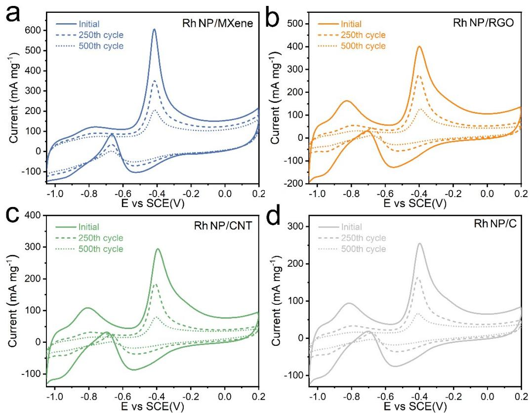
**Fig. S13** The CV curves of (a) Rh NP/Ti<sub>3</sub>C<sub>2</sub>T<sub>x</sub>, (b) Rh NP/RGO, (c) Rh NP/CNT and (d) Rh NP/C before and after 500 cycles.
