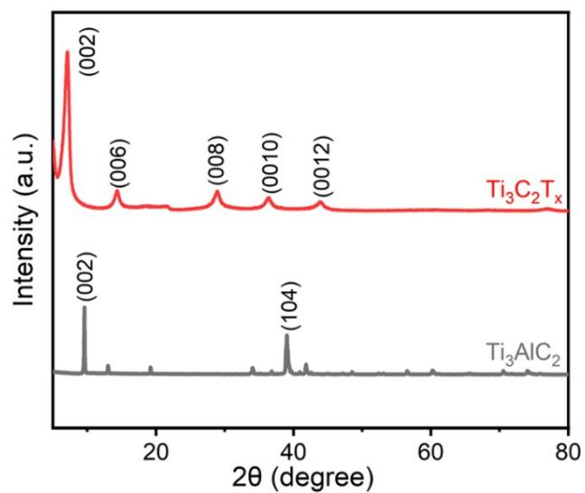
**Fig. S4** XRD patterns of the bulk  $\text{Ti}_3\text{AlC}_2$  and  $\text{Ti}_3\text{C}_2\text{T}_x$  nanosheets.
