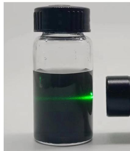
**Fig. S3** The Tyndall phenomenon of the as-obtained  $\text{Ti}_3\text{C}_2\text{T}_x$  MXene solution
