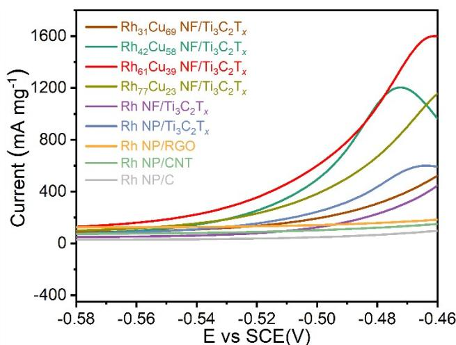
**Fig. S10** LSV curves of the RhCu NF/Ti<sub>3</sub>C<sub>2</sub>T<sub>x</sub> electrocatalysts with different Rh/Cu ratios, Rh NP/Ti<sub>3</sub>C<sub>2</sub>T<sub>x</sub>, Rh NP/RGO, Rh NP/CNT and Rh NP/C in a 1 mol L<sup>-1</sup> KOH with 1 mol L<sup>-1</sup> CH<sub>3</sub>OH
