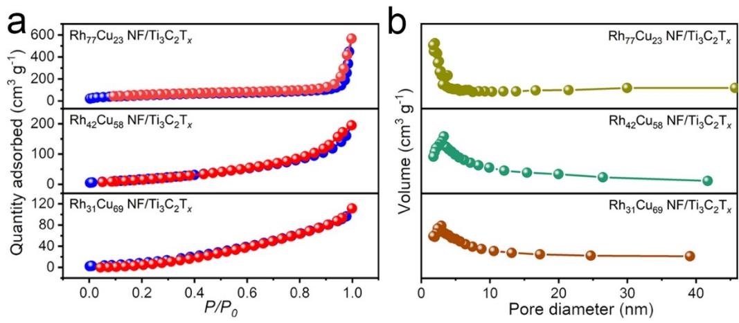
**Fig. S5** (a) Nitrogen adsorption-desorption isotherms and (b) pore size distributions of the  $\text{Rh}_{77}\text{Cu}_{23} \text{NF}/\text{Ti}_3\text{C}_2\text{T}_x$ ,  $\text{Rh}_{42}\text{Cu}_{58} \text{NF}/\text{Ti}_3\text{C}_2\text{T}_x$  and  $\text{Rh}_{31}\text{Cu}_{69} \text{NF}/\text{Ti}_3\text{C}_2\text{T}_x$  samples.
