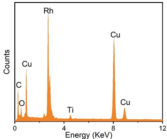
**Fig. S6** EDX spectrum of the  $\text{RhCu NF}/\text{Ti}_3\text{C}_2\text{T}_x$  catalyst.
