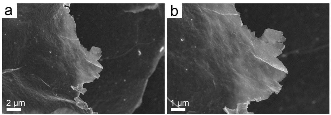
**Fig. S2** Representative SEM images of 2D exfoliated  $\text{Ti}_3\text{C}_2\text{T}_x$  at different magnifications.
