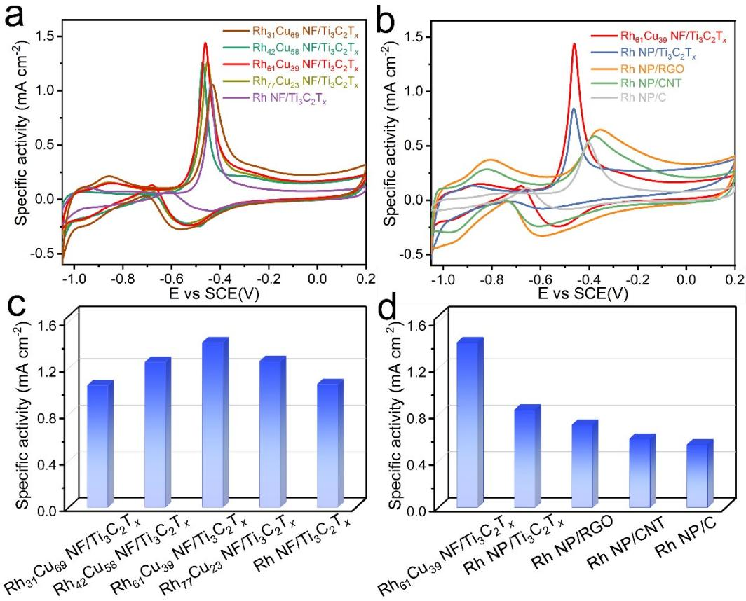
**Fig. S9** The ECSA-normalized CV curves of the (a) RhCu NF/Ti<sub>3</sub>C<sub>2</sub>T<sub>x</sub> catalysts with different Rh/Cu ratios and (b) Rh<sub>61</sub>Cu<sub>39</sub> NF/Ti<sub>3</sub>C<sub>2</sub>T<sub>x</sub>, Rh NP/Ti<sub>3</sub>C<sub>2</sub>T<sub>x</sub>, Rh NP/RGO, Rh NP/CNT and Rh NP/C in 1 mol L<sup>-1</sup> KOH with 1 mol L<sup>-1</sup> CH<sub>3</sub>OH solution. (c-d) Specific activities of various catalysts.
