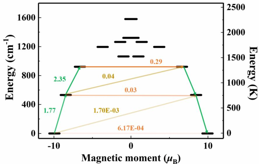
**Figure S21** *Ab initio* calculated possible magnetic relaxation path diagram for **4Dy**. The horizontal orange arrows represent the QTM/TA-QTM processes, while the non-horizontal ones show the spin-phonon transition paths. The numbers next to the arrows are averaged transition magnetic moments ( $(|\mu_x|+|\mu_y|+|\mu_z|)/3$ ) in  $\mu_{\text{B}}$  between the connecting pairs.
