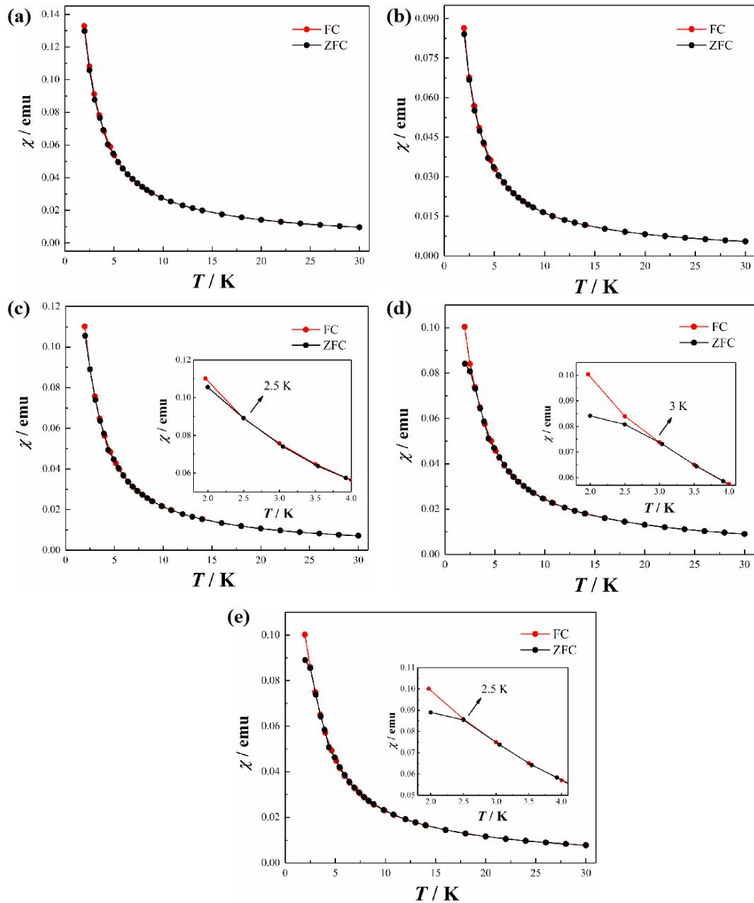
**Figure S12** Field-cooled (FC) and zero-field-cooled (ZFC) magnetic susceptibilities for **1Dy** (a), **2Dy** (b), **3Dy** (c), **4Dy** (d) and **5Dy** (e) under a dc magnetic field of 2000 Oe.
