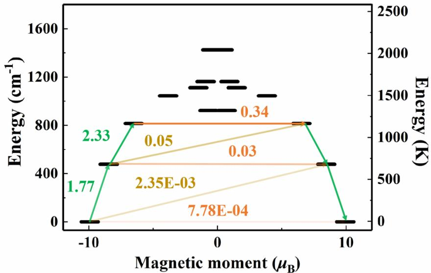
**Figure S23** *Ab initio* calculated possible magnetic relaxation path diagram for **5Dy-2**. The horizontal orange arrows represent the QTM/TA-QTM processes, while the non-horizontal ones show the spin-phonon transition paths. The numbers next to the arrows are averaged transition magnetic moments  $((|\mu_x|+|\mu_y|+|\mu_z|)/3)$  in  $\mu_B$  between the connecting pairs.
