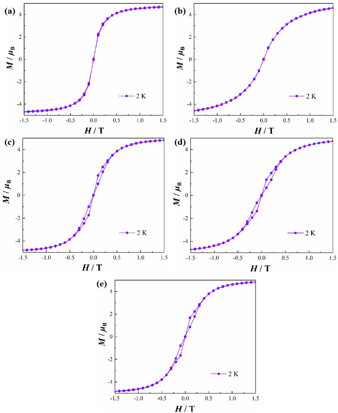
**Figure S13** Magnetic hysteresis loop for **1Dy** (a), **2Dy** (b), **3Dy** (c), **4Dy** (d) and **5Dy** (e) at 2 K with an average scan rate of 30 Oe s<sup>-1</sup>.
