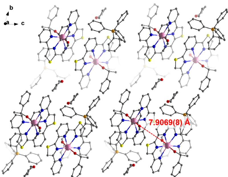
**Figure S4** Packing arrangement of **2Dy**. The red dashed lines represent the nearest intermolecular  $\text{Dy}\cdots\text{Dy}$  separation. For clarity, hydrogen atoms are omitted. Colour codes:  $\text{Dy}$ , pink;  $\text{S}$ , yellow;  $\text{B}$ , orange;  $\text{C}$ , gray;  $\text{O}$ , red;  $\text{N}$ , blue.
