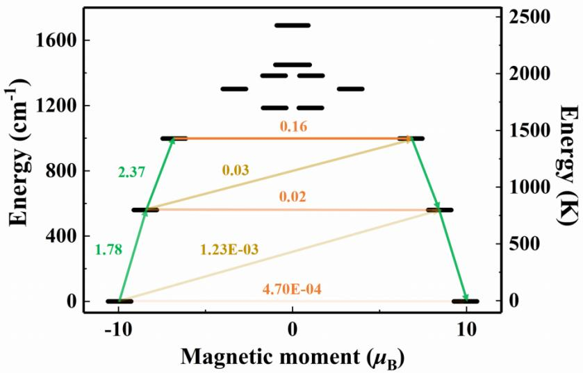
**Figure S22** *Ab initio* calculated possible magnetic relaxation path diagram for **5Dy-1**. The horizontal orange arrows represent the QTM/TA-QTM processes, while the non-horizontal ones show the spin-phonon transition paths. The numbers next to the arrows are averaged transition magnetic moments  $((|\mu_x|+|\mu_y|+|\mu_z|)/3)$  in  $\mu_B$  between the connecting pairs.
