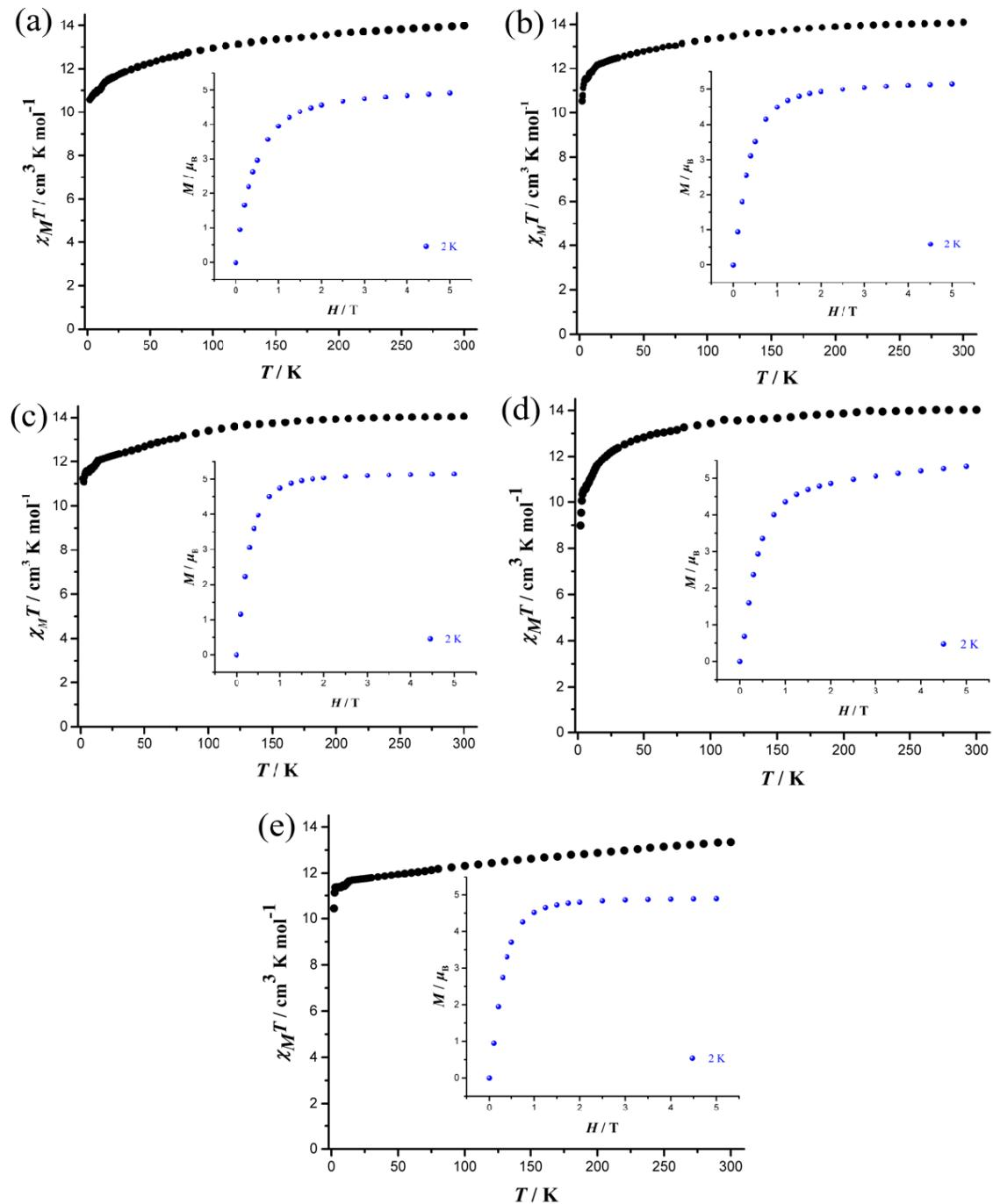
**Figure S8** Temperature dependence of the product  $\chi_M T$  with an applied field of 1 kOe and field dependent magnetization at 2 K up to 5 T (insert) for **1Dy** (a), **2Dy** (b), **3Dy** (c), **4Dy** (d) and **5Dy** (e), respectively.
