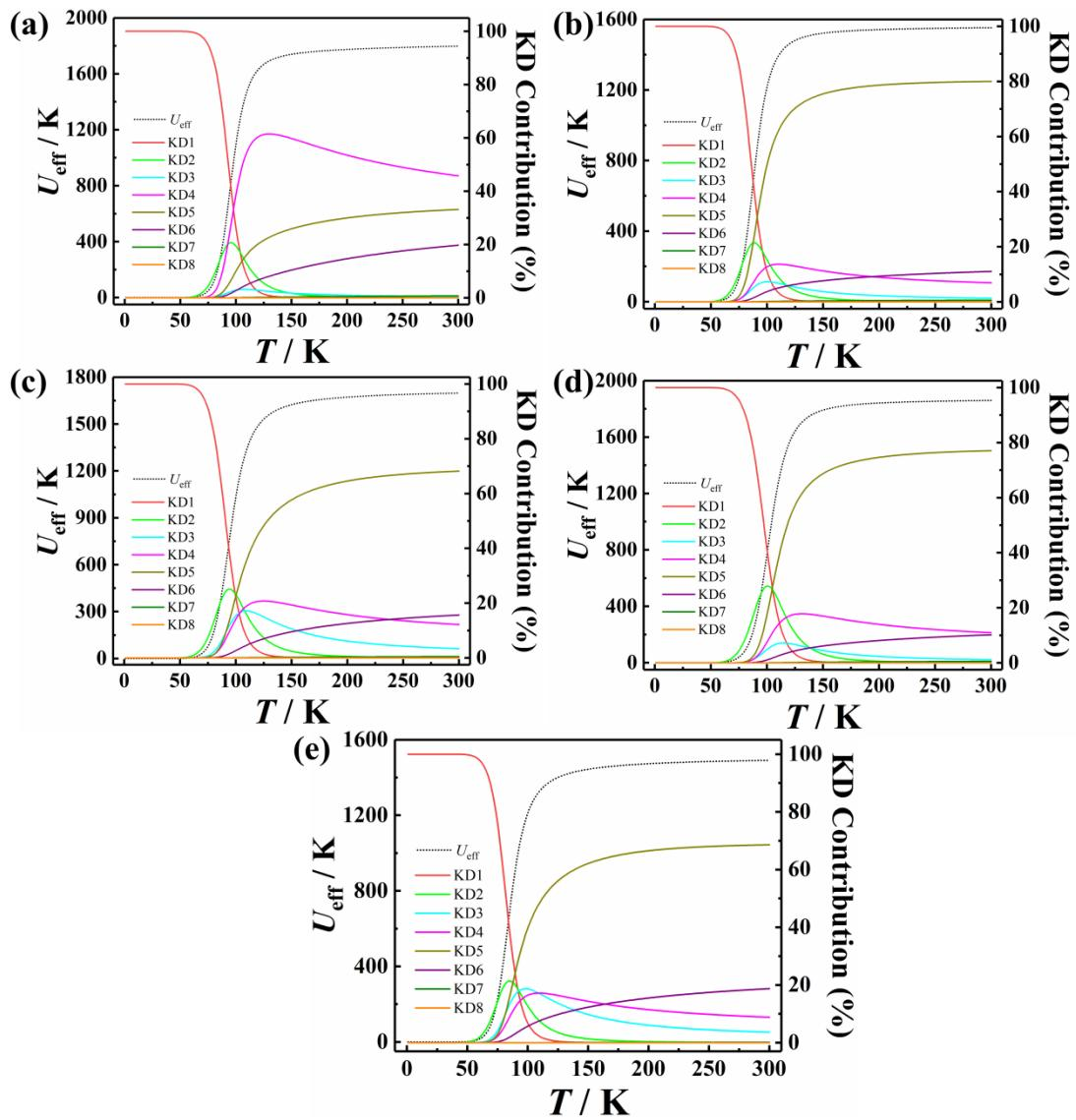
**Figure S24** Predicted  $U_{\text{eff}}$  (black dotted lines) and relaxation contributions from various KDs (coloured solid lines) for **1Dy** (a), **3Dy** (b), **4Dy** (c), **5Dy-1** (d) and **5Dy-2** (e).
