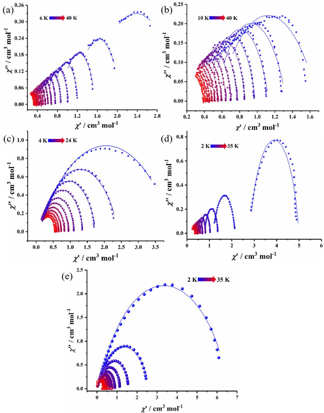
**Figure S11** Cole-Cole plots for **1Dy** (a), **2Dy** (b), **3Dy** (c), **4Dy** (d) and **5Dy** (e) at zero dc field. The solid lines are the best fits obtained with a generalized Debye model.
