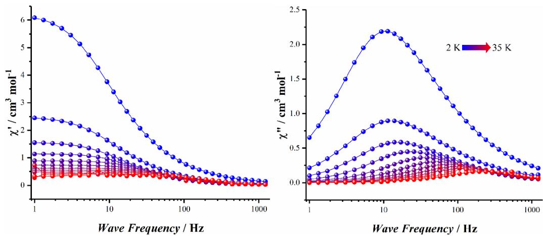
**Figure S10** Frequency dependence of the in-phase  $\chi'$  (left) and out-of-phase  $\chi''$  (right) components of the ac susceptibility for **5Dy** measured under zero dc field. Solid lines represent the fits using the generalized Debye model.
