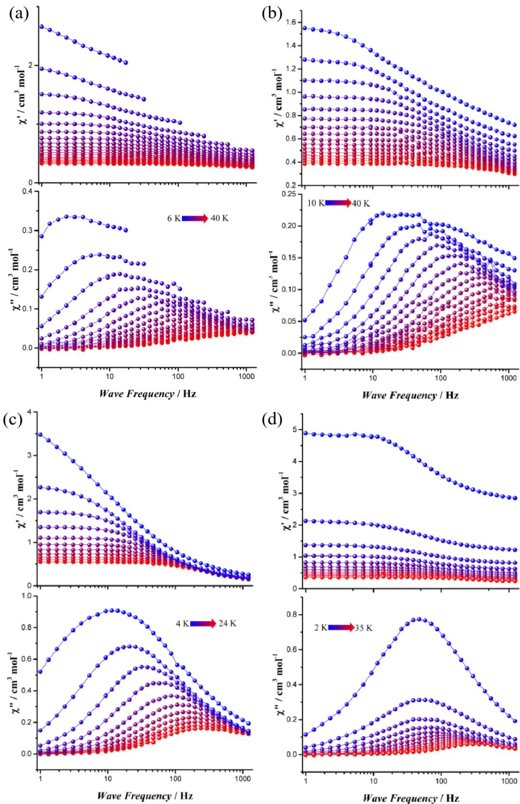
**Figure S9** Frequency dependence of the in-phase  $\chi'$  (top) and out-of-phase  $\chi''$  (bottom) components of the ac susceptibility for **1Dy** (a), **2Dy** (b), **3Dy** (c) and **4Dy** (d) measured under zero dc field. Solid lines represent the fits using the generalized Debye model.
