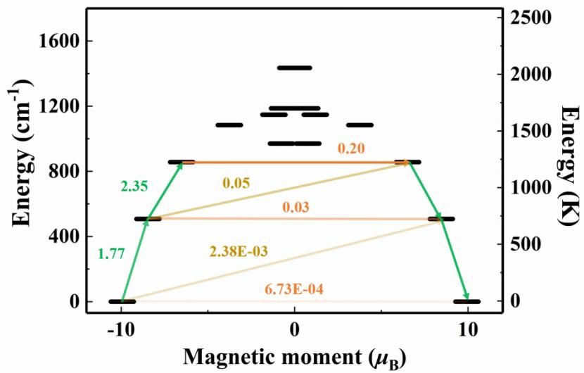
**Figure S20** *Ab initio* calculated possible magnetic relaxation path diagram for **3Dy**. The horizontal orange arrows represent the QTM/TA-QTM processes, while the non-horizontal ones show the spin-phonon transition paths. The numbers next to the arrows are averaged transition magnetic moments ( $(|\mu_x|+|\mu_y|+|\mu_z|)/3$ ) in  $\mu_{\text{B}}$  between the connecting pairs.
